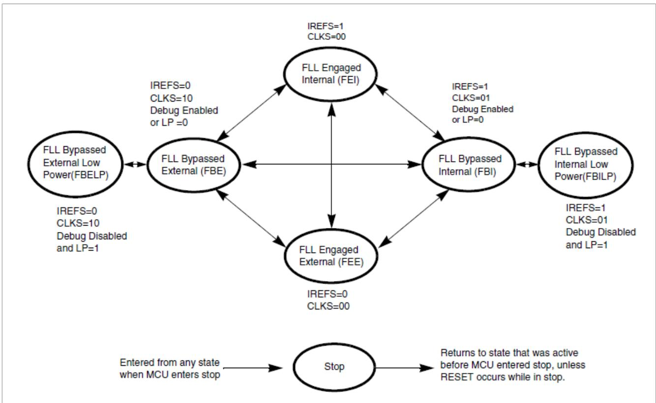
Figure 1. ICS clocking switching modes
