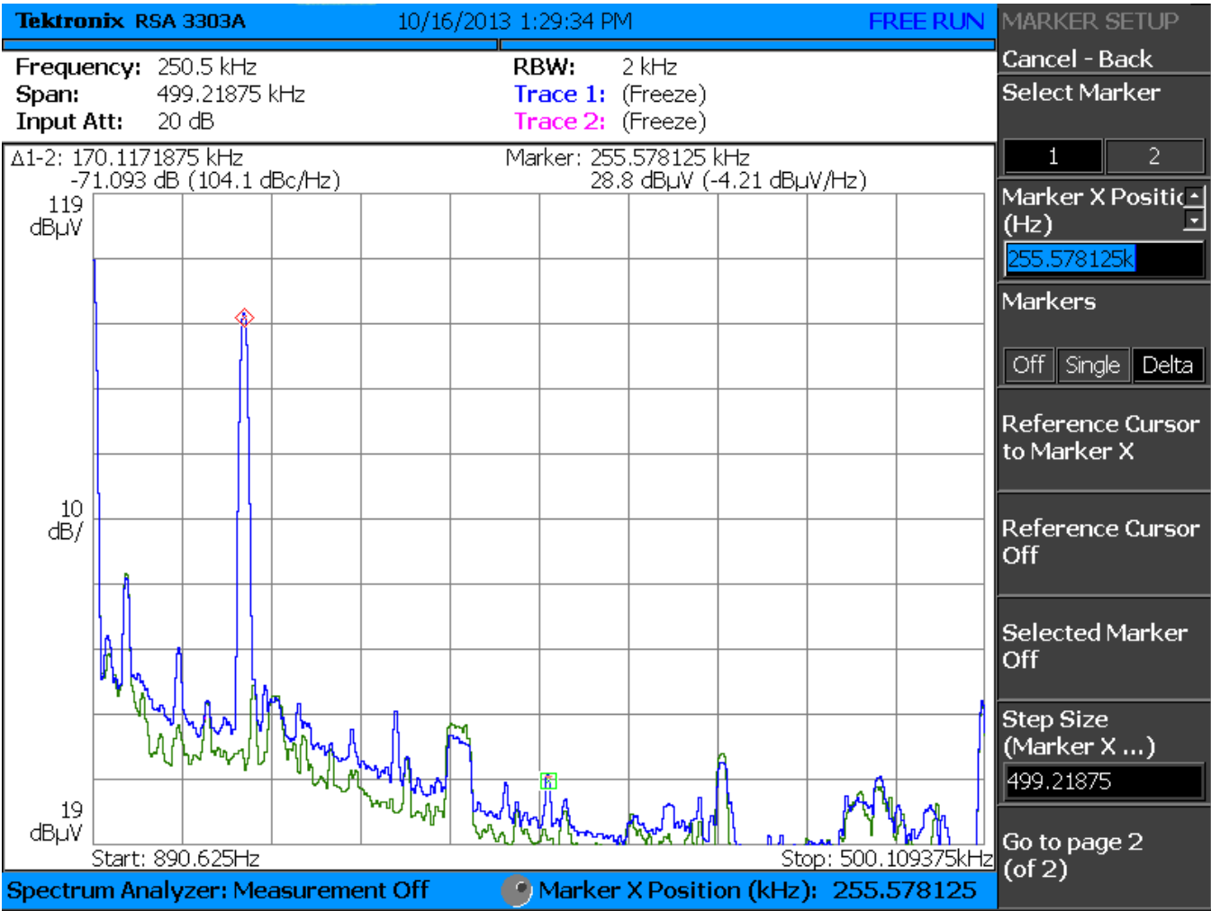
Figure 17. Input signal: 8 mV PP PGA1 31.5 dB, PGA2 32 dB
