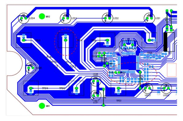
Figure 6 Touch Sense Input PCB layout
