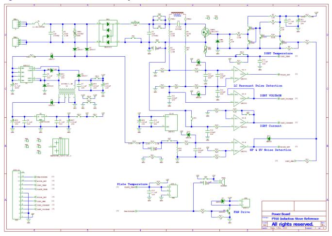
Figure 18 Power board schematic
