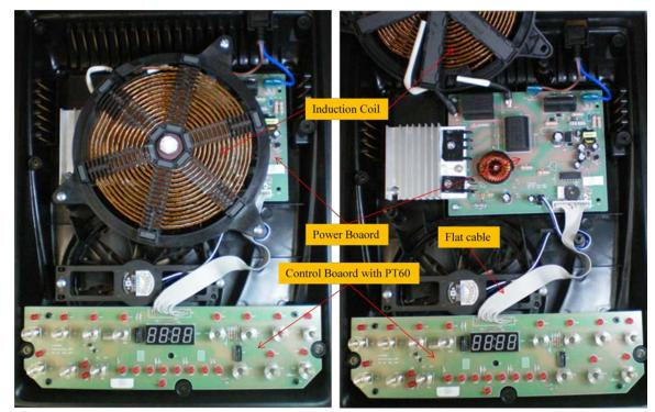
Figure 1 Induction cooker prototype
