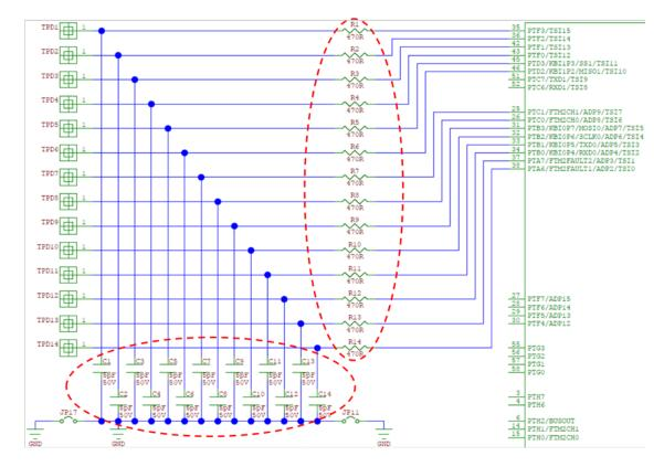
Figure 5 Touch Sense Input circuitry
