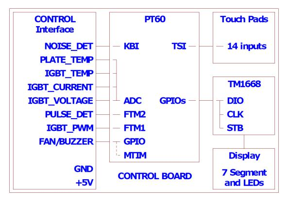
Figure 3 Control board block diagram
