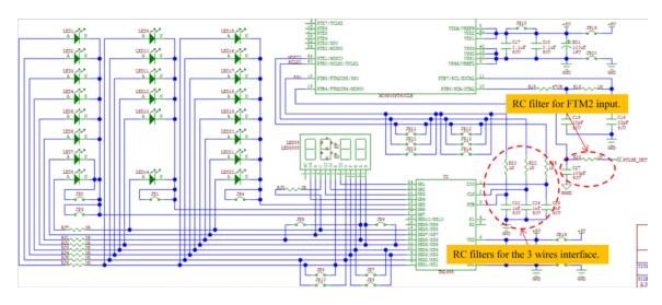
Figure 4 LED driver circuit
