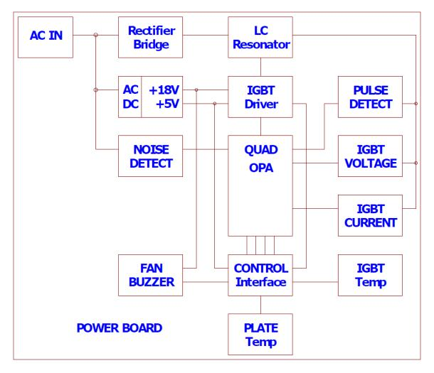
Figure 2 Power board block diagram
