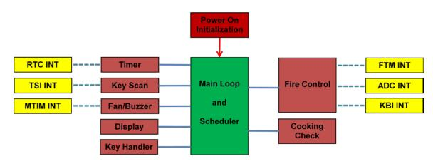
Figure 12 Firmware block diagram
