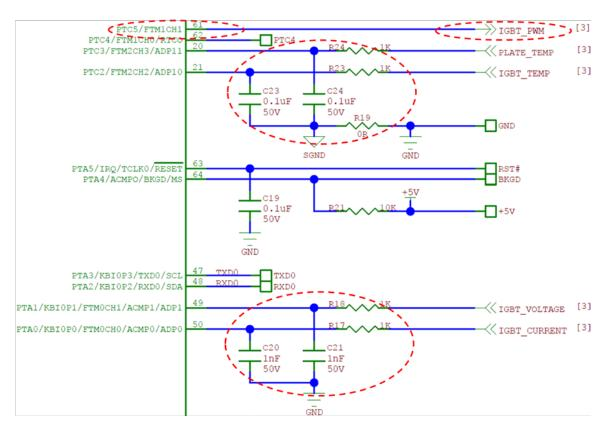
Figure 7 Temperature sensing and voltage/current measurement
