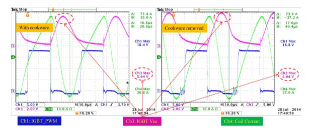
Figure 16 Over driving and cookware removed detection
