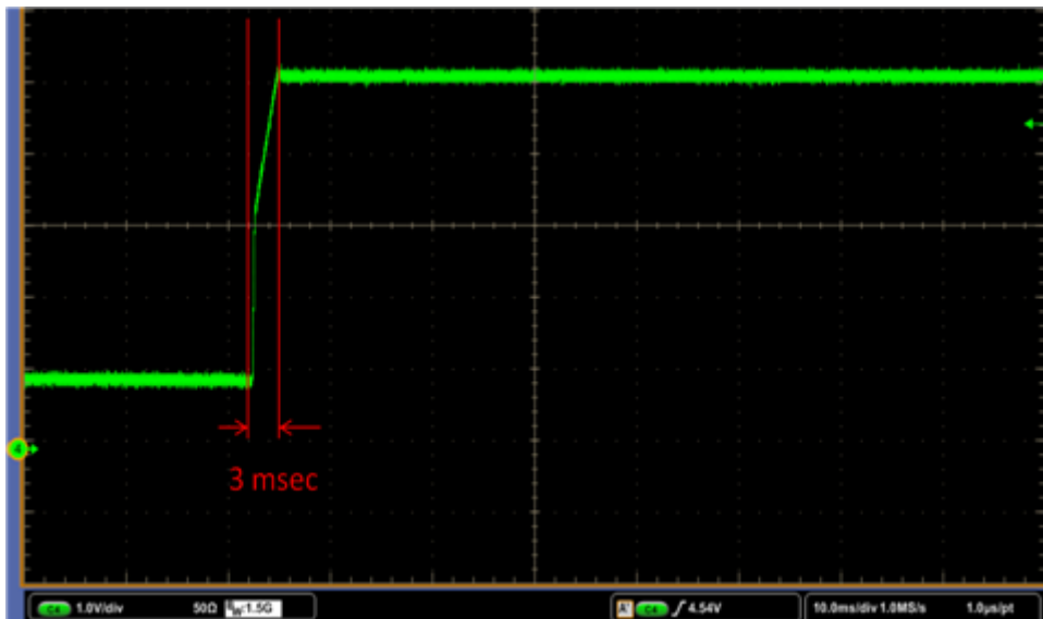
Figure 3. Start-up time profile of fast reference circuit
