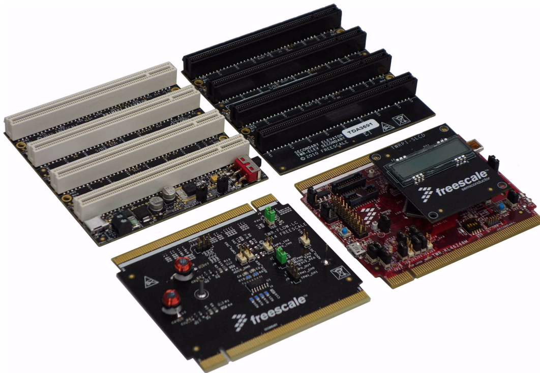
Figure 8. Tower system set used for the LC sensor-based encoder
