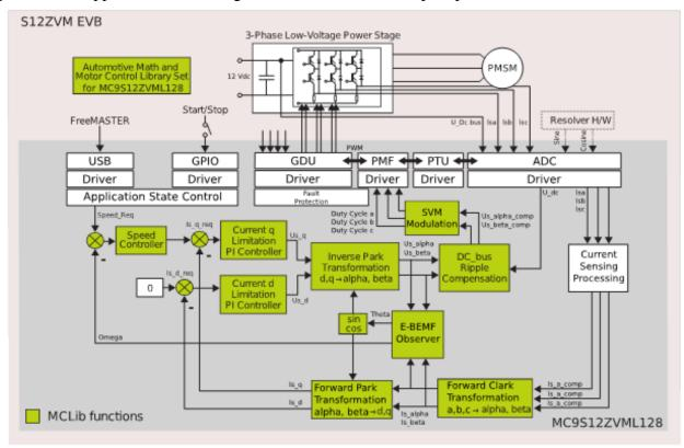
Figure 25. Sensorless FOC implementation
