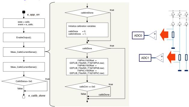
Figure 20. Flow chart of state CALIB
