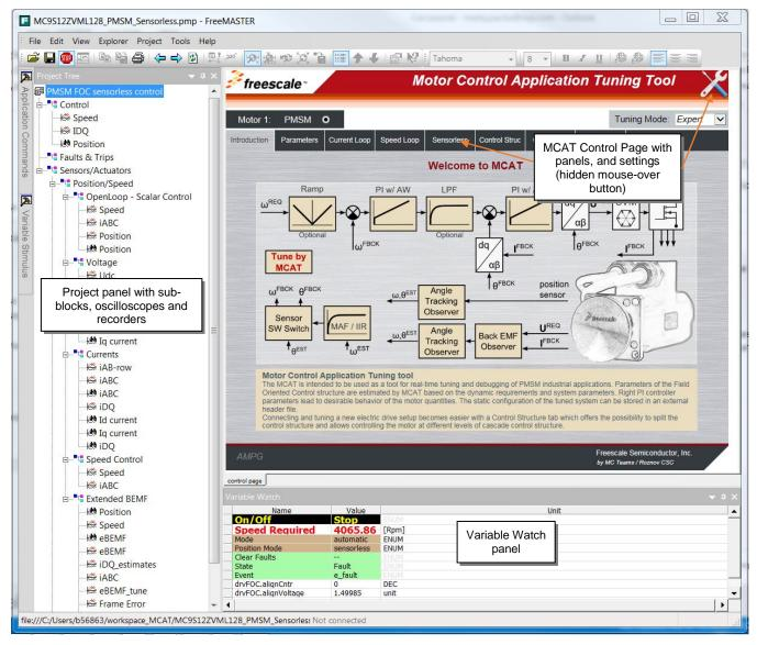
Figure 26. FreeMASTER and Motor Control Application tuning tool
