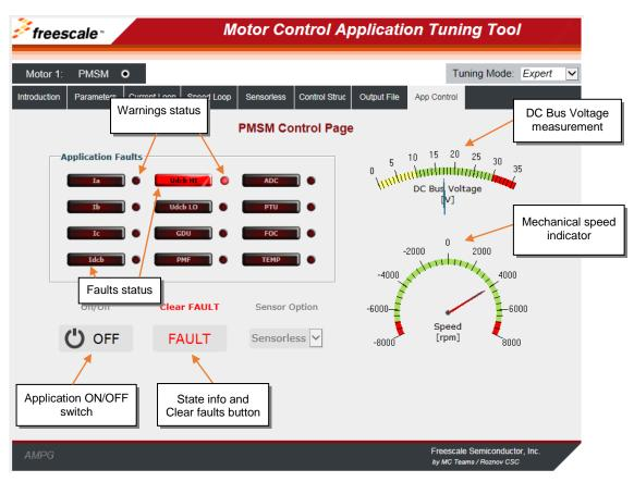
Figure 30. FreeMASTER MCAT control page for controlling the application
