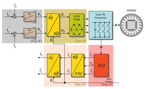
Figure 3. FOC Control Structure
