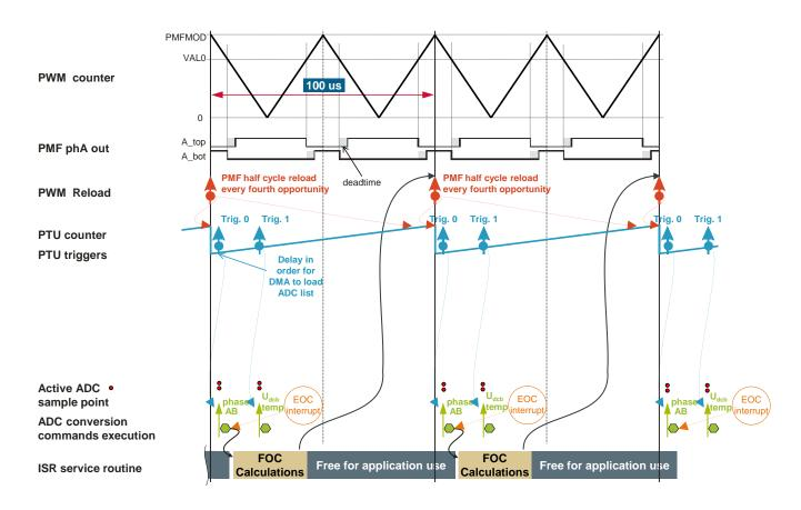
Figure 10. Time Diagram of PWM and ADC Synchronization
