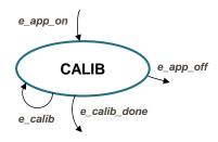
Figure 19. CALIB state with transitions
