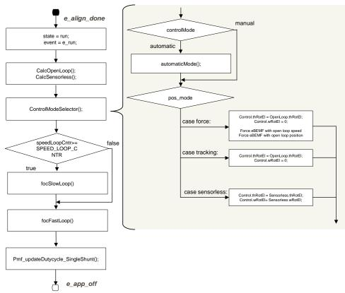
Figure 24. Flow chart of state RUN
