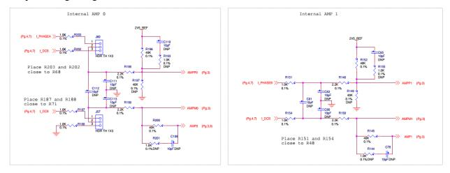
Figure 5. Phase current measurement conditional circuitry
