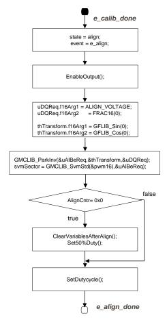
Figure 22. Flow chart of state ALIGN
