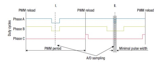
Figure 6. Generated phase duty cycles in different PWM periods
