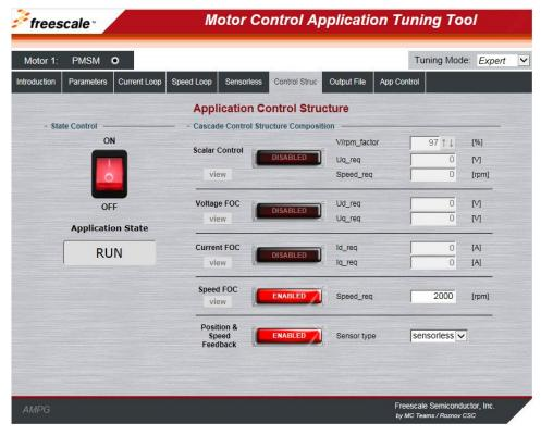
Figure 29. MCAT application control structure page
