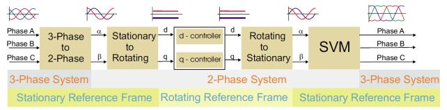
Figure 1. Field oriented control transformations
