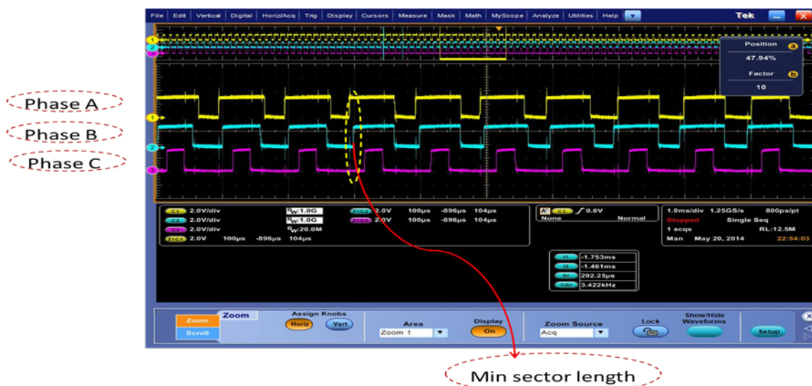
Figure 29. PWM pulses shift when voltage vector crosses V100 sector border
