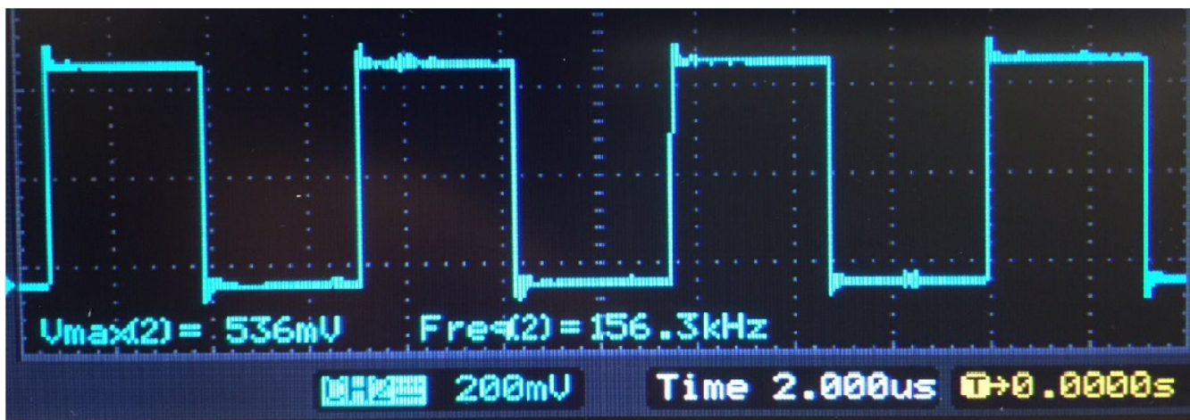
Figure 9. FEE mode clock BUSOUT (BUSOUT/128) output at 156.25 KHz frequency scope shot
