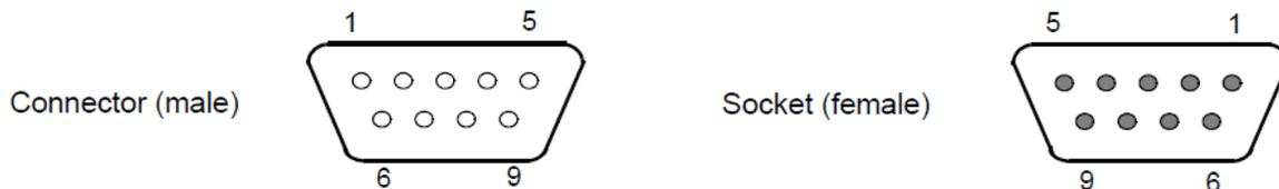
Figure 15. DB-9 connector and socket
