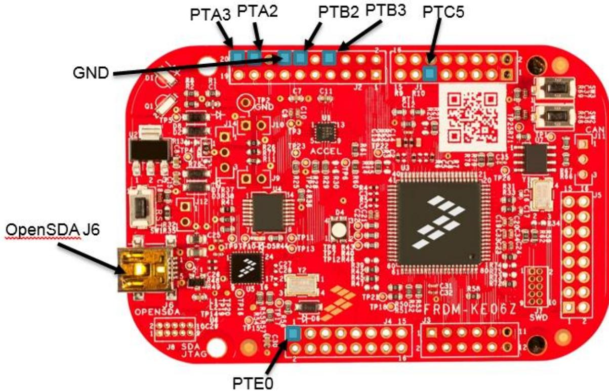
Figure 4. FRDM-KE06Z and Used Pins
