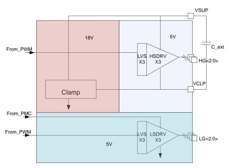
Figure 2. Clamp Circuit Diagram
