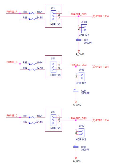
Figure 6. Phase Detector External Circuit on PCB
