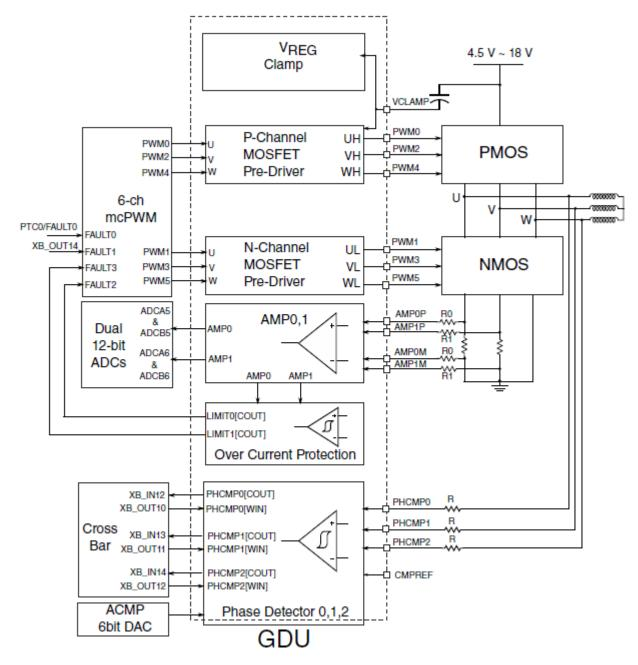
Figure 1. GDU Block Diagram
