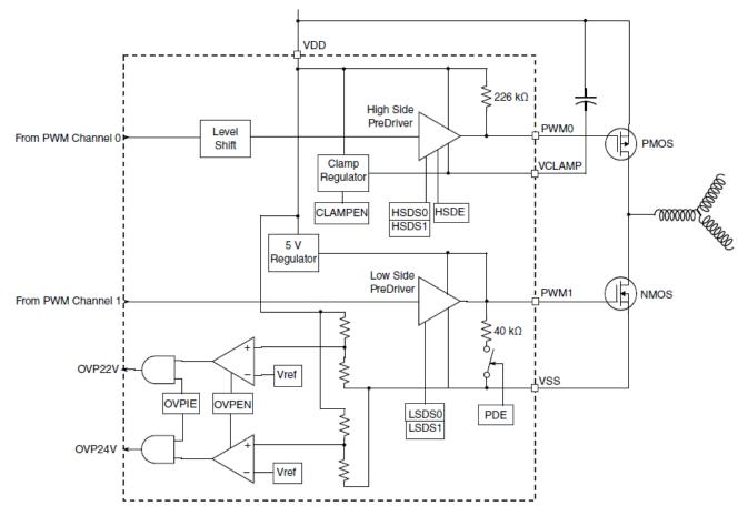
Figure 3. Pre-driver Circuit Diagram
