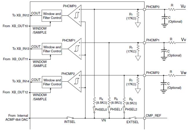
The *Figure 5* shows the block diagram of the phase detector in GDU.
