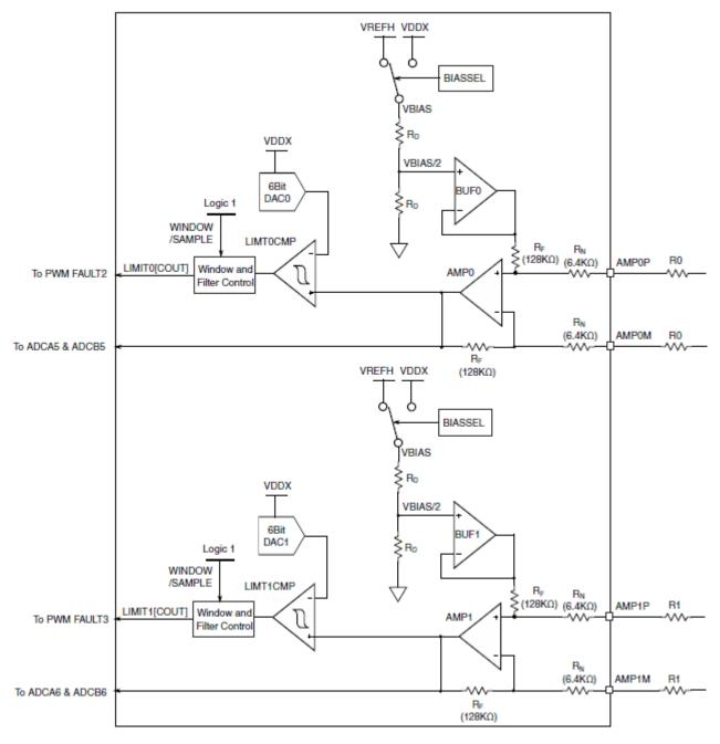
Figure 4. Current Sensor and OCP Circuit Diagram
