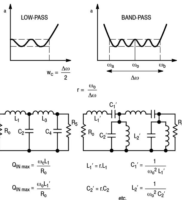
**Figure 25. Conversion from Low-Pass into Band-Pass Filter**
