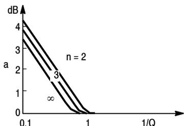
**Figure 24. Insertion Losses as a Function of 1/Q**
