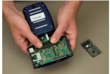
Step 3: Install the Debug board onto the Personality board.
