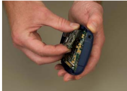
Step 2: Gently rock the CPU card back and forth to remove.
