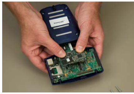
Step 4: Reinstall the CPU board
