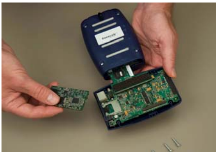
Step 4: Reinstall the CPU board
