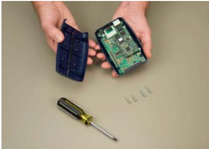
Step 1: Remove the four screws from the “Demo” configuration back enclosure. Retain the screws.
