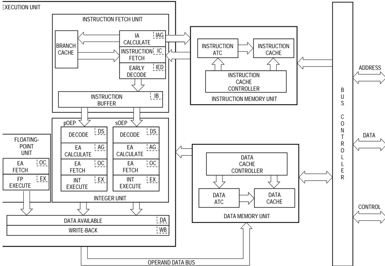
Figure 1. This represents the block diagram of the MC68060 processor. The superscalar dispatch of the MC68060 is evident in the dual pipeline shown in the Integer Unit.
