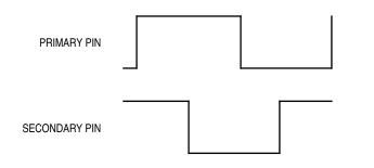
When DESIRED\_POSITION is less than CURRENT\_POSITION, the bit pattern from MSB to LSB defines the output levels at the programmed step rates, i.e., bit 14 is moved into bit 15 to define the output. The output pins are sequenced as shown.
