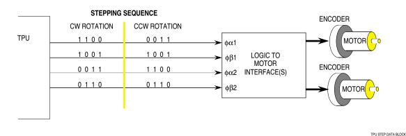
The logic output to the stepper motor varies from zero at the low state (0) to five at the high state (1). The outputs are driven from channels four through seven (TPUCH4 – TPUCH7) of the TPU. Because of the voltage difference between the logic outputs and the voltage requirement of the stepper motor, an interface must be used.
