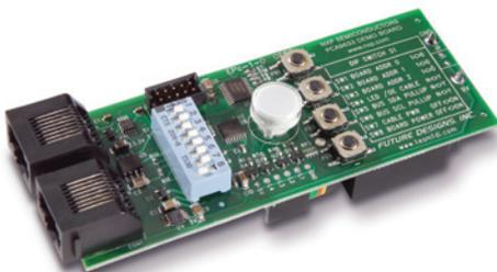
The board includes external 60-V FET drivers, which can be connected to high-current, 350-mA LEDs. A four-key keypad gives the user direct control over the RGBA color mixing and light patterns. Power can be supplied by the board's 9-V battery or via an external power connector. The RJ45 connector and cable can be used to daisy-chain multiple boards, enabling the microcontroller on one board to act as the master for up to seven additional boards.
