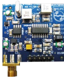
SA602AD + SA604AD OM13535 RF = 45 MHz; IF = 455 kHz
