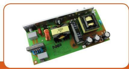
Simplifying the design of highefficiency resonant power supplies
