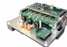
EV-INVERTER power inverter control reference design for electric vehicle traction motors and DC to DC converters
