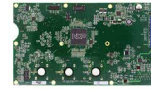
EV-INVERTERHDBT power inverter control (ICP 2.0) reference design for electric vehicle high-voltage traction inverters, using IGBT power modules
