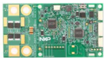
RDDRONE-BMS772 3 to 6 cell BMS on mobile robotics (drones and rovers) reference design
