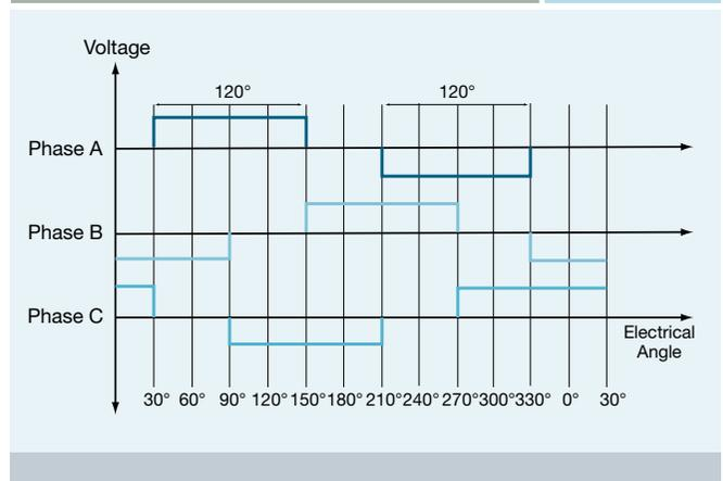
The motor can have more than one pole-pair per phase. The number of pole-pairs per phase defines the ratio between the electrical revolution and the mechanical revolution. For example, the BLDC motor shown has three pole-pairs per phase, which represents three electrical revolutions per mechanical revolution.
