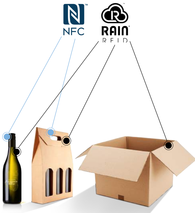
RFID-NFC identifies items at the unit, carton, or pallet level
