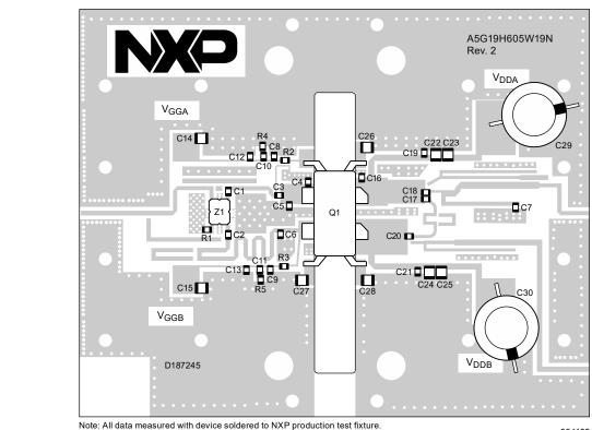
Figure 3. A5G19H605W19N production test fixture component layout
