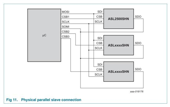
During the SPI data transfer, the identifier byte and the actual content of the addressed registers is returned via the SDO pin. The same happens for pure read accesses. Here the read-only bit must be set to 1. The content of the data bytes that are transmitted to the ASL2500SHN is ignored.
