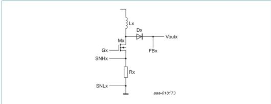
Fig 4. Phase of the boost converter with IC and application connections
