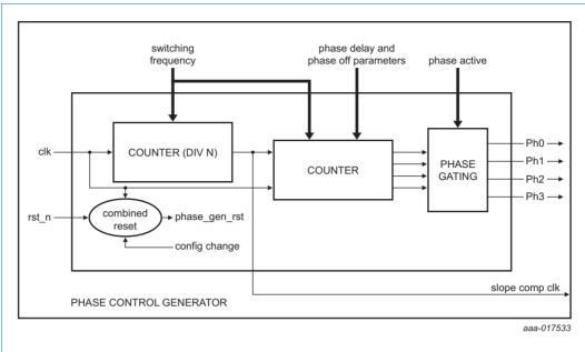
Fig 6. Phase control generator
