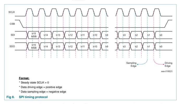
The data bits of the ASL2500SHN are arranged in registers of one-byte length. Each register is assigned to a 7-bit address. For writing into a register, 2 bytes must be sent to the LED driver. The first byte is an identifier byte that consists of the 7-bit address and one read-only bit. For writing, the read-only bit must be set to 0. The second byte is the data that is written into the register. So an SPI access consists of at least 16 bit.
