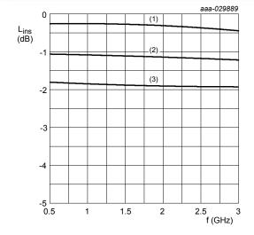
Diode inserted in series with a 50  $\Omega$  strip line circuit and biased via the analyzer T-network; T<sub>amb</sub> = 25 °C
