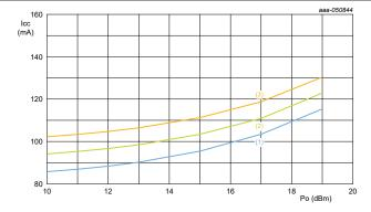
Figure 3.  $I_{cc}$  versus  $P_{out}$  over frequency at 25  $^{o}$ C
