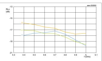
Figure 9. RLi versus frequency over temperature
