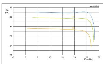
Figure 7. Gain versus Pout over temperature at 5 GHz
