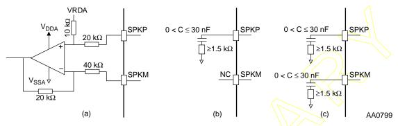
Figure 4-2 Codec Output Configurations
