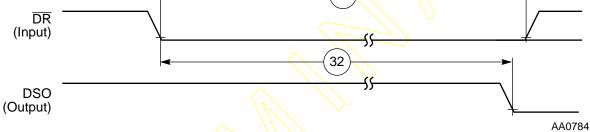
Figure 2-13 Recovery from Wait/Stop State Using DR—Asynchronous Timing
