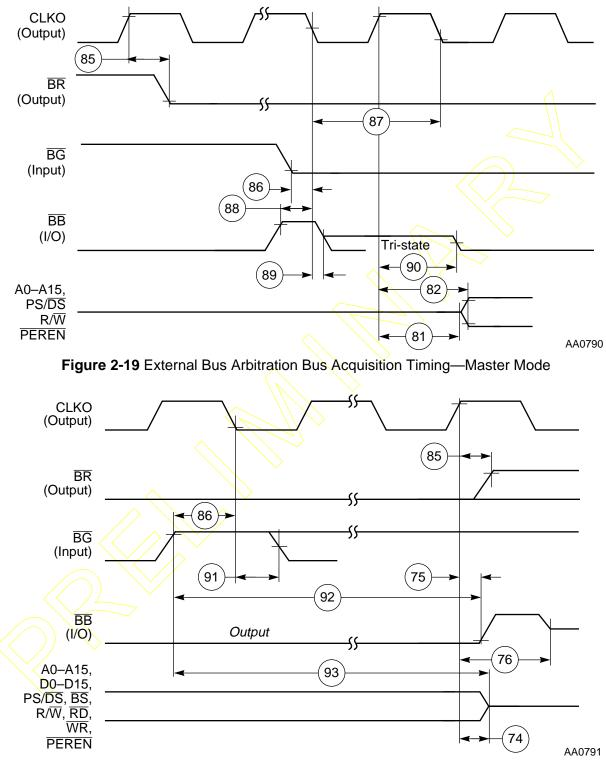
Figure 2-20 External Bus Arbitration Bus Release Timing-Master Mode
