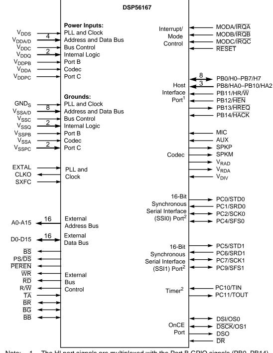
Note: The HI port signals are multiplexed with the Port B GPIO signals (PB0–PB14). 1. The 16-bit SSI and Timer signals are multiplexed with the Port C GPIO signals 2. (PC0-PC2, PC4-PC7, and PC9-PC11).
