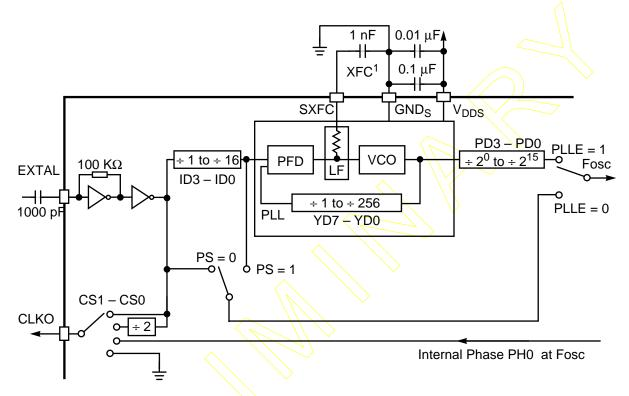
Note: 1. Must be a low leakage capacitor and must be located very close to the SXFC and VDDS pins.
