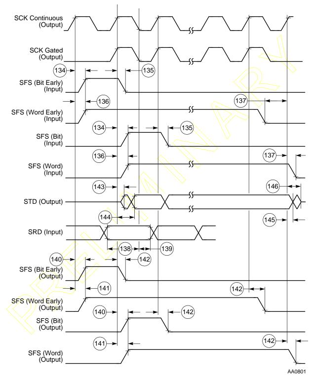
Figure 2-28 SSI Internal Clock Timing
