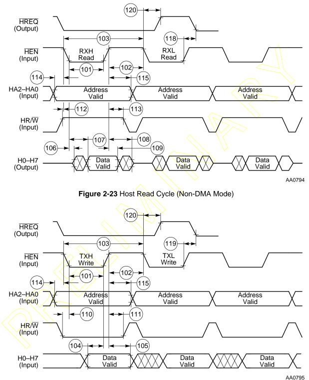
Figure 2-24 Host Write Cycle (Non-DMA Mode)
