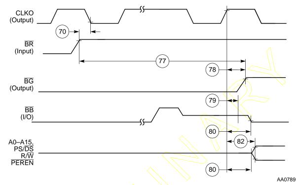
Figure 2-18 External Bus Arbitration Bus Acquisition Timing—Slave Mode
