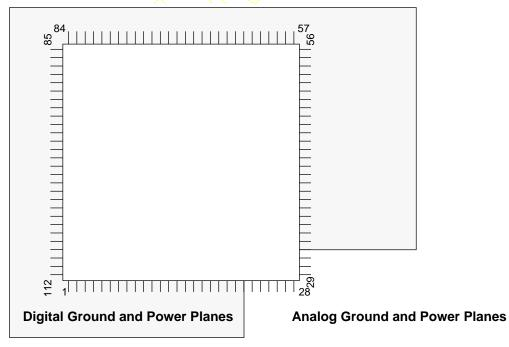
Figure 4-3 Recommended Ground and Power Plane Layout
