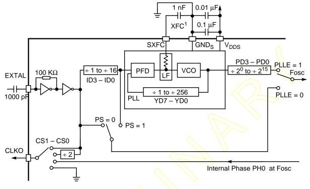
Note: 1. Must be a low leakage capacitor and must be located very close to the SXFC and VDDS pins.
