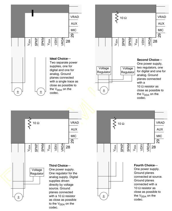
Figure 4-6 Four Possible Power Supply Connections
