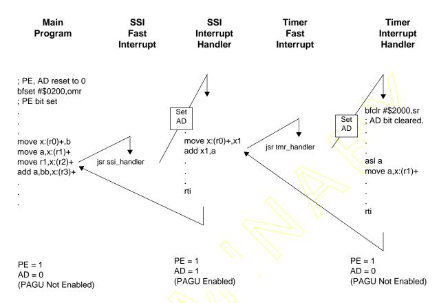
Figure 4-15 PAGU Operation During Normal and Nested Long Interrupt Service Routine
