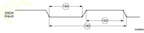
Figure 2-32 OnCE Serial Clock Timing
