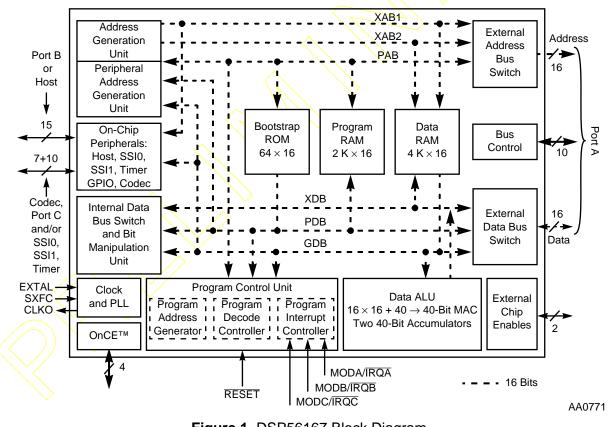
Figure 1 DSP56167 Block Diagram
