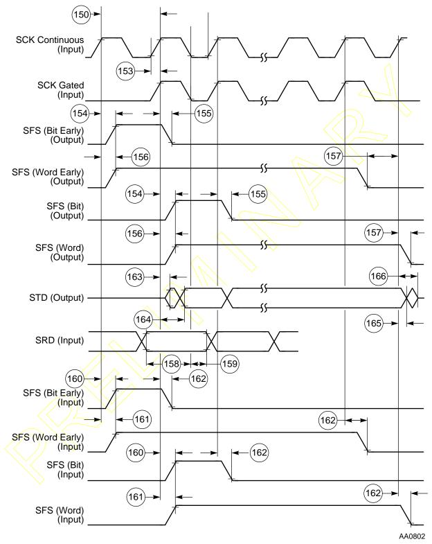
Figure 2-29 SSI External Clock Timing
