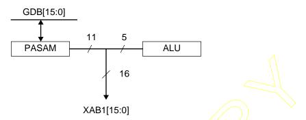
Figure 4-8 Programmable Absolute Short Addressing Mode Architecture
