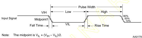
Note: The midpoint is  $V_{IL} + (V_{IH} - V_{IL})/2$ .
