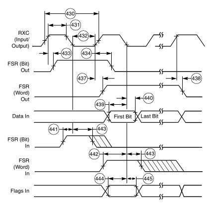
Figure 2-39. ESSI Receiver Timing
