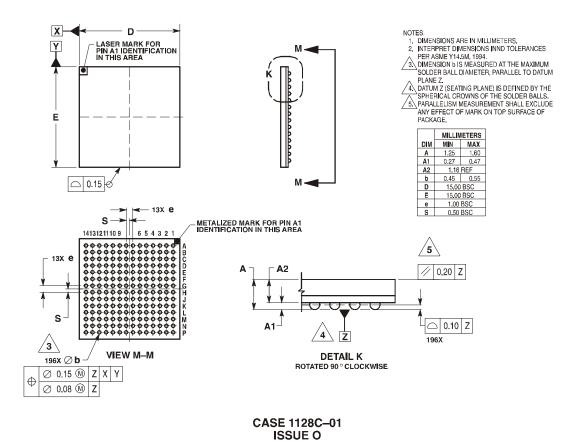
Figure 3-6. DSP56303 Mechanical Information, 196-pin MAP-BGA Package
