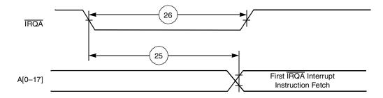
Figure 2-10. Recovery from Stop State Using IRQA Interrupt Service
