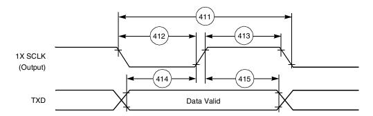
Figure 2-37. SCI Asynchronous Mode Timing
