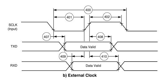
Figure 2-36. SCI Synchronous Mode Timing
