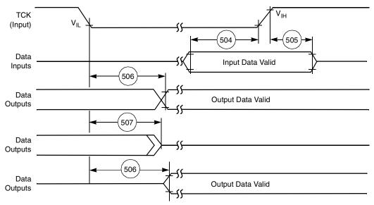
Figure 2-45. Boundary Scan (JTAG) Timing Diagram
