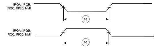
Figure 2-6. External Interrupt Timing (Negative Edge-Triggered)
