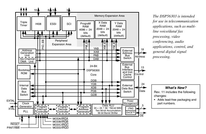
Figure 1. DSP56303 Block Diagram
