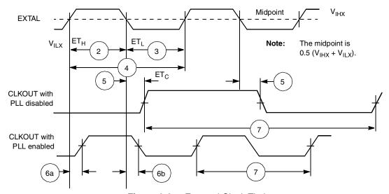
Figure 2-2. External Clock Timing
