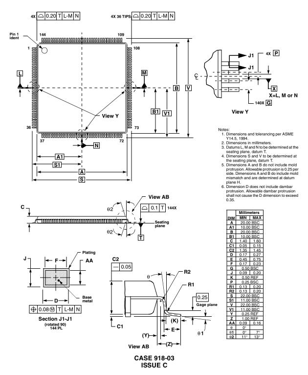
Figure 3-3. DSP56303 Mechanical Information, 144-pin TQFP Package
