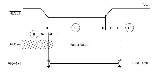
Figure 2-3. Reset Timing
