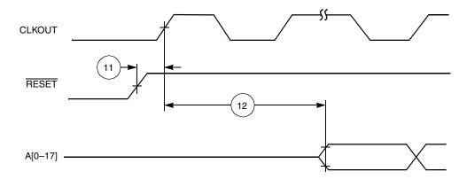
Figure 2-4. Synchronous Reset Timing
