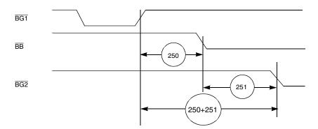
Figure 2-26. Asynchronous Bus Arbitration Timing
