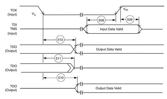
Figure 2-46. Test Access Port Timing Diagram
