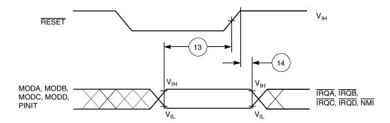
Figure 2-8. Operating Mode Select Timing
