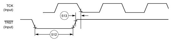
Figure 2-47. TRST Timing Diagram
