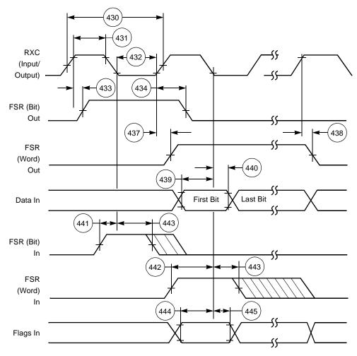
Figure 2-25. ESSI Receiver Timing
