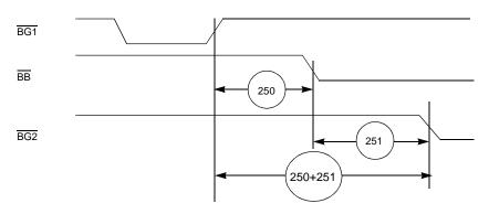
Figure 2-12. Asynchronous Bus Arbitration Timing
