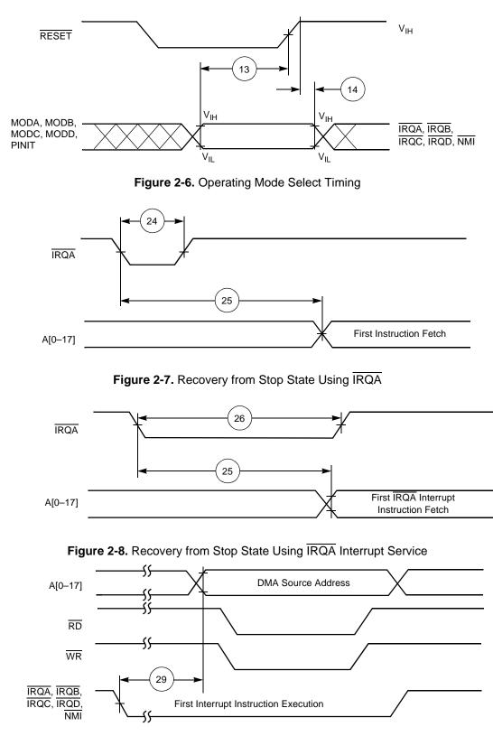
Figure 2-9. External Memory Access (DMA Source) Timing
