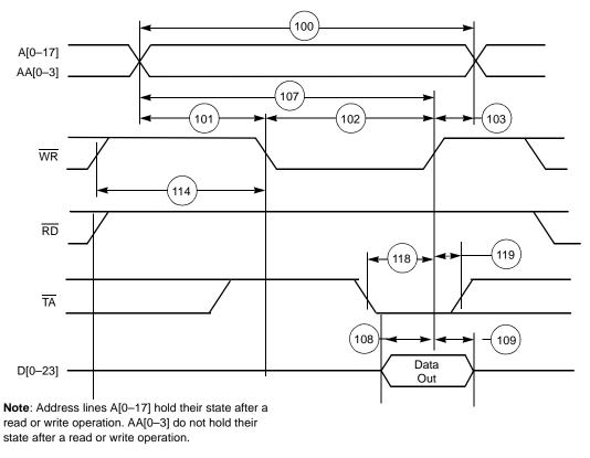
Figure 2-11. SRAM Write Access
