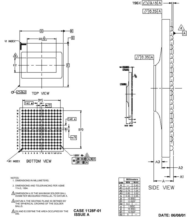
Figure 3-3. DSP56321T Mechanical Information, 196-pin FC-PBGA Package
