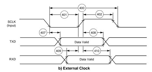
Figure 2-22. SCI Synchronous Mode Timing
