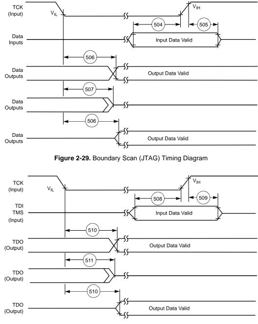
Figure 2-30. Test Access Port Timing Diagram
