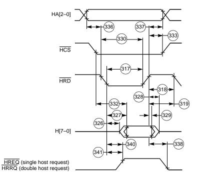
Figure 2-15. Read Timing Diagram, Non-Multiplexed Bus, Double Data Strobe
