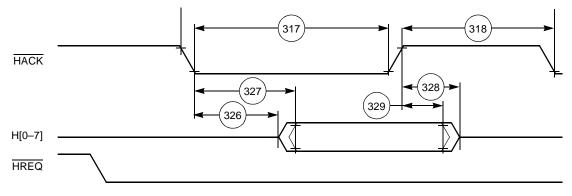
Figure 2-13. Host Interrupt Vector Register (IVR) Read Timing Diagram
