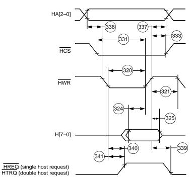
Figure 2-17. Write Timing Diagram, Non-Multiplexed Bus, Double Data Strobe
