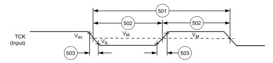
Figure 2-28. Test Clock Input Timing Diagram
