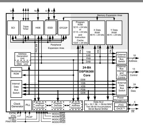
Figure 1. DSP56321T Block Diagram
