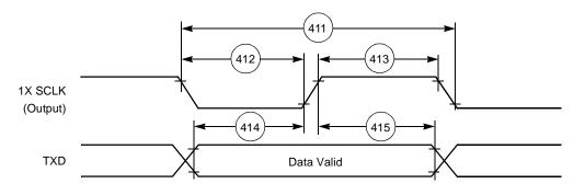
Figure 2-23. SCI Asynchronous Mode Timing
