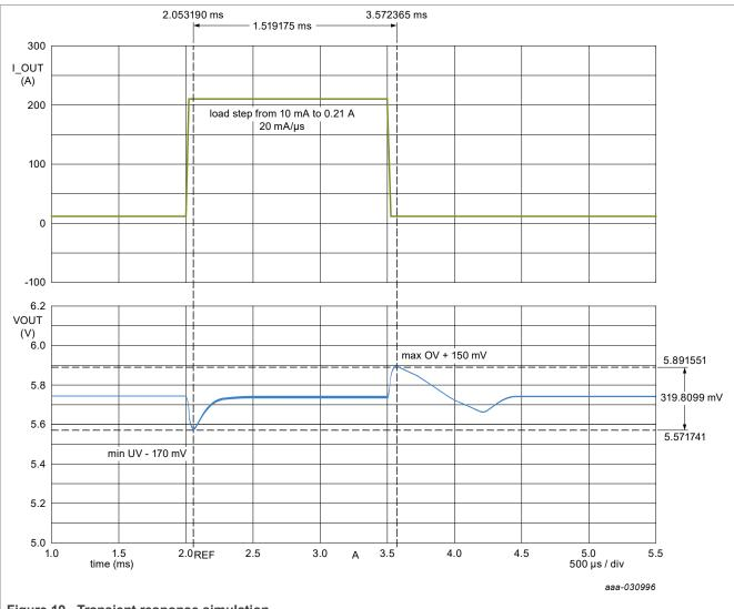
Figure 19. Transient response simulation
