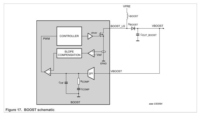
It is recommended to select a Schottky diode for D<sub>BOOST</sub> to limit the impact on the SMPS efficiency.
