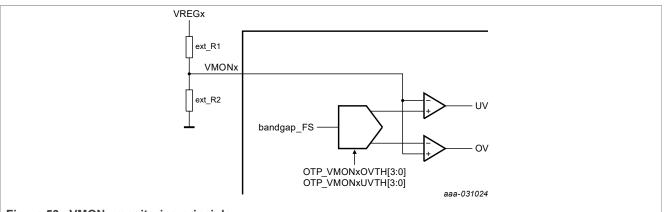
Figure 53. VMONx monitoring principle
