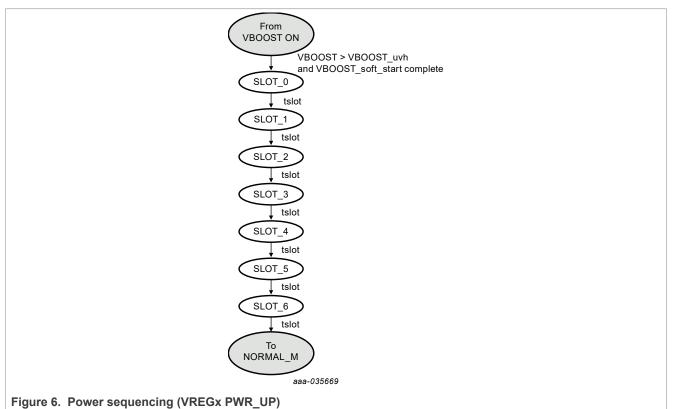
Each regulator is assigned to a SLOT by OTP configuration using OTP\_VB1S[2:0] for BUCK1, OTP\_VB2S[2:0] for BUCK2, OTP\_VB3S[2:0] for BUCK3, OTP\_LDO1S[2:0] for LDO1 and OTP\_LDO2S[2:0] for LDO2.
