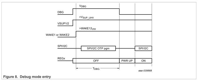
When the DBG pin is asserted low after  $T_{DBG}$  without SPI/I2C command access, the device starts with the internal OTP configuration.
