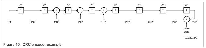
The effect of CRC encoding procedure is shown in the following table. The seed value is appended into the most significant bits of the shift register.
