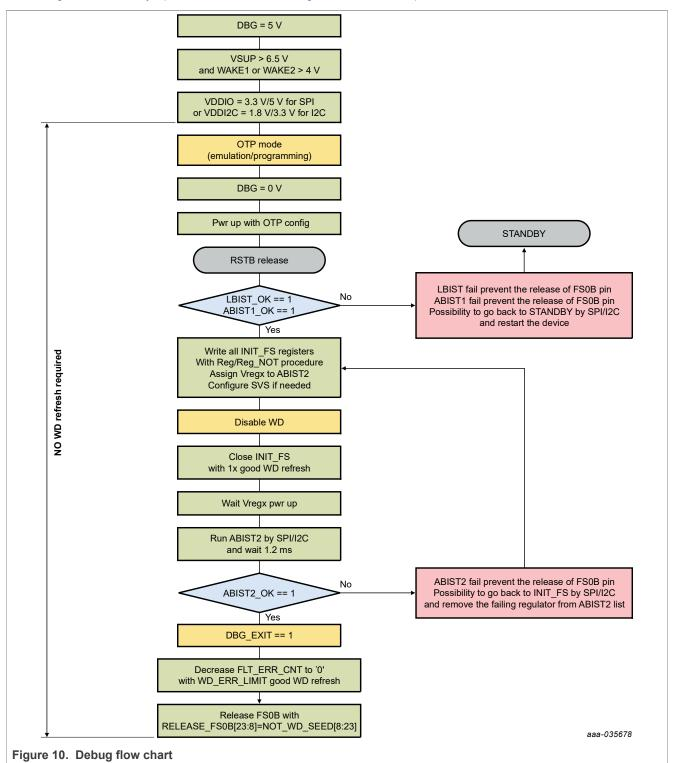
*Note:* Disabling the watchdog before INIT\_FS closure and Debug mode exit by SPI/I2C allows FS0B release. Otherwise, FS0B is stuck low in Debug mode.
