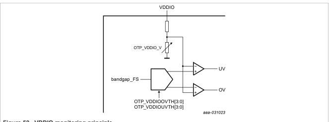
Figure 52. VDDIO monitoring principle
