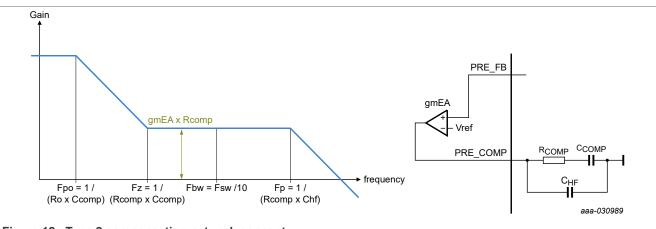
Figure 12. Type 2 compensation network concept
