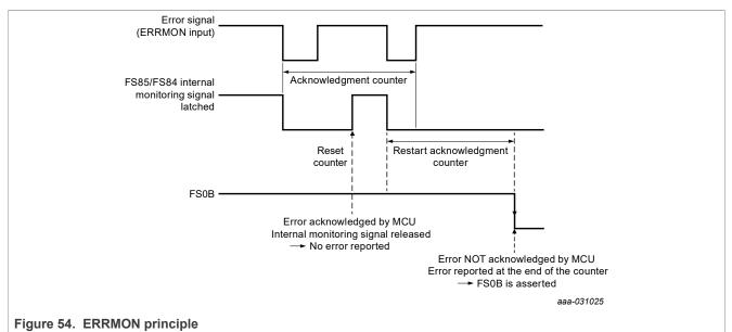
When ERRMON fault is detected, the fail-safe reaction on RSTB and/or FS0B is configurable with the ERRMON\_FS\_IMPACT bit during the INIT\_FS phase.
