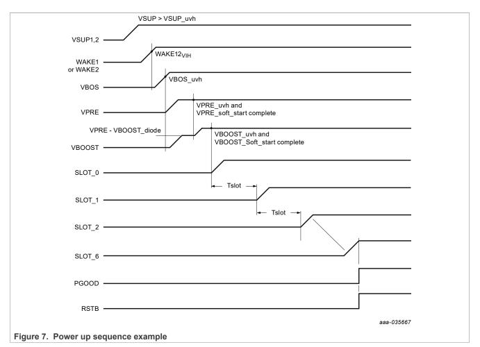
PGOOD and RSTB release depends on the combination of the power up sequence and what regulator is assigned to PGOOD and ABIST1 through the voltage monitoring connection (VCOREMON, VDDIOMON and VMONx). The FS85\_FS84\_OTP\_Config file used to generate the OTP configuration of the device draws the power up sequence of an OTP configuration in the OTP conf summary sheet.
