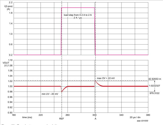
Figure 23. Transient response simulation
