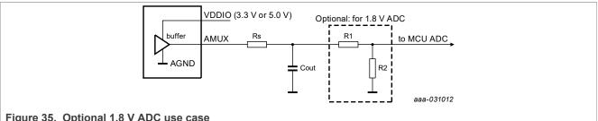
Figure 35. Optional 1.8 V ADC use case
