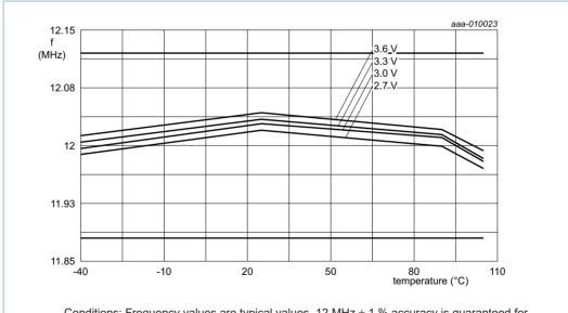
Conditions: Frequency values are typical values. 12 MHz  $\pm$  1 % accuracy is guaranteed for 2.7 V  $\leq$  V<sub>DD</sub>  $\leq$  3.6 V and T<sub>amb</sub> = –25 °C to +85 °C. Variations between parts may cause the IRC to fall outside the 12 MHz  $\pm$  1 % accuracy specification for voltages below 2.7 V.
