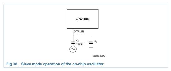
In slave mode the input clock signal should be coupled through a capacitor of 100 pF (Figure 38), with an amplitude between 200 mV (RMS) and 1000 mV (RMS). This corresponds to a square wave signal with a signal swing of between 280 mV and 1.4 V. The XTALOUT pin in this configuration can be left unconnected.
