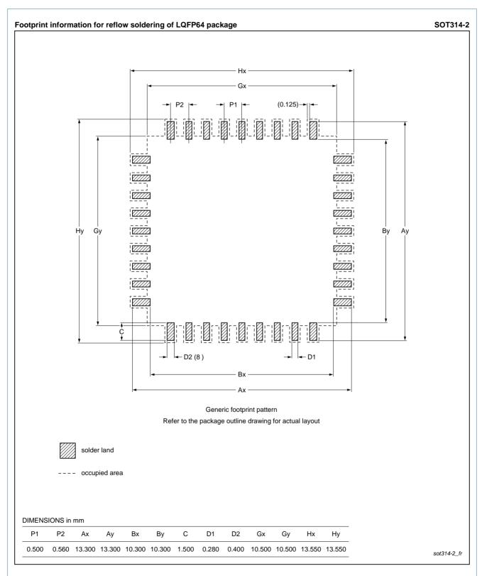
Fig 46. Reflow soldering for the LQFP64 package
