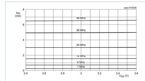
Conditions:  $T_{amb} = 25 \,^{\circ}\text{C}$ ; active mode entered executing code while (1) {} from flash; all peripherals disabled in the SYSAHBCLKCTRL register (SYSAHBCLKCTRL = 0x1F), all peripheral clocks disabled; internal pull-up resistors disabled; BOD disabled; low-current mode.
