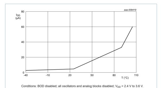
Fig 18. Power-down mode: Typical supply current I<sub>DD</sub> versus temperature for different
