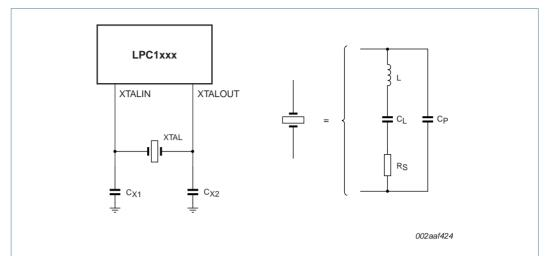
Fig 39. Oscillator modes and models: oscillation mode of operation and external crystal model used for  $C_{X1}/C_{X2}$  evaluation
