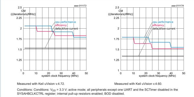
Fig 21. CoreMark score for different power mode settings of the power profiles
