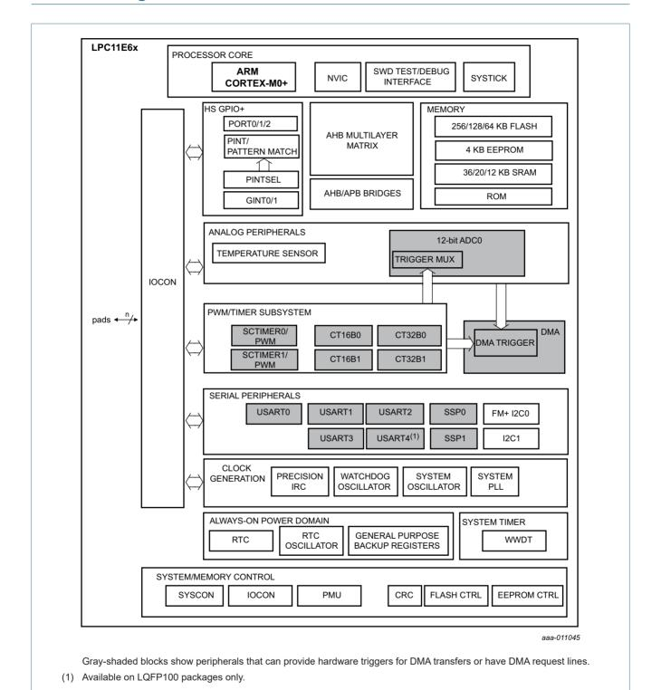
Fig 3. LPC11E6x block diagram
