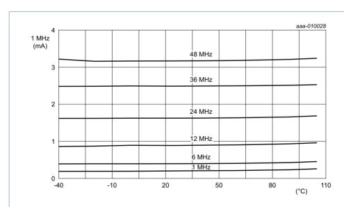
Conditions:  $V_{DD} = 3.3~V$ ; sleep mode entered from flash; all peripherals disabled in the SYSAHBCLKCTRL register (SYSAHBCLKCTRL = 0x1F) all peripheral clocks disabled; internal pull-up resistors disabled; BOD disabled; low-current mode.
