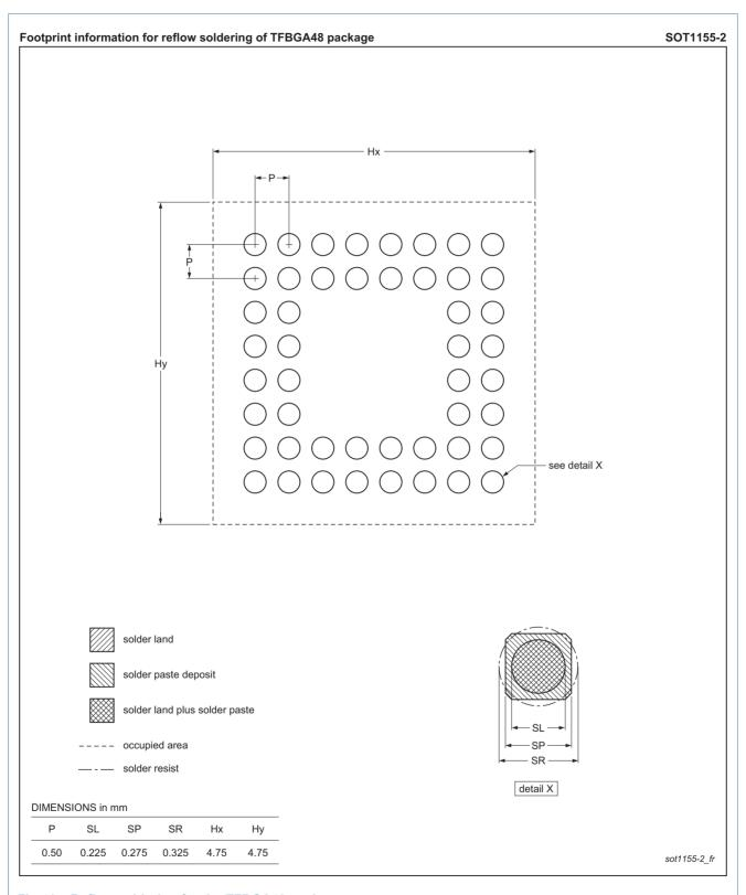
Fig 41. Reflow soldering for the TFBGA48 package
