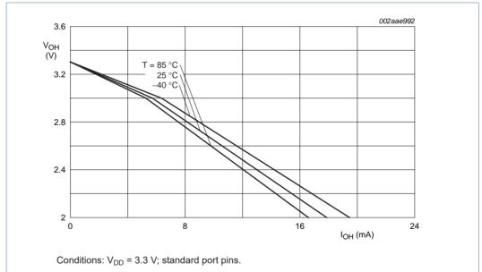
Fig 18. Typical HIGH-level output voltage  $V_{OH}$  versus HIGH-level output source current I<sub>OH</sub>
