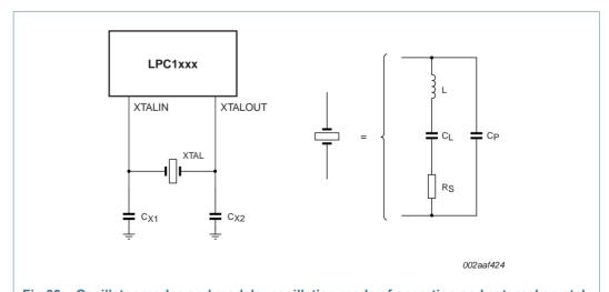
Fig 30. Oscillator modes and models: oscillation mode of operation and external crystal model used for  $C_{X1}/C_{X2}$  evaluation
