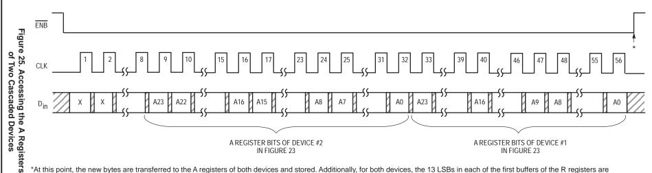
\*At this point, the new bytes are transferred to the A registers of both devices and stored. Additionally, for both devices, the 13 LSBs in each of the first buffers of the R registers are transferred to the respective R register's second buffer. Thus, the R, N, and A counters can be presented new divide ratios at the same time. The first buffer of each R register is not affected. Neither C register is affected.
