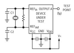
Figure 9. Test Circuit — Crystal Mode
