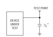
\*Includes all probe and fixture capacitance.
