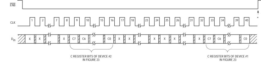
\*At this point, the new bytes are transferred to the C registers of both devices and stored. No other registers are affected.
