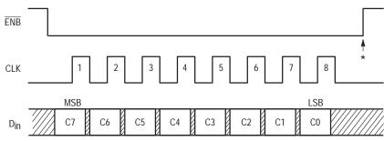
\* At this point, the new byte is transferred to the C register and stored. No other registers are affected.
