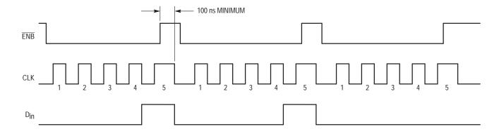
NOTE: It may not be convenient to control the ENB or CLK pins during power up per the Pin Descriptions. If this is the case, the part may be initialized through the serial port as shown in the figure above. The sequence is similar to accessing the registers except that the CLK must remain high at least 100 ns after ENB is brought high. Note that 3 groups of 5 bits are needed.
