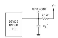
\*Includes all probe and fixture capacitance.
