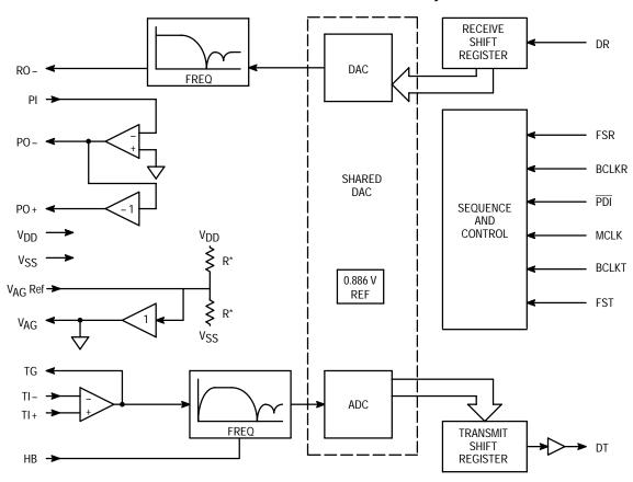
Figure 1. MC145483 13-Bit Linear PCM Codec-Filter Block Diagram
