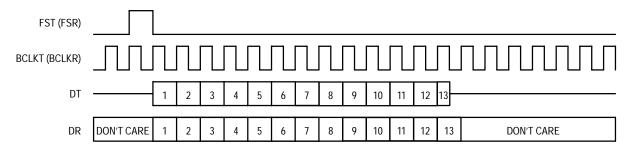
Figure 2b. Short Frame Sync (Transmit and Receive Have Individual Clocking)
