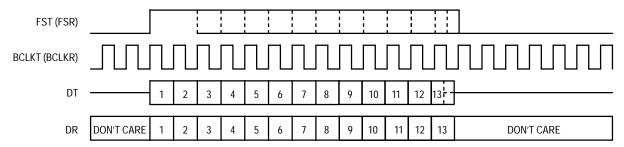
Figure 2a. Long Frame Sync (Transmit and Receive Have Individual Clocking)
