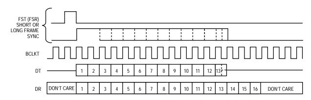
Figure 2d. Receive Gain Adjust (BCLKR = 1)
