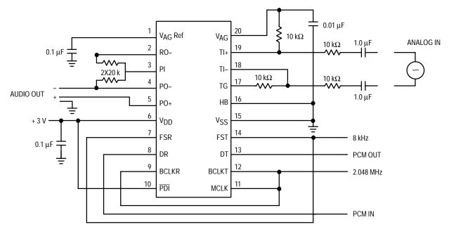
Figure 5. MC145483 Test Circuit — Signals Referenced to VAG Pin
