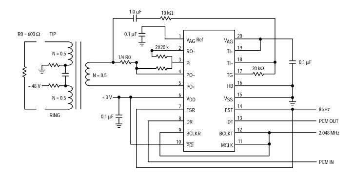
Figure 8. MC145483 Step-Up Transformer Line Interface
