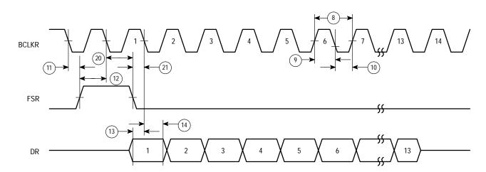
Figure 4. Short Frame Sync Timing
