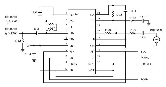
Figure 6. MC145483 Test Circuit — Signals Referenced to VSS
