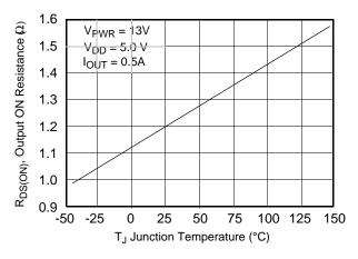
Figure 25. Maximum Output ON Resistance vs. Junction Temperature
