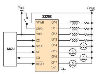
Figure 1. 33298 Simplified Application Diagram
