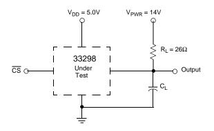
C<sub>I</sub> represents the total capacitance of the test fixture and probe.
