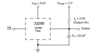
C<sub>1</sub> represents the total capacitance of the test fixture and probe.
