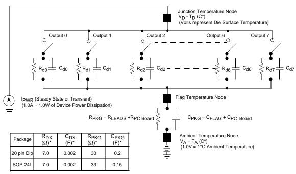
\*  $\Omega$  = °C/W, F = W s/°C, I<sub>PWR</sub> = W, and V<sub>A</sub> = °C
