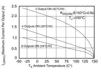
Figure 24. Maximum SOP Package Steady State Output Current vs. Ambient Temperature
