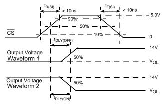
1.  $^t\text{DLY}(\text{ON})$  and  $^t\text{DLY}(\text{OFF})$  are turn-on and turn-off propagation delay times.
