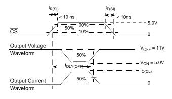
1.  $t_{\text{PDLY(OFF)}}$  is the output fault unlatch disable propagation delay time required to correctly report an output fault after  $\overline{\text{CS}}$  rises. It represents an output commanded ON while having an existing output short (over-current) to supply.
