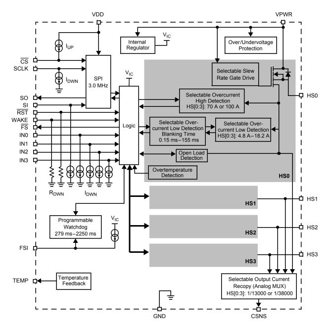
Figure 2. 33580 Simplified Internal Block Diagram
