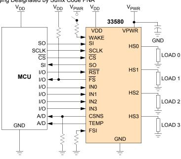
Figure 1. 33580 Simplified Application Diagram
