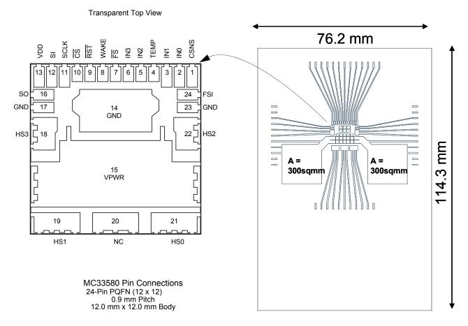
Figure 12. Thermal Test Board
