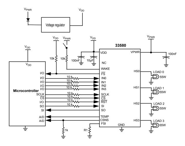
Automotive lamps do not tolerate high voltages very well. Tests of a few lamps indicate that failures can occur when 18V is applied for a few seconds. Consequently, PWM switching reduces the effective RMS voltage in order to drive bulbs safety.
