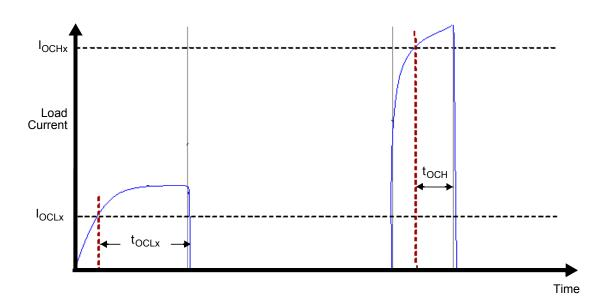
Figure 5. Overcurrent Shutdown
