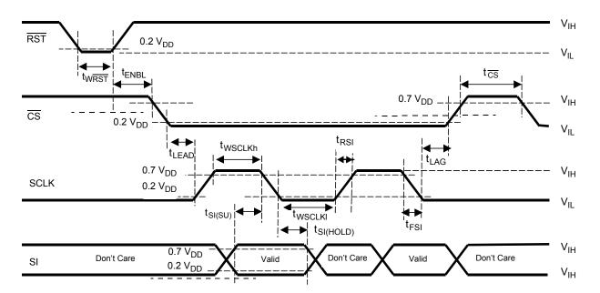
**Figure 7. Input Timing Switching Characteristics**
