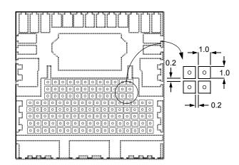
Note: Recommended via diameter is 0.5 mm. PTH (plated through hole) via must be plugged / filled with epoxy or solder mask in orde to minimize void formation and to avoid any solder wicking into the via
