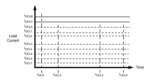
Figure 6. Overcurrent Low and High Detection
