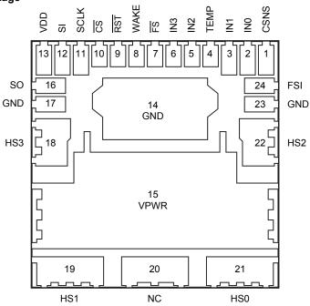
Figure 3. 33580 Pin Connections
