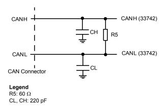
Figure 36. CAN Bus Standard Termination
