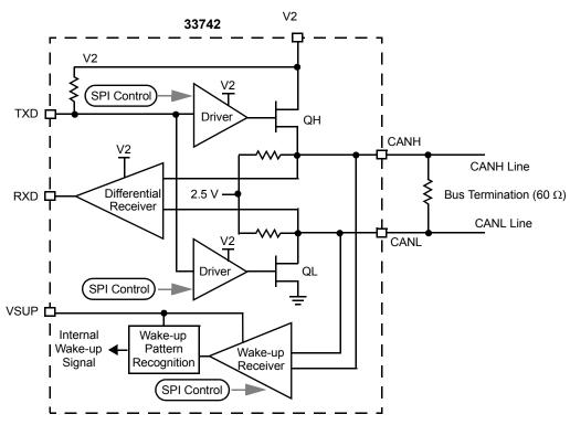
Figure 19. Simplified Block Diagram of CAN Interface
