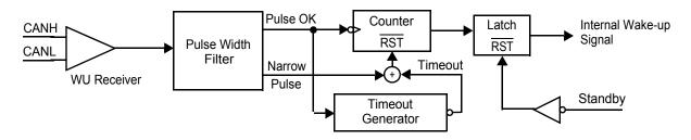
Figure 23. Wake-up Functional Block Diagram
