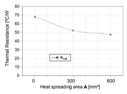
Figure 40. Device on Thermal Test Board  $\textbf{R}_{\theta \text{JA}}$
