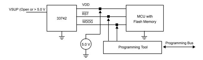
Note External supply and sources applied to VDD, RST, and WDOG test points on application circuit board.
