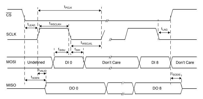
Note Incoming data at MOSI pin is sampled by the 33742 at SCLK falling edge. Outgoing data at MISO pin is set by the 33742 at SCLK rising edge (after  $t_{VALID}$  delay time).
