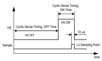
Figure 30. HS Operation When Cyclic Sense Is Selected
