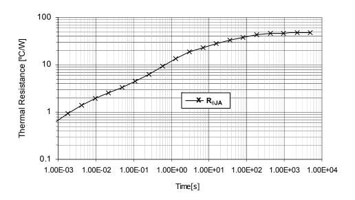
Figure 41. Transient Thermal Resistance  $R_{\theta JA,}$  1 W Step response, Device on Thermal Test Board Area A = 600 (mm²)
