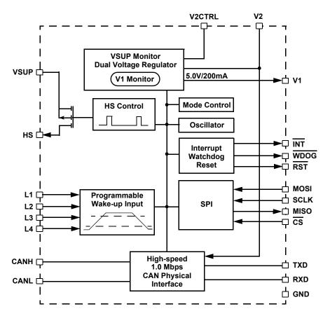
Figure 2. 33742 Simplified Internal Block Diagram
