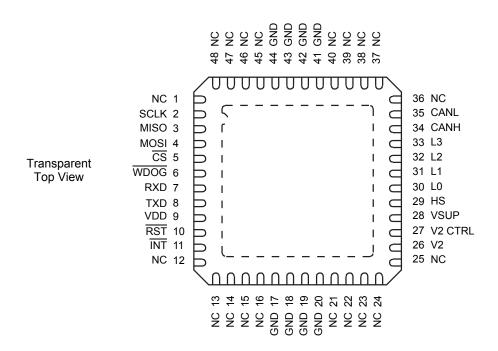
Figure 4. 33742 48-Pin Connections
