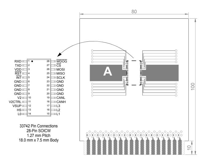
Figure 39. Thermal Test Board
