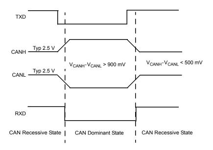
Figure 20. CAN Interface Levels
