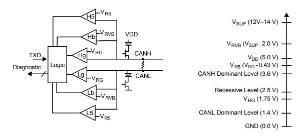
Figure 24. CAN Bus Simplified Structure
