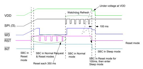
Figure 35. Under-voltage at VDD. Sleep mode selected.
