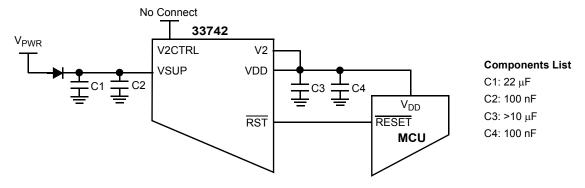
Figure 32. V2 Regulator Electrical Connection
