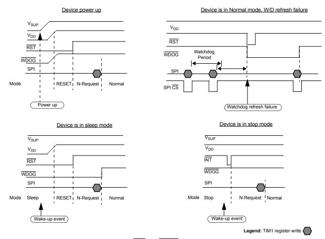
Figure 12. RST and WDOG Output Operation
