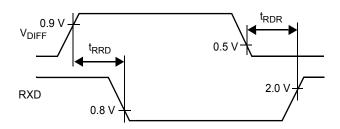
Figure 10. Propagation Delay CAN to RXD
