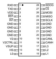
Figure 3. 33742 28-Pin Connections
