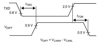
Figure 9. Propagation Delay TXD to CAN
