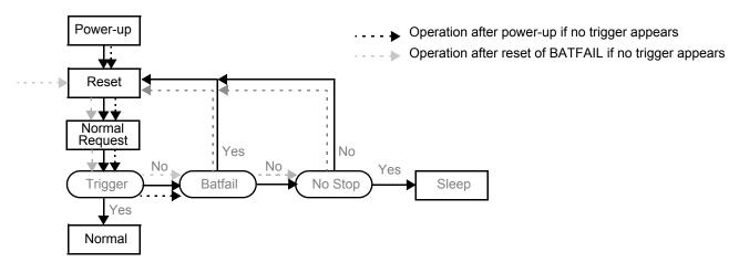
Figure 14. Operation After SBC Power-up
