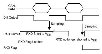
**Note** RXD Flag is neither the RXPR bit in the LPC register nor the CANF bit in INTR register.
