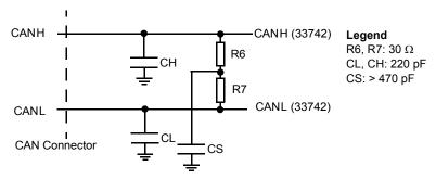
Figure 37. CAN Bus Split Termination
