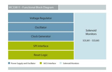
Figure 7. Functional Internal Block Diagram
