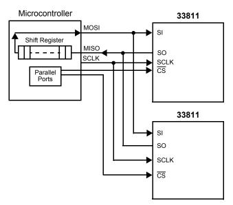
Figure 6. SPI Parallel Interface with Microprocessor
