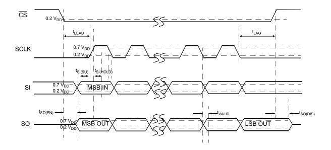
Figure 4. SPI Timing Characteristics
