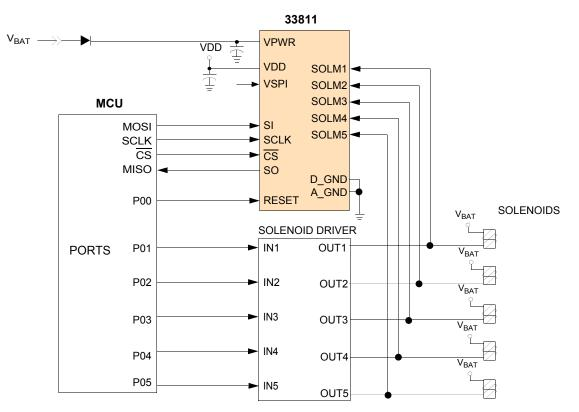
Figure 1. 33811 Simplified Application Diagram
