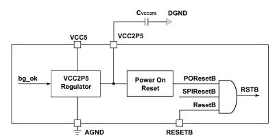
Figure 7. V<sub>CC2P5</sub> voltage regulator and power on reset overview
