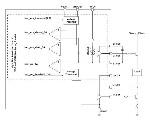
Figure 18. V<sub>DS</sub> monitors and load biasing for HS2 and HS4
