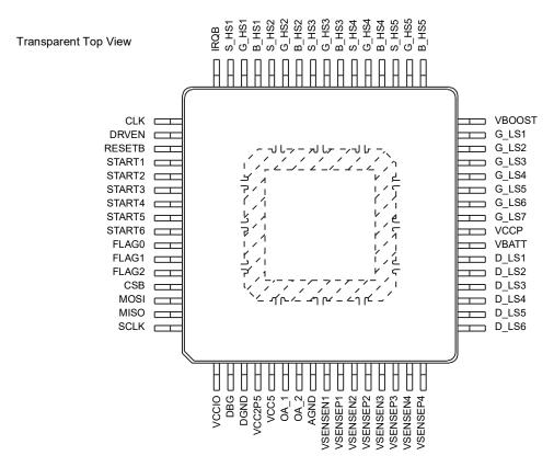
Figure 3. 33816 64-Pin LQFP-EP pinout diagram
