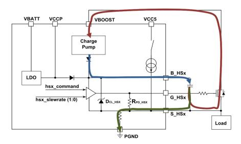
Figure 15. Booststrap load current path during start-up sequence using charge pump
