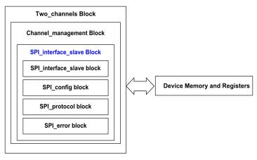
Figure 30. Spi\_interface\_slave block diagram
