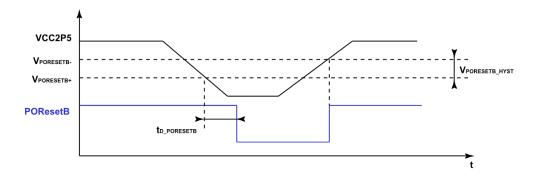
Figure 8. POResetB diagram
