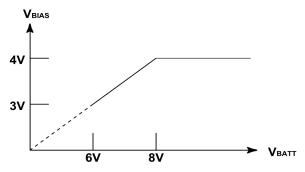
Figure 19. Biasing Voltage vs. V<sub>BATT</sub>
