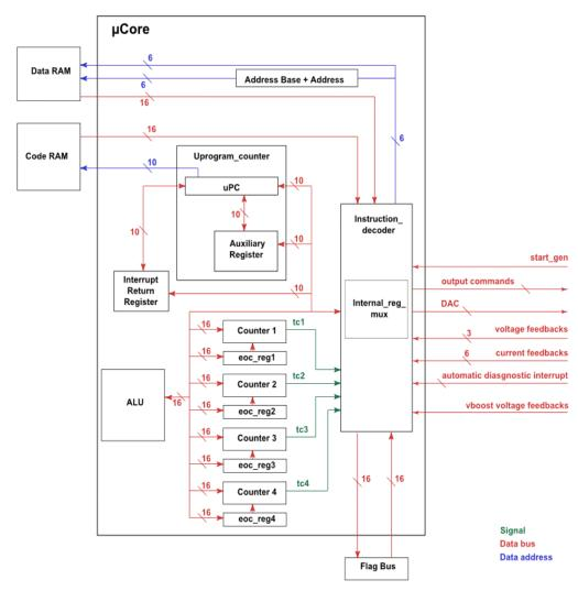
Figure 36. Microcore block diagram
