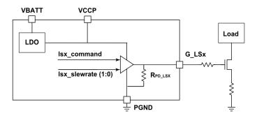
Figure 16. Low-side pre-driver block diagram
