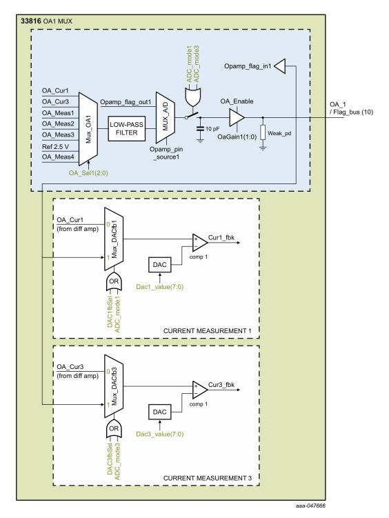
Figure 22. Measurement function OA1 detail
