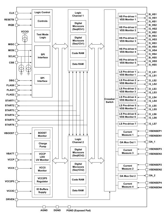
Figure 2. 33816 simplified internal block diagram
