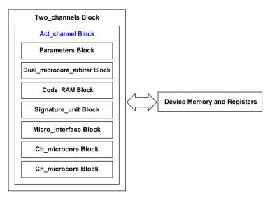
Figure 33. Act\_channels block diagram
