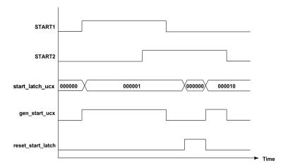
Figure 35. Smart start latch diagram
