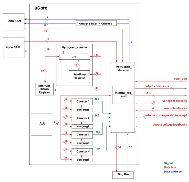
Figure 44. Microcore block diagram
