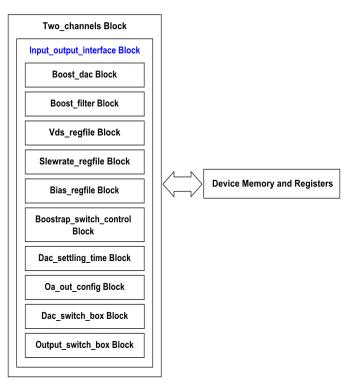
Figure 39. Input\_output\_interface block diagram
