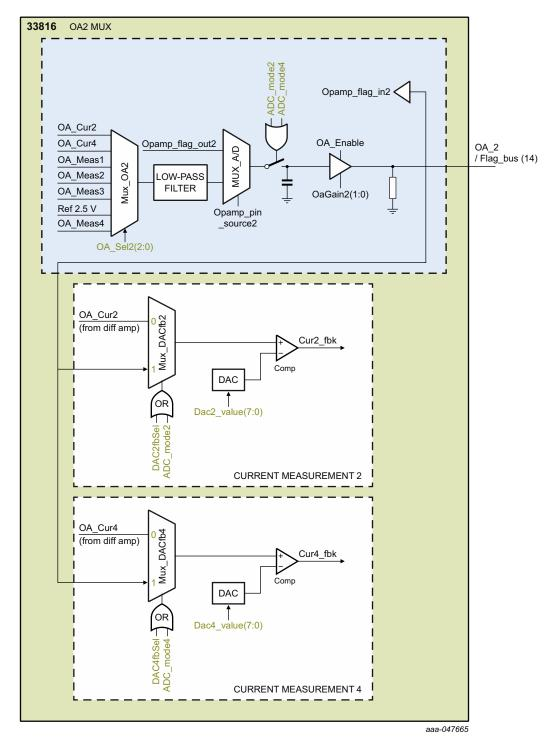
Figure 23. Measurement function OA2 detail
