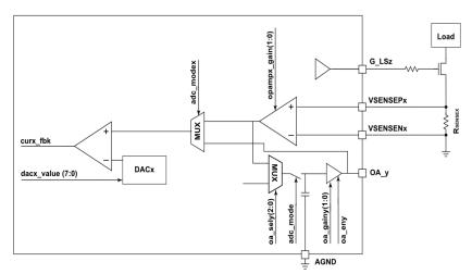
Figure 20. General purpose current measurement block diagram
