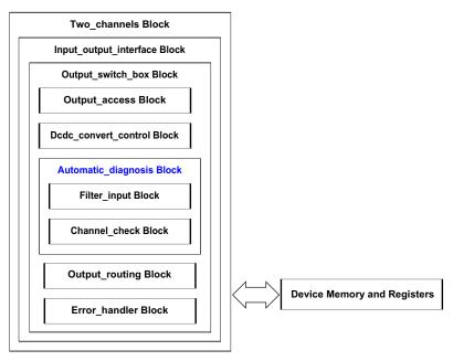
Figure 41. Automatic\_diagnosis block diagram
