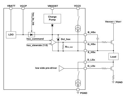
Figure 13. High-side pre-driver block diagram
