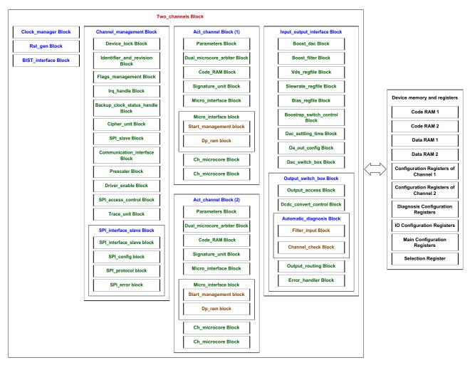
Figure 26. Device logic block hierarchic overview
