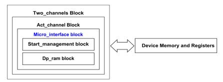
Figure 34. Micro\_interface block diagram
