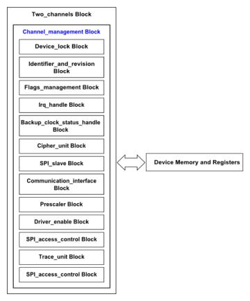
Figure 28. Channel\_management block diagram
