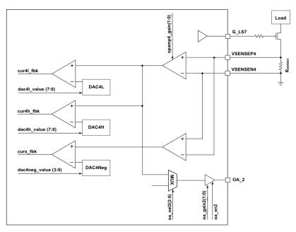
Figure 21. 4th current measurement block diagram
