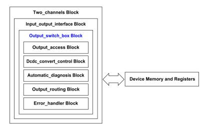
Figure 40. Output\_switch\_box block diagram
