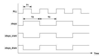
Figure 24. Timing diagrams for cksys, cksys\_cram, and cksys\_dram
