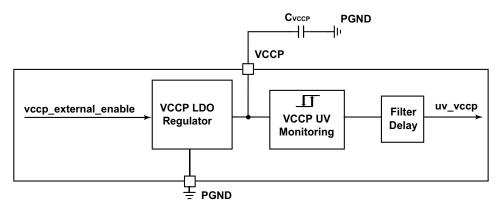
Figure 10. VCCP undervoltage monitoring
