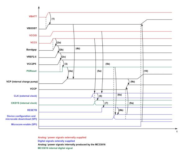
Figure 5. Power up sequence timing diagram
