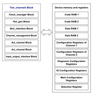
Figure 27. Two\_channels block overview
