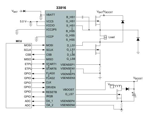
Figure 1. MC33816 simplified application diagram
