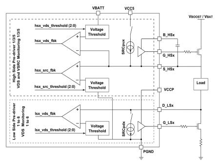
Figure 17. V<sub>DS</sub> and V<sub>SRC</sub> monitors and load biasing
