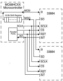
Figure 6. SPI Serial Interface with Microprocessor
