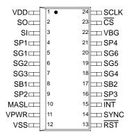
Figure 3. 33884 Pin Connections
