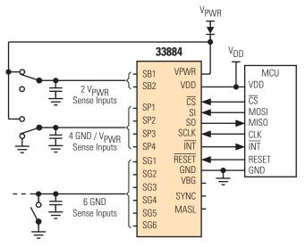
Figure 1. 33884 Simplified Application Diagram
