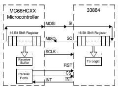
Figure 4. SPI Interface with Microprocessor
