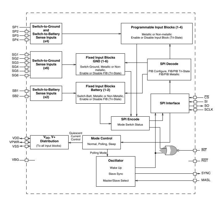
Figure 2. 33884 Simplified Block Diagram
