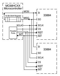
Figure 5. SPI Parallel Interface with Microprocessor
