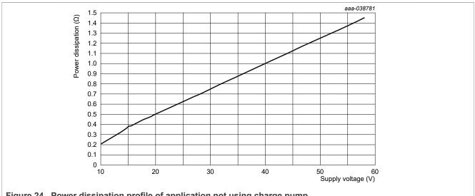
Figure 24. Power dissipation profile of application not using charge pump
