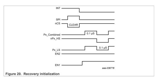
The horizontal divisions are not to scale. They are a reference to show the sequence of operation. Either individual nPx\_HS and Px\_LS or nPx\_Combined may be used. nPx\_Combined is defined as both nPx\_HS and Px\_LS tied together or operated to the same logic level simultaneously.
