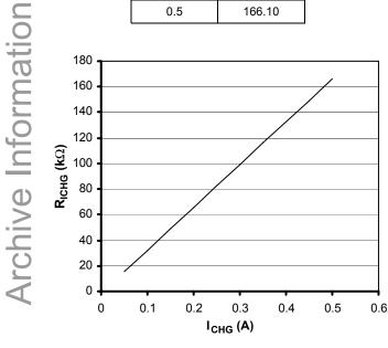
Figure 20. External Resistor (R<sub>ICHG</sub>) Value Versus Charging Current Limit Value (I<sub>CHG</sub>)
