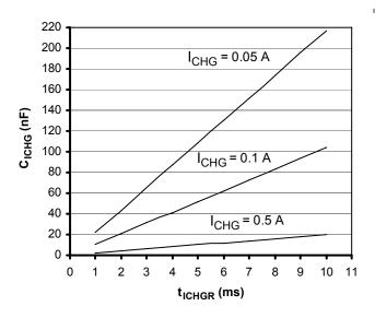
Figure 21. Charging Current External Capacitor (C<sub>ICHG</sub>) Versus Charging Current Rise Time t<sub>ICHGR</sub>
