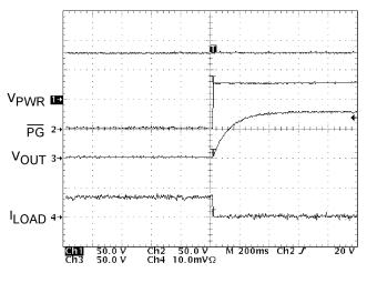
Figure 16. Overvoltage Fault
