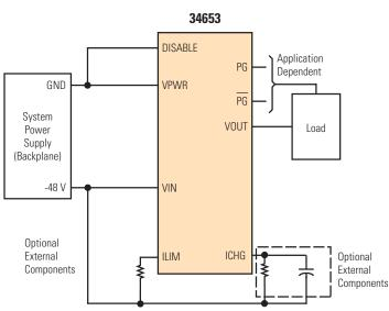
Figure 1. 34653 Simplified Application Diagram
