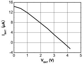
Figure 7. BAT Pin Current vs Battery Voltage in OVP V<sub>IN</sub> = 7.0V, T<sub>A</sub> = 25°C
