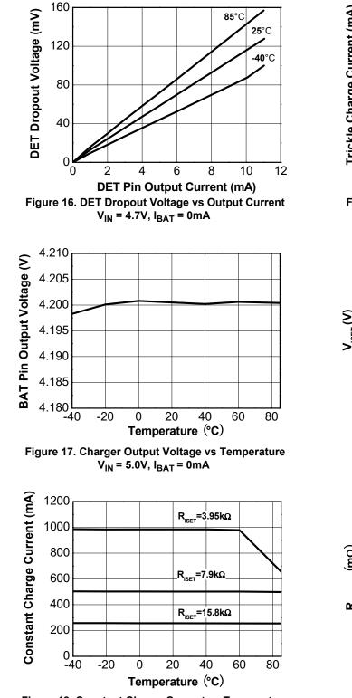
Figure 18. Constant Charge Current vs Temperature V<sub>IN</sub> = 5.0V, V<sub>BAT</sub> = 3.7V
