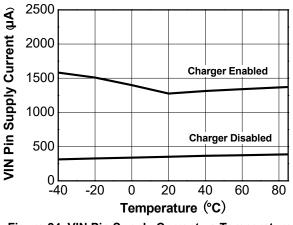
Figure 24. VIN Pin Supply Current vs Temperature  $V_{IN} = 5.0V$
