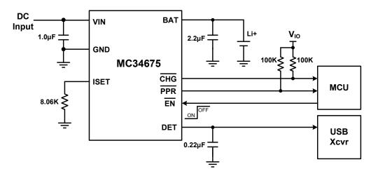
Figure 30. Li+ Battery Charger in Handheld System
