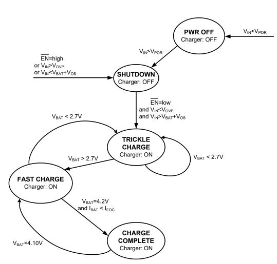
Figure 29. Charge Cycle State Diagram
