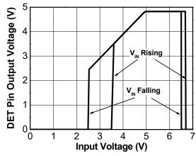
Figure 13. DET Pin Output Voltage vs Input Voltage R<sub>DET</sub> = 470 $\Omega$ , I<sub>BAT</sub> = 0mA, T<sub>A</sub> = 25°C
