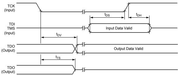
Figure 29. Test Access Port Timing Diagram
