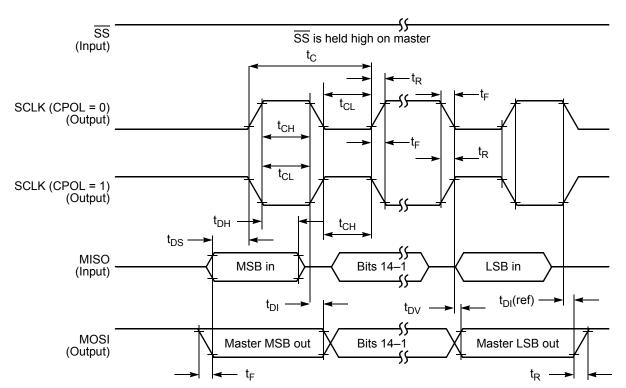
Figure 20. SPI Master Timing (CPHA = 0)
