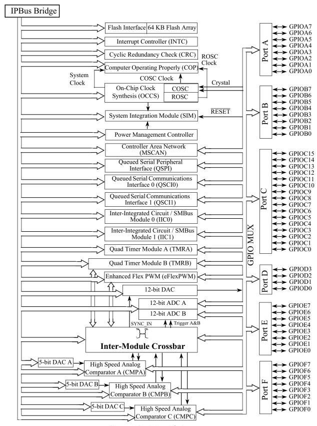
Figure 2. Peripheral Subsystem
