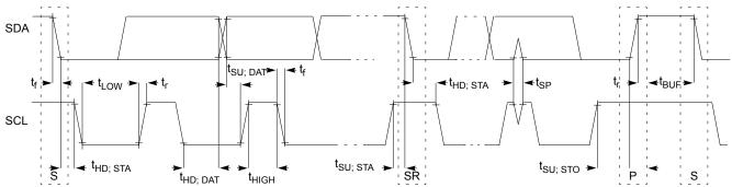
Figure 27. Timing Definition for Standard Mode Devices on the I<sup>2</sup>C Bus
