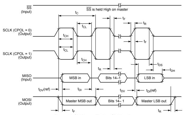
Figure 21. SPI Master Timing (CPHA = 1)
