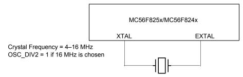
Figure 9. Typical Crystal Oscillator Circuit without Frequency Compensation Capacitor
