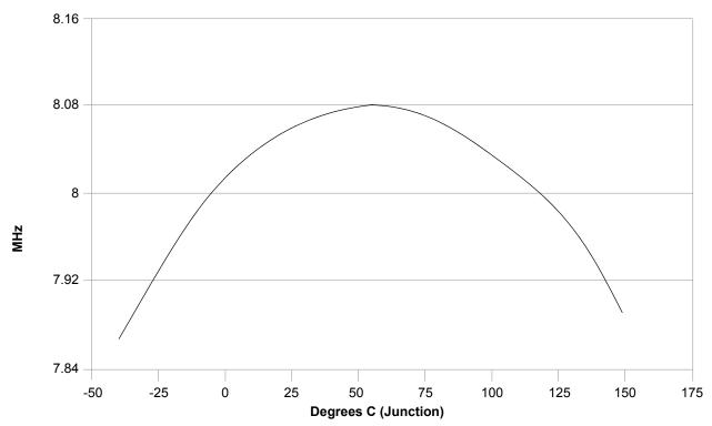
Figure 18. Relaxation Oscillator Temperature Variation (Typical) After Trim
