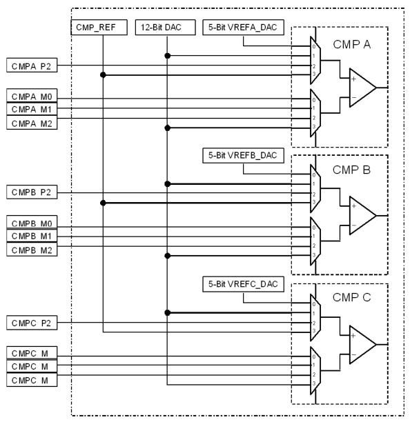
Figure 12. On-Chip Comparator Connections
