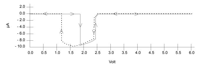
Figure 14. I<sub>IN</sub>/I<sub>OZ</sub> versus V<sub>IN</sub> (Typical; Pull-Up Disabled)
