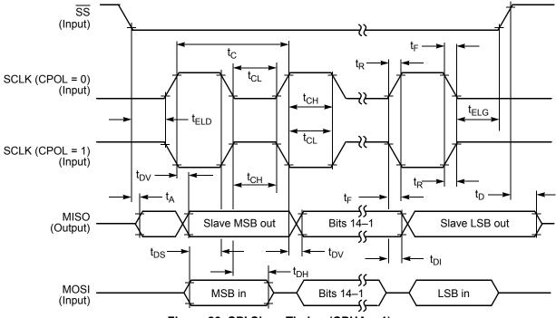
Figure 23. SPI Slave Timing (CPHA = 1)
