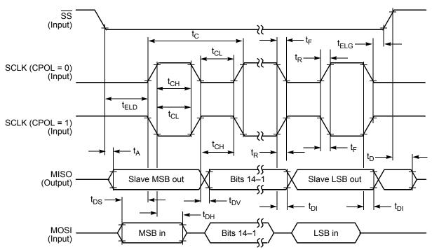
Figure 22. SPI Slave Timing (CPHA = 0)
