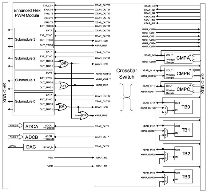
Figure 13. Crossbar Switch Connections
