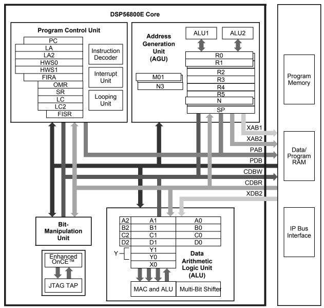
Figure 1. 56800E Core Block Diagram
