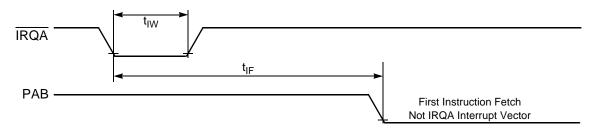
Figure 10-8 Recovery from Stop State Using Asynchronous Interrupt Timing
