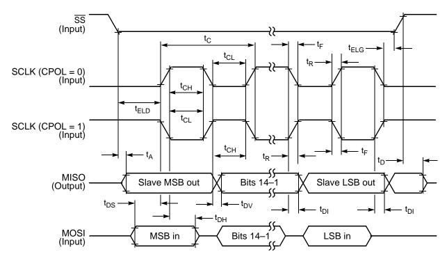
Figure 10-11 SPI Slave Timing (CPHA = 0)
