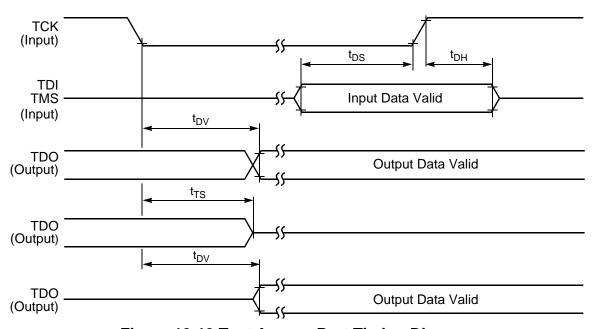
Figure 10-19 Test Access Port Timing Diagram
