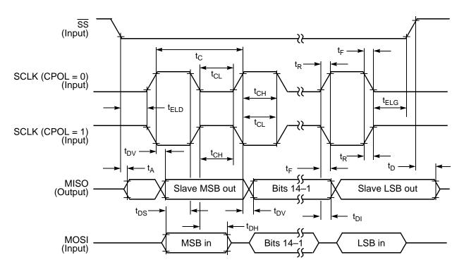
Figure 10-12 SPI Slave Timing (CPHA = 1)
