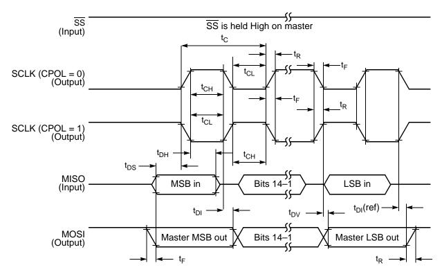
Figure 10-9 SPI Master Timing (CPHA = 0)
