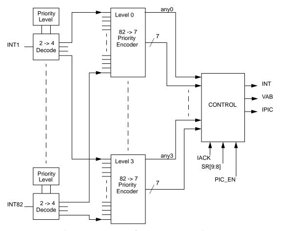
Figure 5-1 Interrupt Controller Block Diagram
