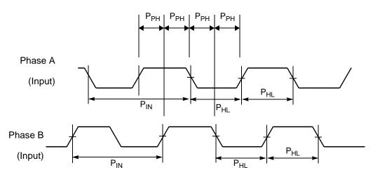
Figure 10-14 Quadrature Decoder Timing
