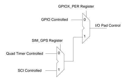
Figure 6-10 Overall Control of Pads Using SIM\_GPS Control
