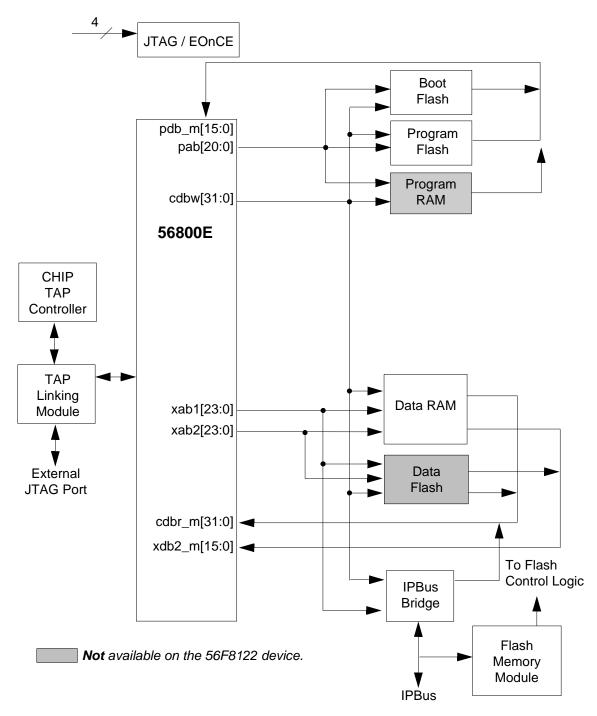
Figure 1-1 System Bus Interfaces
