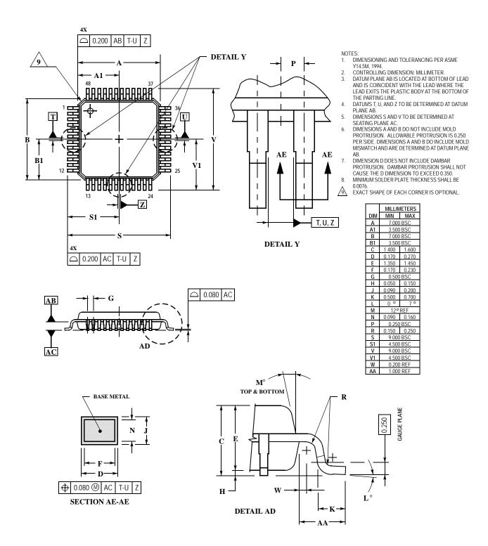
Figure 11-3 48-Pin LQFP Mechanical Information
