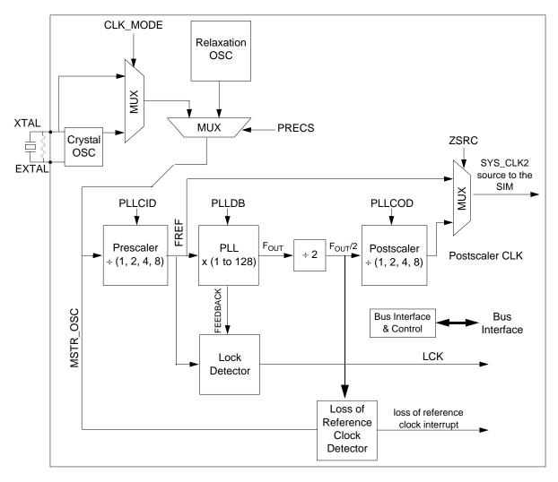
**Figure 3-4 Internal Clock Operation**
