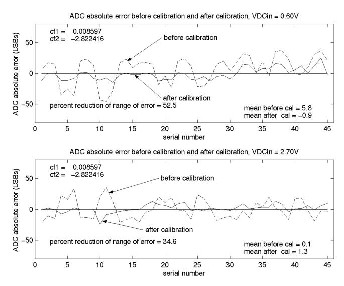
Figure 10-20 ADC Absolute Error Over Processing and Temperature Extremes Before and After Calibration for VDC<sub>in</sub> = 0.60V and 2.70V
