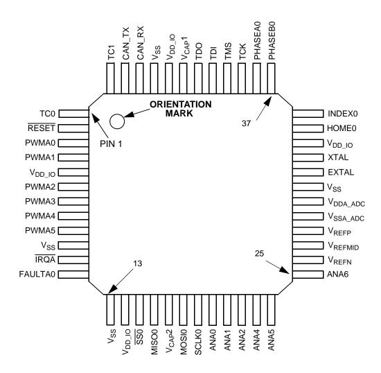
Figure 11-1 Top View, 56F8322 48-Pin LQFP Package
