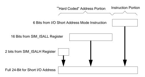
Figure 6-13 I/O Short Address Determination
