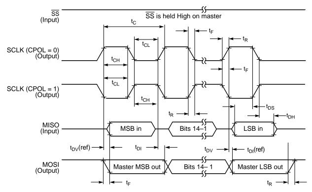
Figure 10-10 SPI Master Timing (CPHA = 1)
