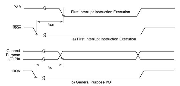
Figure 10-7 External Level-Sensitive Interrupt Timing
