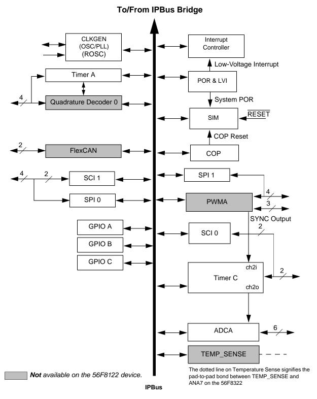
Figure 1-2 Peripheral Subsystem
