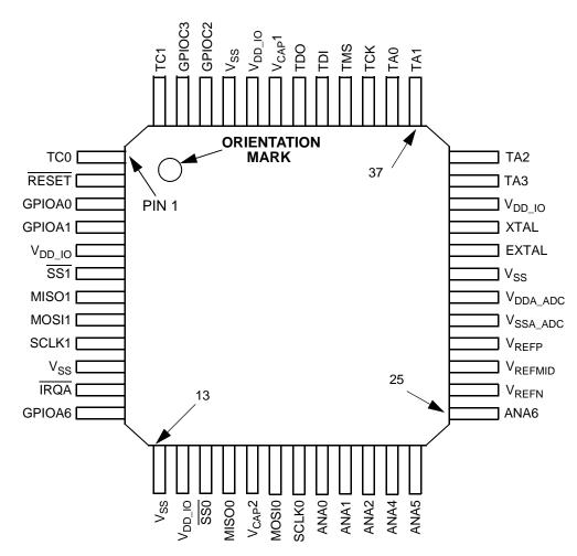
Figure 11-2 Top View, 56F8122 48-Pin LQFP Package
