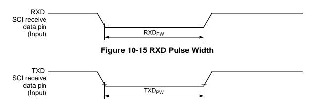
Figure 10-16 TXD Pulse Width
