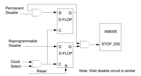
Figure 6-16 Internal Stop Disable Circuit
