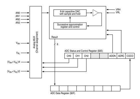
Figure 7-1 ADC Converter Block Diagram
