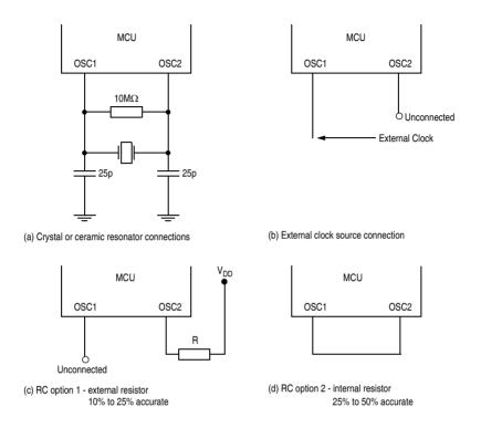
Figure 2-1 Oscillator Connections
