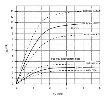
Figure 3-2 Typical  $I_{OL}$  vs  $V_{OL}$  @ $V_{DD}$ =5V
