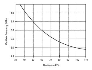
Figure 2-2 Typical Oscillator Frequency for Selected External Resistor
