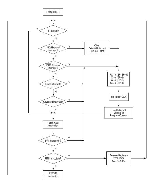
Figure 5-2 Hardware Interrupt Processing Flowchart
