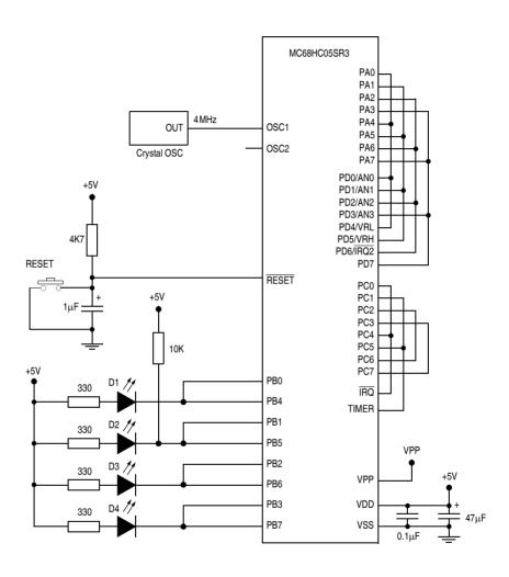
Figure 10-1 MC68HC05SR3 Self-Check Circuit
