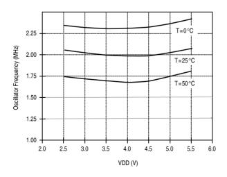
Figure 2-3 Typical Oscillator Frequency for Wire-Strap Connection
