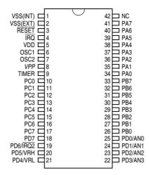
Figure 2-5 Pin Assignment for 42-pin SDIP
