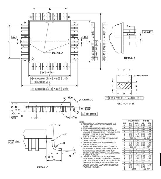
Figure 12-3 44-pin QFP Package
