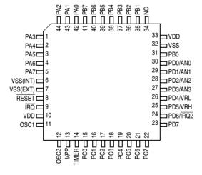
Figure 2-6 Pin Assignment for 44-pin QFP
