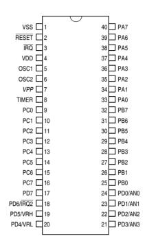
Figure 2-4 Pin Assignment for 40-pin PDIP
