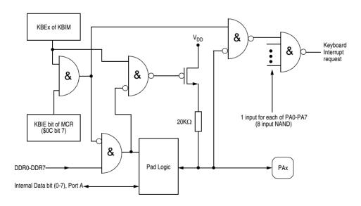
Figure 5-4 Keyboard Interrupt Circuitry
