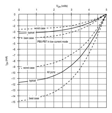
Figure 3-3 Typical  $I_{OH}$  vs  $V_{OH}$  @ $V_{DD}$ =5V
