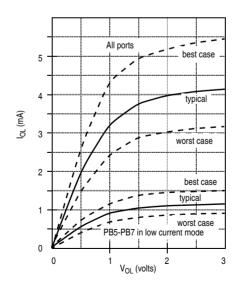
Figure 3-4 Typical  $I_{OL}$  vs  $V_{OL}$  @ $V_{DD}$ =3V
