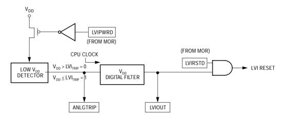
Figure 1. LVI module block diagram
