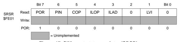
Figure 17. SIM reset status register (SRSR)
