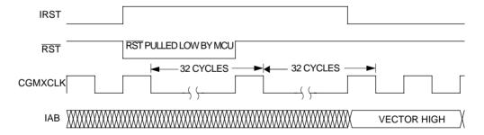
Figure 4. Internal reset timing
