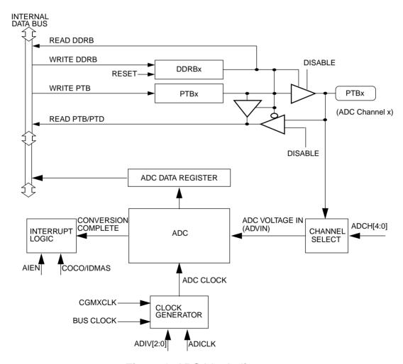
Figure 1. ADC block diagram
