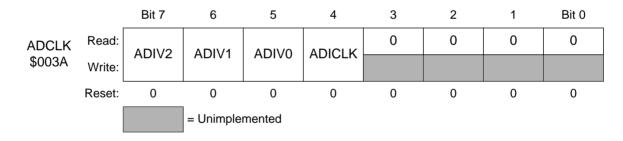
Figure 4. ADC clock register
