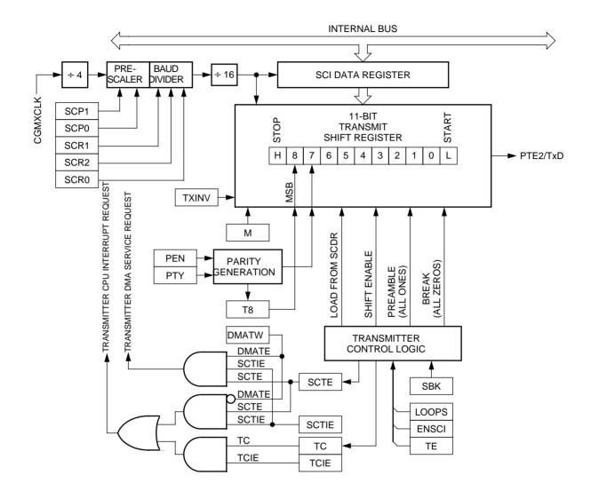
Figure 2. SCI transmitter
