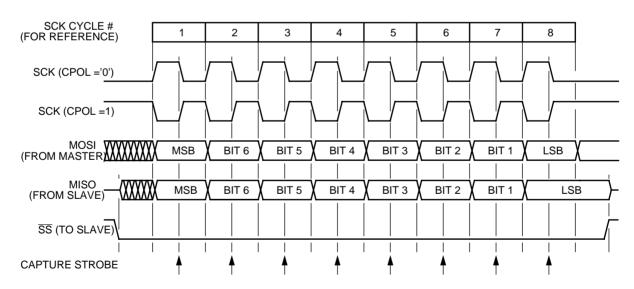
Figure 6. Transmission format (CPHA = '1')
