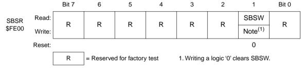
Figure 16. SIM break status register (SBSR)
