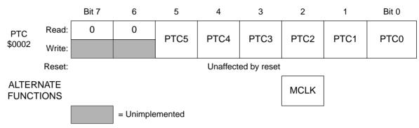
Figure 7. Port C data register (PTC)
