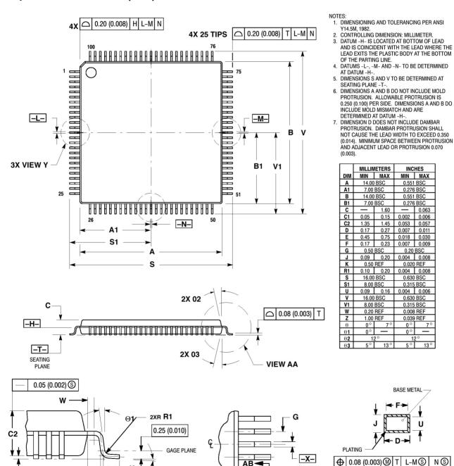
Figure 7. 100-pin QFP
