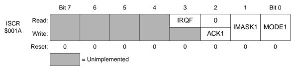
Figure 5. IRQ status and control register (ISCR)
