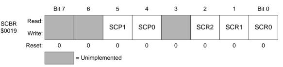
Figure 12. SCI Baud Rate Register (SCBR)
