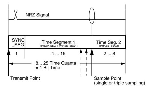
Figure 8. Segments within the bit time
