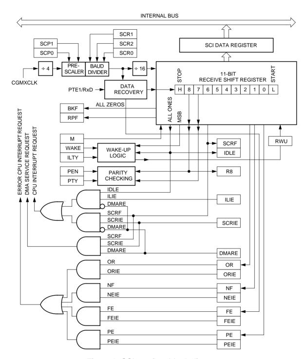
Figure 3. SCI receiver block diagram
