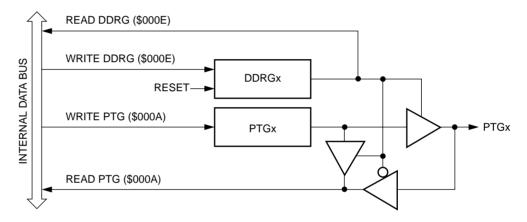
Figure 21. Port G I/O circuit
