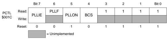
Figure 5. PLL control register (PCTL)
