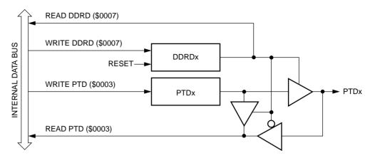
Figure 12. Port D I/O circuit
