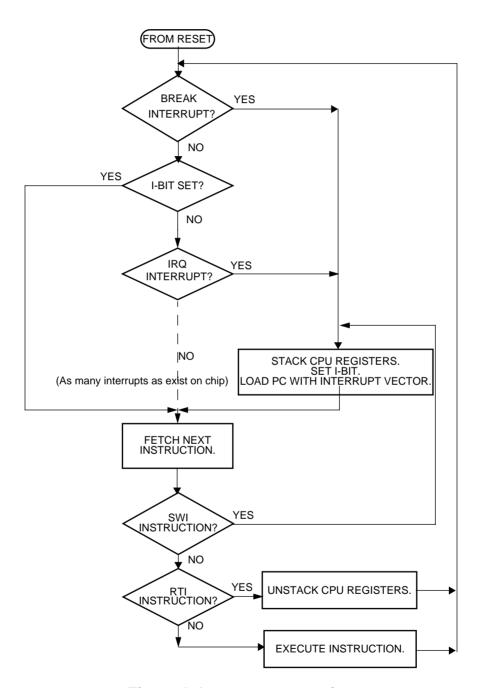
Figure 8. Interrupt processing
