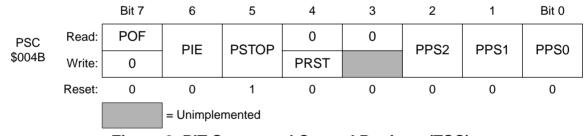
Figure 2. PIT Status and Control Register (TSC)
