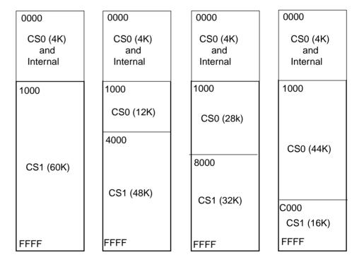
Figure 7 Software controlled chip-select combinations
