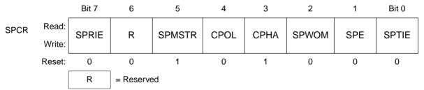
Figure 13. SPI control register (SPCR)
