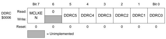
Figure 8. Data direction register C (DDRC)
