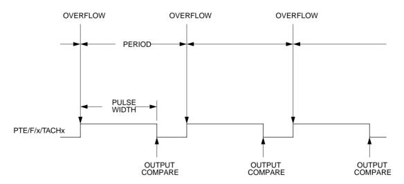
Figure 2. PWM period and pulse width
