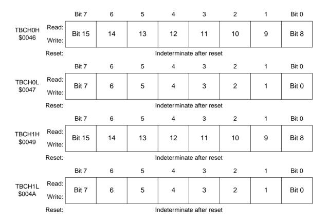
Figure 16. TIMB channel registers (TBCH0H/L-TBCH1H/L)
