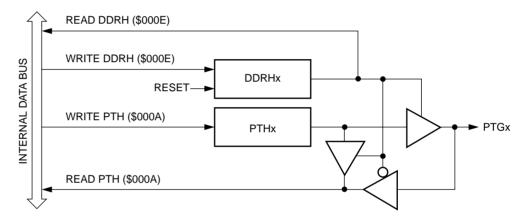
Figure 24. Port H I/O circuit
