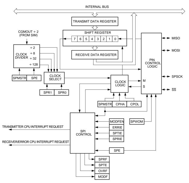
Figure 2. SPI module block diagram
