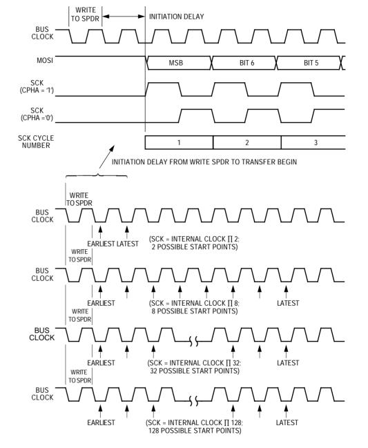
Figure 7. Transmission start delay (master)
