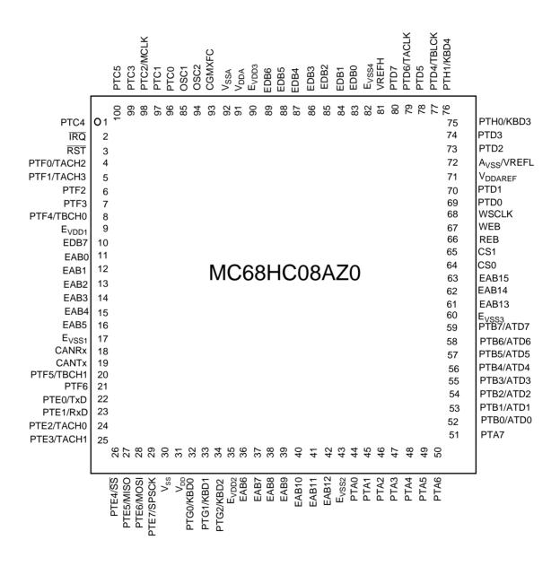
Figure 2. 100 QFP pin assignments
