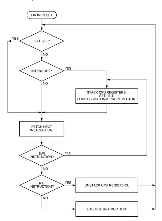
Figure 4. IRQ interrupt flowchart
