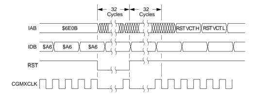
Figure 13. WAIT recovery from internal reset
