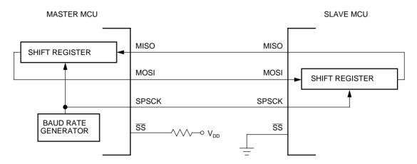
Figure 3. Full-duplex master-slave connections
