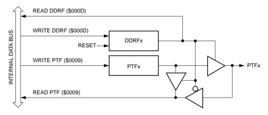
Figure 18. Port F I/O circuit
