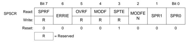
Figure 14. SPI status and control register (SPSCR)
