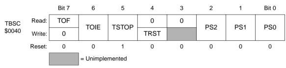
Figure 11. TIMB status and control register (TBSC)
