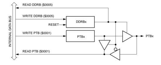
Figure 6. Port B I/O circuit
