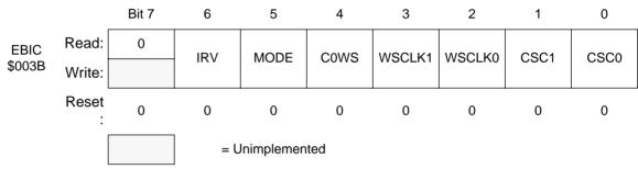
Figure 11 EBI control register (EBIC)
