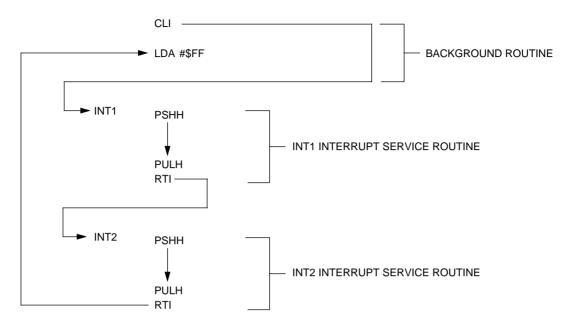
Figure 10. Interrupt recognition example
