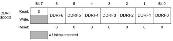
Figure 17. Data direction register F (DDRF)
