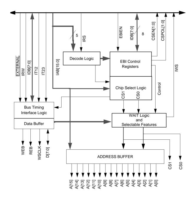
Figure 6 EBI Block Diagram
