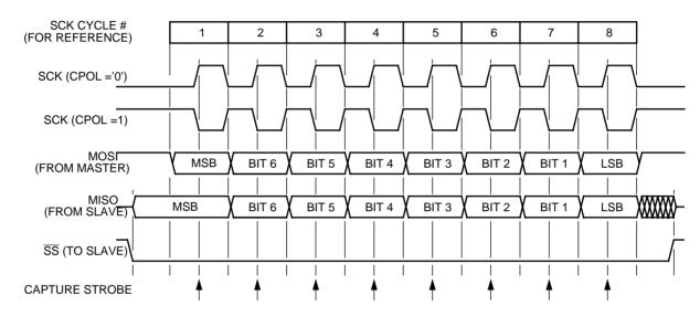
Figure 4. Transmission format (CPHA = '0')
