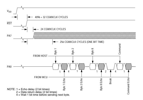
Figure 6. Monitor mode entry timing
