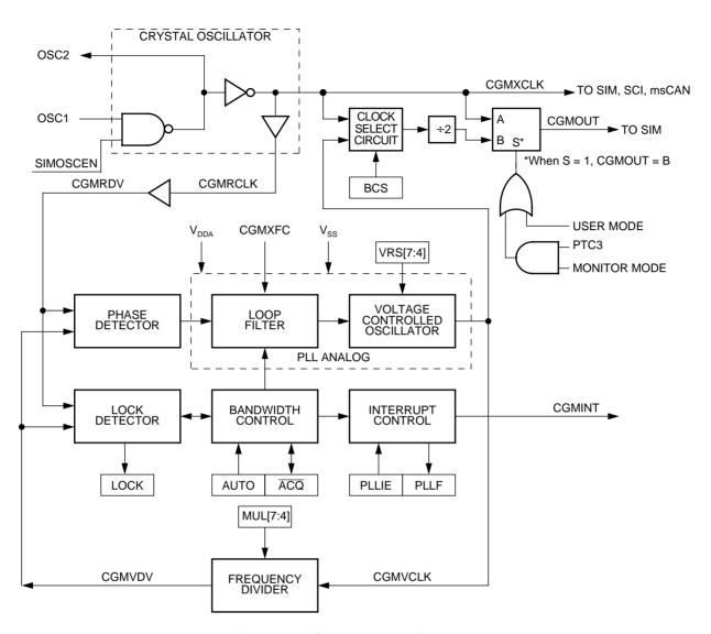
Figure 1. CGM block diagram
