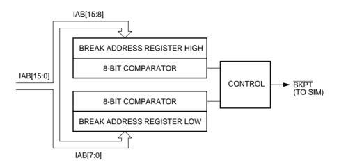
Figure 11. Break module block diagram
