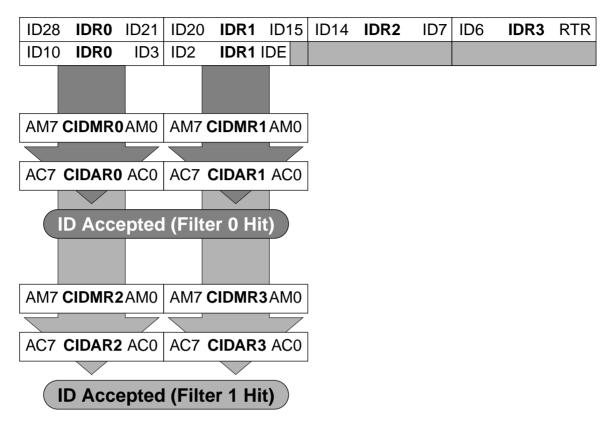
Figure 4. Dual 16-bit maskable acceptance filters
