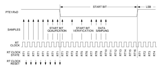
Figure 4. Receiver data sampling
