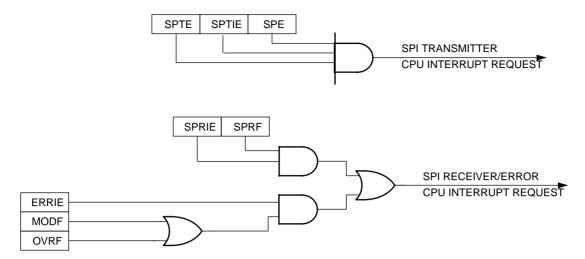
Figure 10. SPI interrupt request generation
