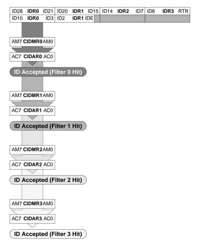
Figure 5. Quadruple 8-bit maskable acceptance filters
