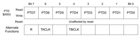
Figure 10. Port D data register (PTD)
