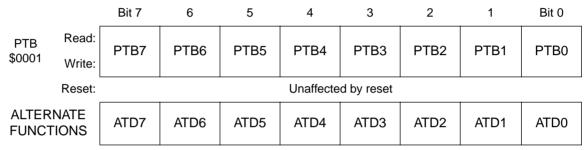
Figure 4. Port B data register (PTB)
