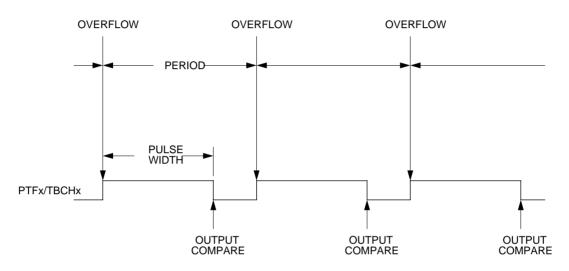
Figure 10. PWM period and pulse width
