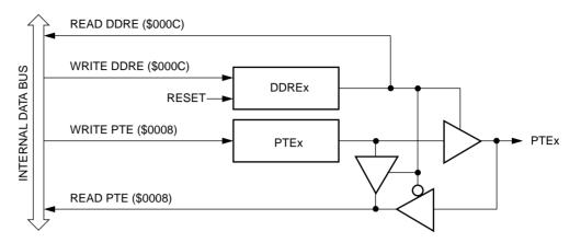
Figure 15. Port E I/O circuit
