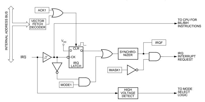
Figure 3. IRQ module block diagram
