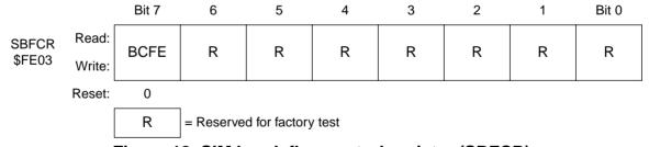
Figure 18. SIM break flag control register (SBFCR)
