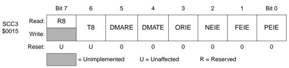
Figure 7. SCI control register 3 (SCC3)
