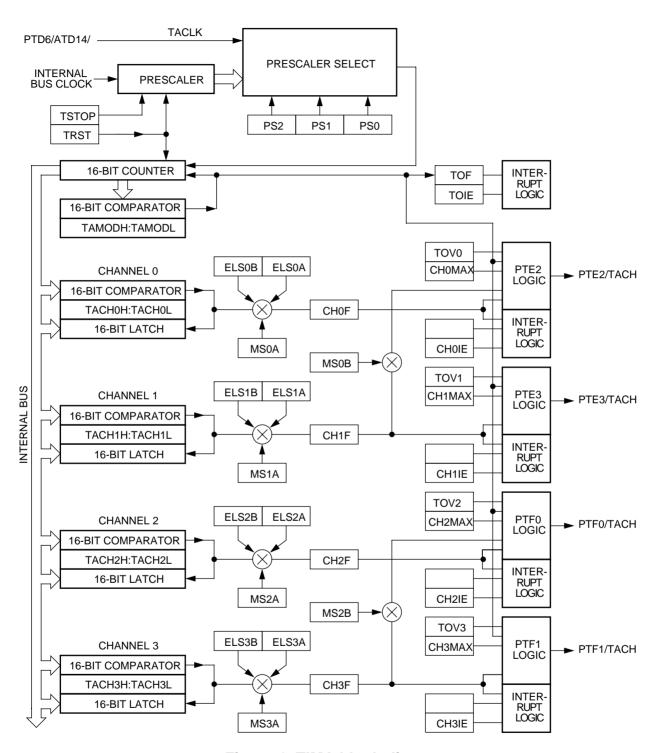
Figure 1. TIMA block diagram
