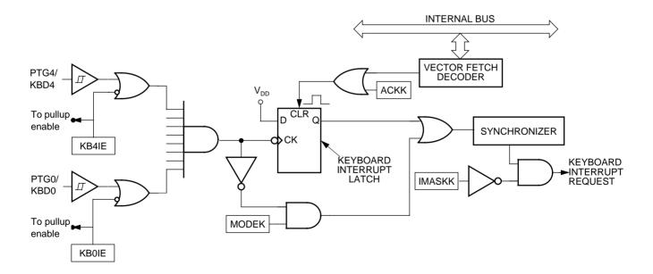
Figure 5. Keyboard module block diagram
