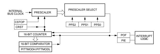
Figure 1. PIT Block Diagram
