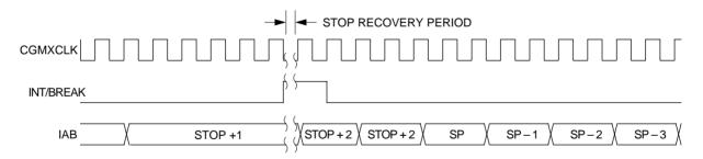
Figure 15. STOP mode recovery from interrupt or break
