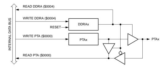
Figure 3. Port A I/O Circuit
