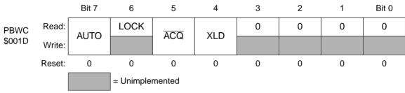
Figure 7. PLL bandwidth control register (PBWC)
