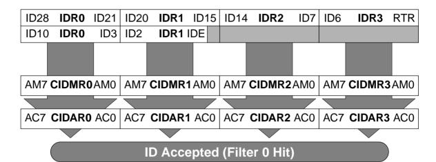
Figure 3. Single 32-bit maskable identifier acceptance filter
