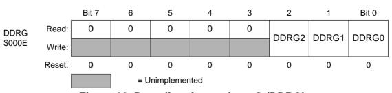
Figure 20. Data direction register G (DDRG)
