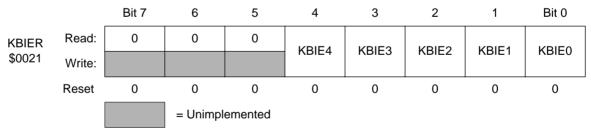
Figure 7. Keyboard interrupt enable register (KBIER)
