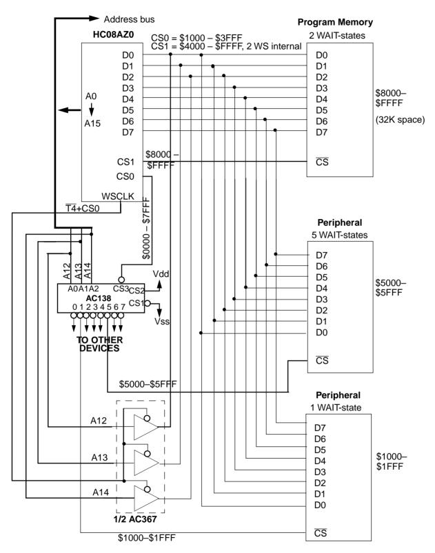
Figure 10 WAIT state selection for multiple I/O peripherals
