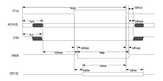
Figure 4 High performance write timings
