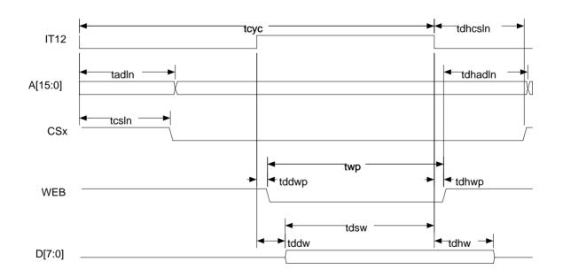
Figure 6 Low-noise mode write timings
