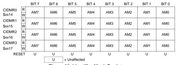
Figure 26. Identifier Mask Registers
