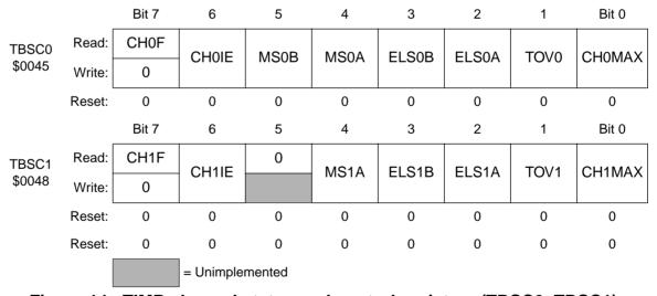
Figure 14. TIMB channel status and control registers (TBSC0-TBSC1)
