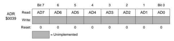
Figure 3. ADC data register
