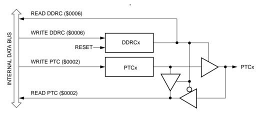
Figure 9. Port C I/O circuit
