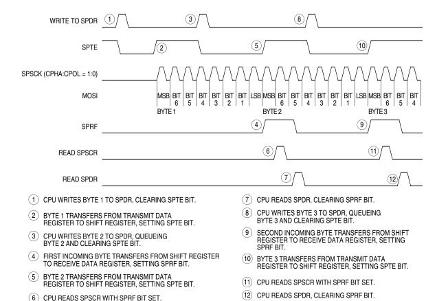
Figure 16-10. SPRF/SPTE CPU Interrupt Timing
