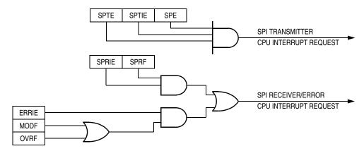
Figure 16-9. SPI Interrupt Request Generation
