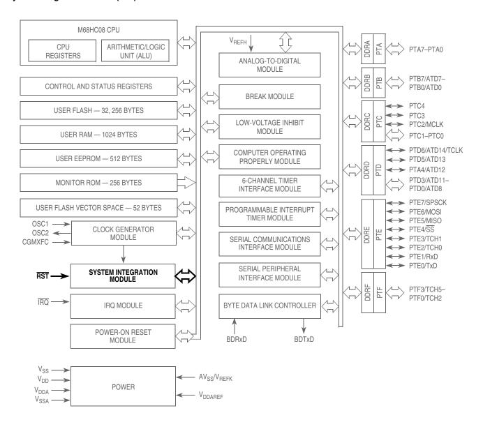
Figure 15-1. Block Diagram Highlighting SIM Block and Pins
