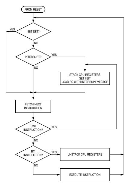
Figure 10-3. IRQ Interrupt Flowchart
