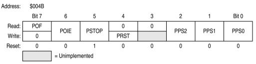
Figure 12-2. PIT Status and Control Register (PSC)
