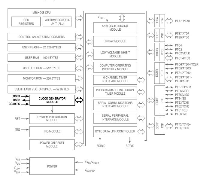
Figure 5-1. Block Diagram Highlighting CGM Block and Pins
