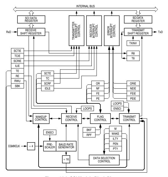
Figure 14-2. SCI Module Block Diagram
