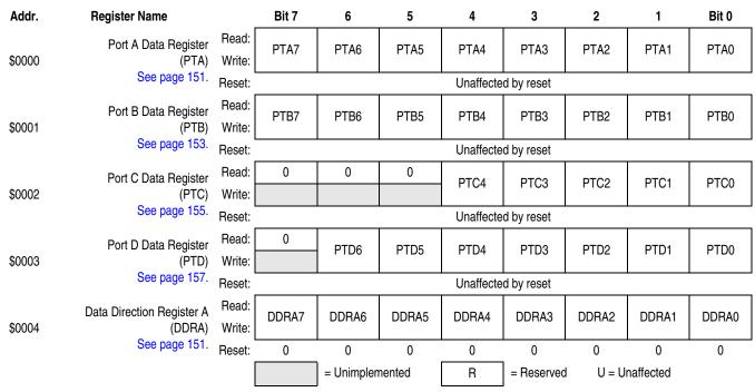
Figure 2-2. I/O Data, Status and Control Registers (Sheet 1 of 6)
