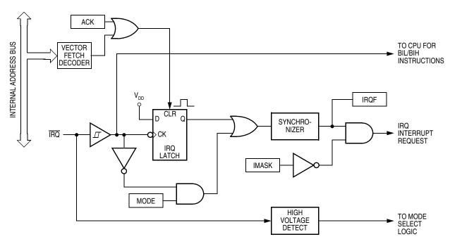
Figure 10-2. IRQ Block Diagram
