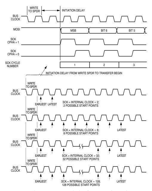
Figure 16-6. Transmission Start Delay (Master)
