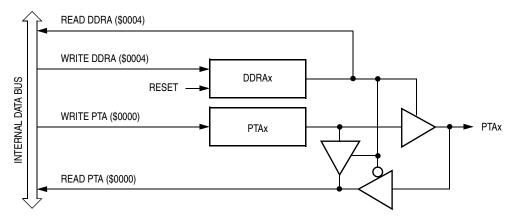
Figure 13-3. Port A I/O Circuit
