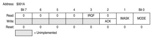
Figure 10-4. IRQ Status and Control Register (ISCR)
