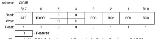
Figure 4-16. BDLC Analog and Roundtrip Delay Register (BARD)
