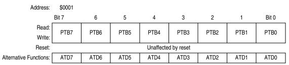
Figure 13-4. Port B Data Register (PTB)
