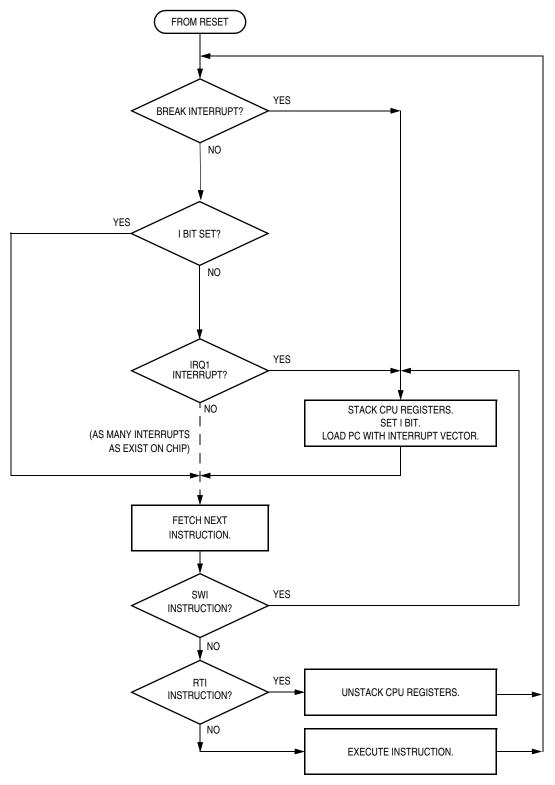
Figure 15-9. Interrupt Processing
