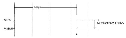
Figure 4-11. J1850 VPW Received BREAK Symbol Times
