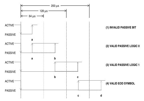
Figure 4-8. J1850 VPW Received Passive Symbol Times
