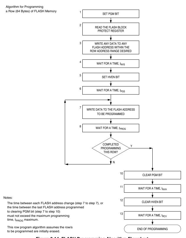
Figure 2-14. FLASH Programming Algorithm Flowchart
