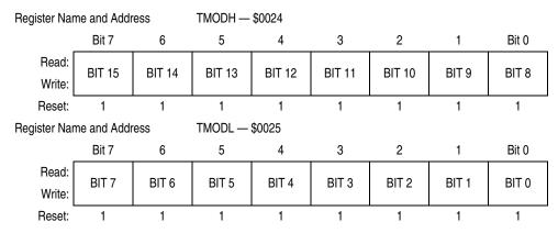
Figure 17-6. TIM Counter Modulo Registers (TMODH and TMODL)
