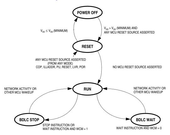
Figure 4-3. BDLC Operating Modes State Diagram
