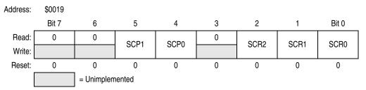
Figure 14-16. SCI Baud Rate Register (SCBR)
