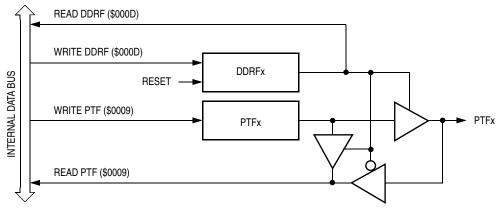
Figure 13-18. Port F I/O Circuit
