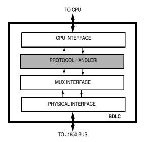
Figure 4-13. BDLC Block Diagram
