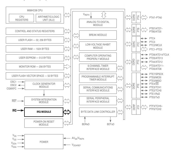
Figure 10-1. Block Diagram Highlighting IRQ Block and Pins
