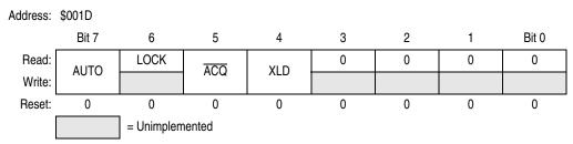
Figure 5-5. PLL Bandwidth Control Register (PBWC)
