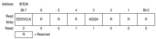
Figure 7-1. Configuration Register (CONFIG2)
