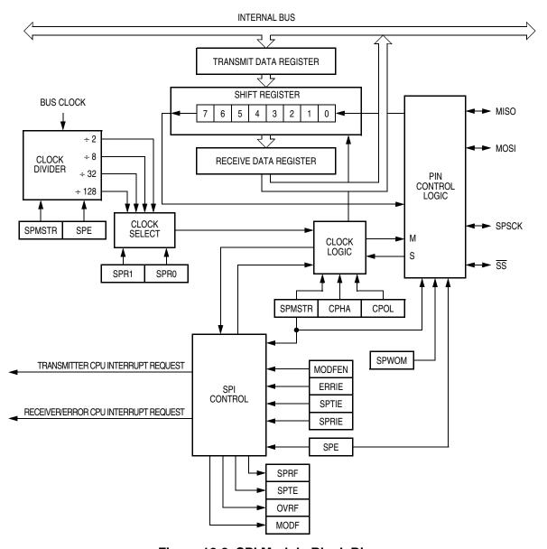
Figure 16-2. SPI Module Block Diagram
