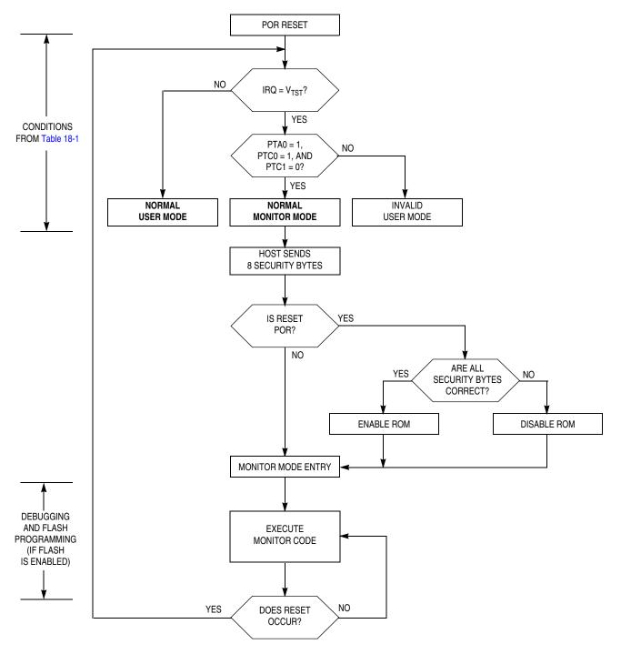
Figure 18-5. Simplified Monitor Mode Entry Flowchart
