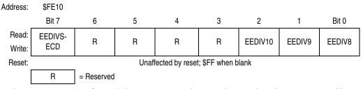
Figure 2-9. EEPROM Divider Nonvolatile Register High (EEDIVHNVR))
