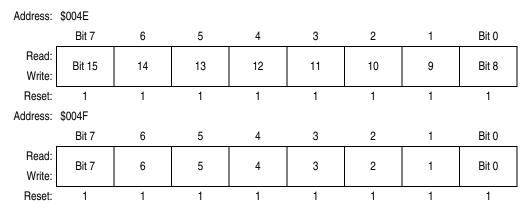
Figure 12-4. PIT Counter Modulo Registers (PMODH-PMODL)
