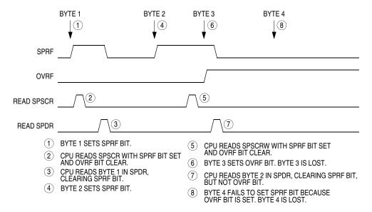
Figure 16-7. Missed Read of Overflow Condition
