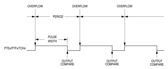
Figure 17-3. PWM Period and Pulse Width
