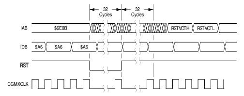
Figure 15-14. Wait Recovery from Internal Reset
