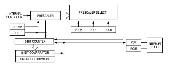
Figure 12-1. PIT Block Diagram
