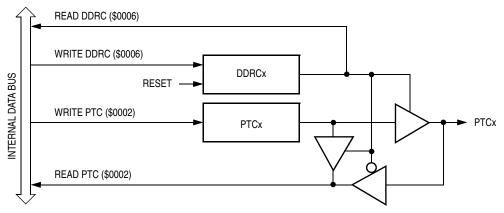
Figure 13-9. Port C I/O Circuit
