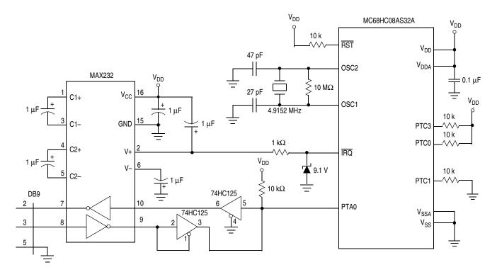
Figure 18-6. Normal Monitor Mode Circuit
