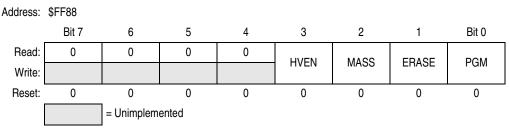
Figure 2-11. FLASH Control Register (FLCR)
