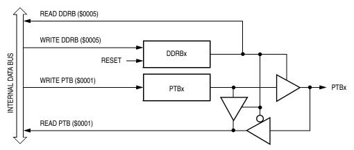
Figure 13-6. Port B I/O Circuit
