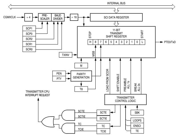
Figure 14-4. SCI Transmitter
