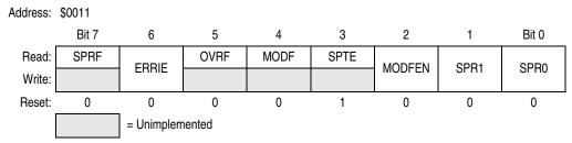
Figure 16-13. SPI Status and Control Register (SPSCR)
