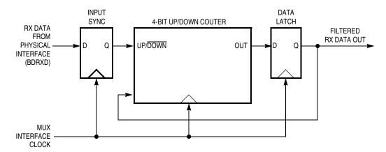
Figure 4-5. BDLC Rx Digital Filter Block Diagram
