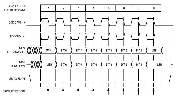
Figure 16-5. Transmission Format (CPHA = 1)
