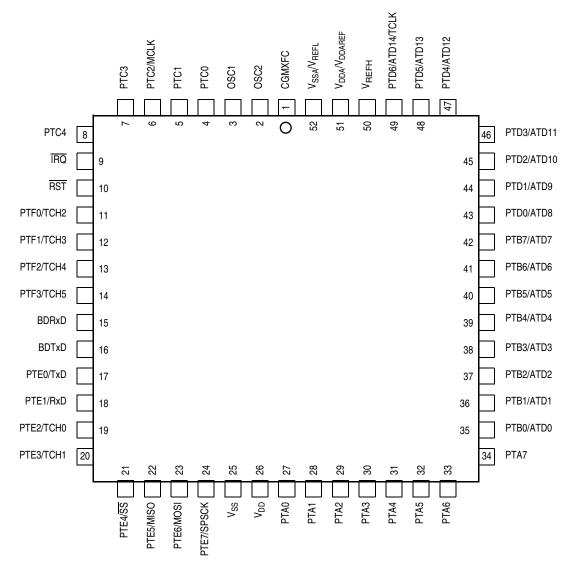
Figure 1-2. 52-Pin PLCC Assignments (Top View)
