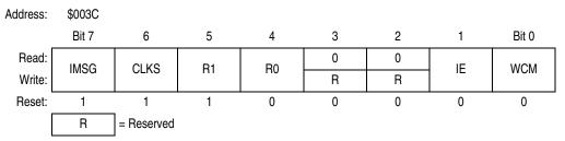
Figure 4-17. BDLC Control Register 1 (BCR1)
