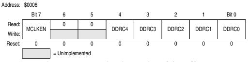
Figure 13-8. Data Direction Register C (DDRC)
