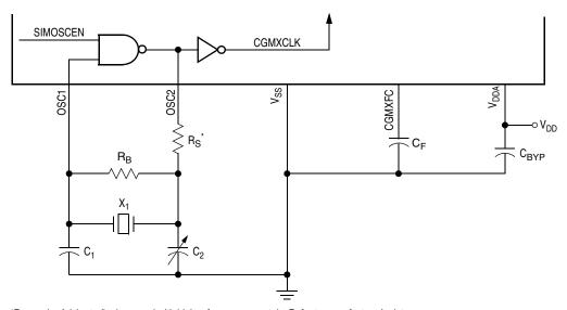
${}^{\star}R_{S}$  can be 0 (shorted) when used with higher-frequency crystals. Refer to manufacturer's data.
