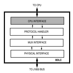
Figure 4-15. BDLC Block Diagram
