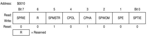
Figure 16-12. SPI Control Register (SPCR)
