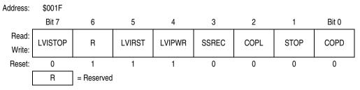
Figure 6-1. Configuration Register (CONFIG1)
