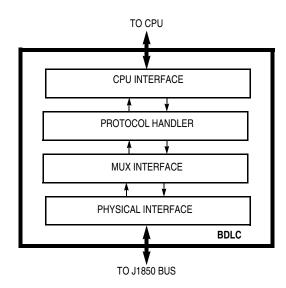
Figure 4-2. BDLC Block Diagram
