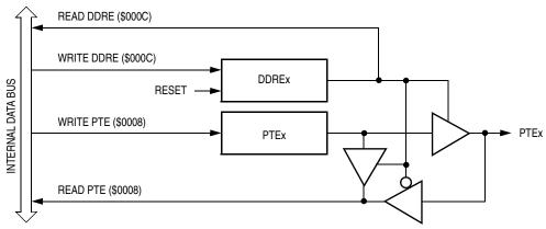
Figure 13-15. Port E I/O Circuit
