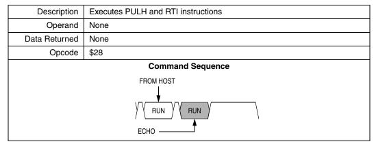
The MCU executes the SWI and PSHH instructions when it enters monitor mode. The RUN command tells the MCU to execute the PULH and RTI instructions. Before sending the RUN command, the host can
