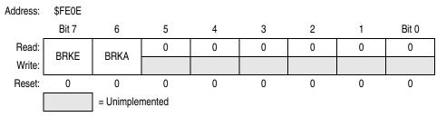
Figure 18-3. Break Status and Control Register (BSCR)
