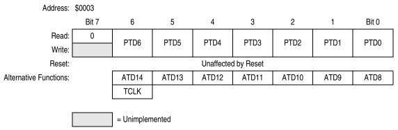
Figure 13-10. Port D Data Register (PTD)
