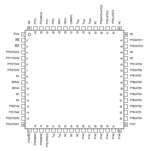
Figure 1-3. 64-Pin QFP Assignments (Top View)
