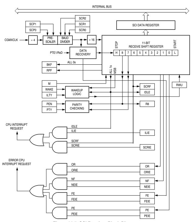
Figure 14-5. SCI Receiver Block Diagram
