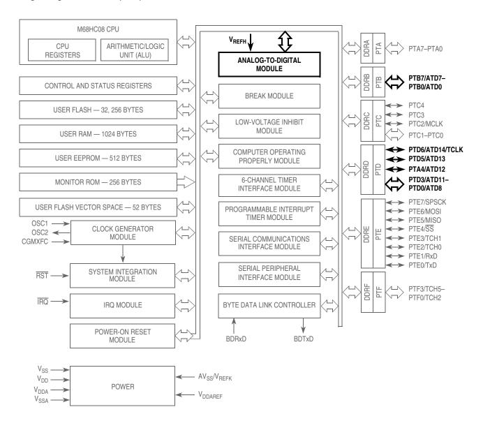
Figure 3-1. Block Diagram Highlighting ADC Block and Pins
