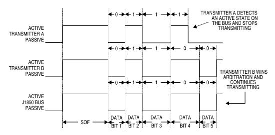
Figure 4-12. J1850 VPW Bitwise Arbitrations
