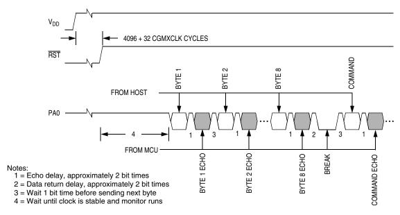
Figure 18-13. Monitor Mode Entry Timing
