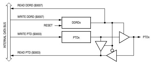
Figure 13-12. Port D I/O Circuit
