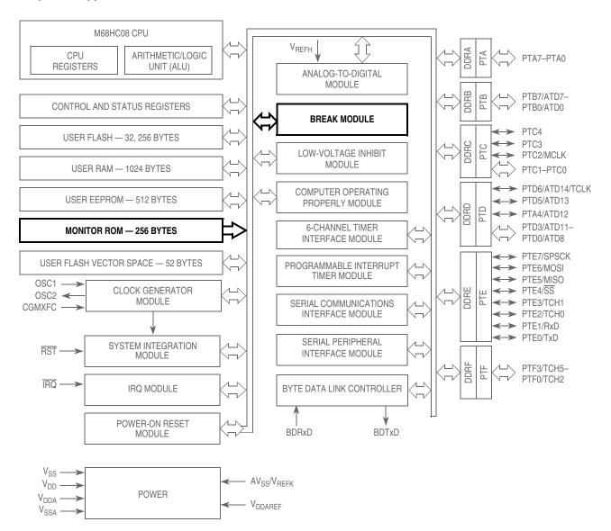
Figure 18-1. Block Diagram Highlighting BRK and MON Blocks
