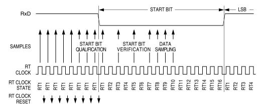
Figure 14-6. Receiver Data Sampling
