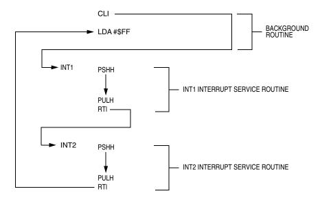
Figure 15-11. Interrupt Recognition Example
