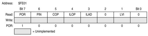
Figure 15-18. SIM Reset Status Register (SRSR)
