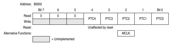
Figure 13-7. Port C Data Register (PTC)
