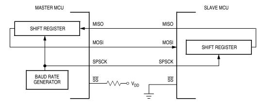
Figure 16-3. Full-Duplex Master-Slave Connections
