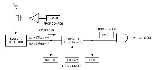
Figure 11-1. LVI Module Block Diagram
