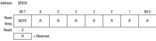
Figure 15-19. SIM Break Flag Control Register (SBFCR)
