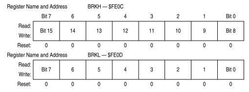
Figure 18-4. Break Address Registers (BRKH and BRKL)
