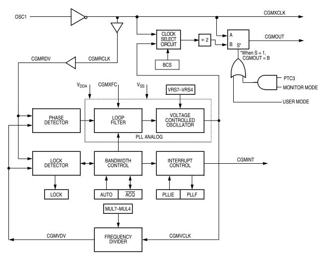
Figure 5-2. CGM Block Diagram
