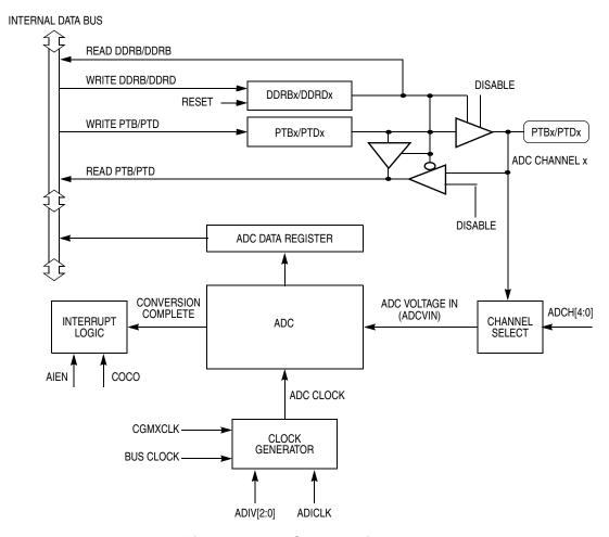
Figure 3-2. ADC Block Diagram
