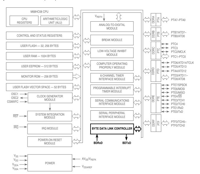
Figure 4-1. Block Diagram Highlighting BDLC Block and Pins
