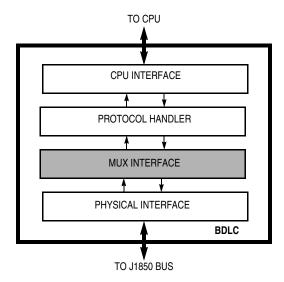
Figure 4-4. BDLC Block Diagram
