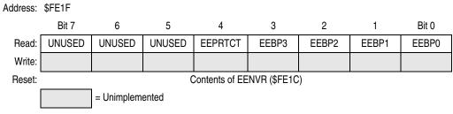
Figure 2-5. EEPROM Array Configuration Register (EEACR)
