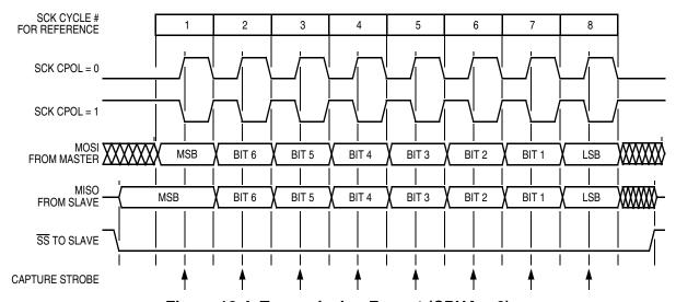
Figure 16-4. Transmission Format (CPHA = 0)
