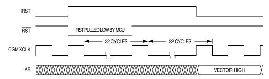
Figure 15-5. Internal Reset Timing
