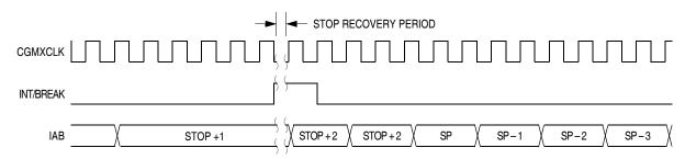
Figure 14-19. Stop Mode Recovery from Interrupt
