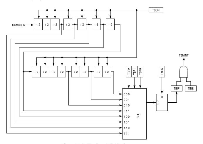
Figure 16-1. Timebase Block Diagram
