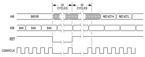
Figure 14-17. Wait Recovery from Internal Reset
