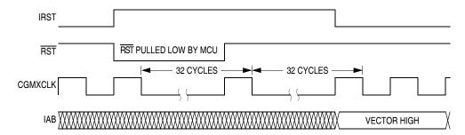
Figure 14-5. Internal Reset Timing
