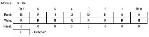
Figure 14-12. Interrupt Status Register 1 (INT1)
