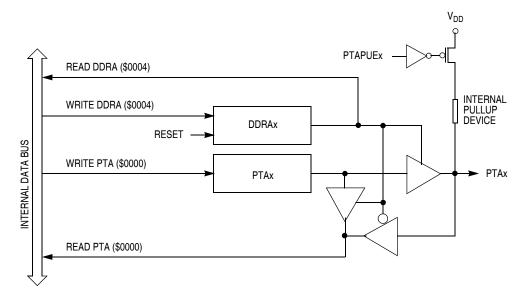
Figure 12-4. Port A I/O Circuit
