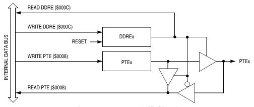
Figure 12-19. Port E I/O Circuit
