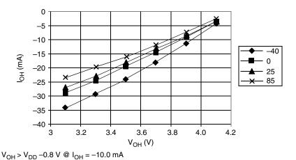
Figure 19-3. Typical High-Side Driver Characteristics — Port PTC1–PTC0 (V<sub>DD</sub> = 4.5 Vdc)
