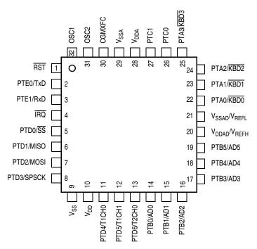
Figure 1-2. 32-Pin LQFP Pin Assignments
