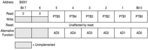
Figure 12-6. Port B Data Register (PTB)
