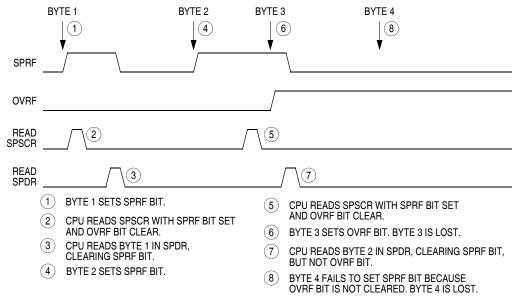
Figure 15-10. Missed Read of Overflow Condition
