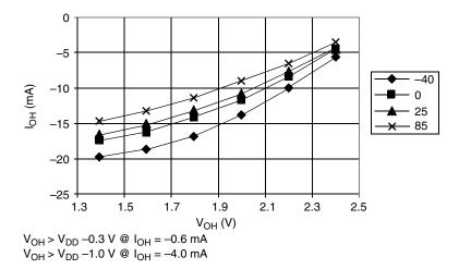
Figure 19-6. Typical High-Side Driver Characteristics — Ports PTB5–PTB0, PTD6–PTD0, and PTE1–PTE0 (V<sub>DD</sub> = 2.7 Vdc)
