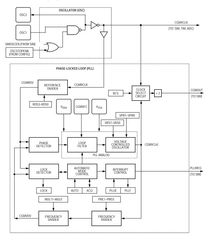
Figure 4-1. CGM Block Diagram
