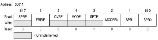
Figure 15-15. SPI Status and Control Register (SPSCR)
