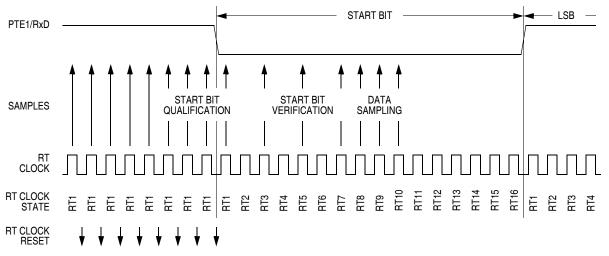
Figure 13-7. Receiver Data Sampling
