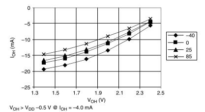
Figure 19-4. Typical High-Side Driver Characteristics — Port PTC1–PTC0 (V<sub>DD</sub> = 2.7 Vdc)
