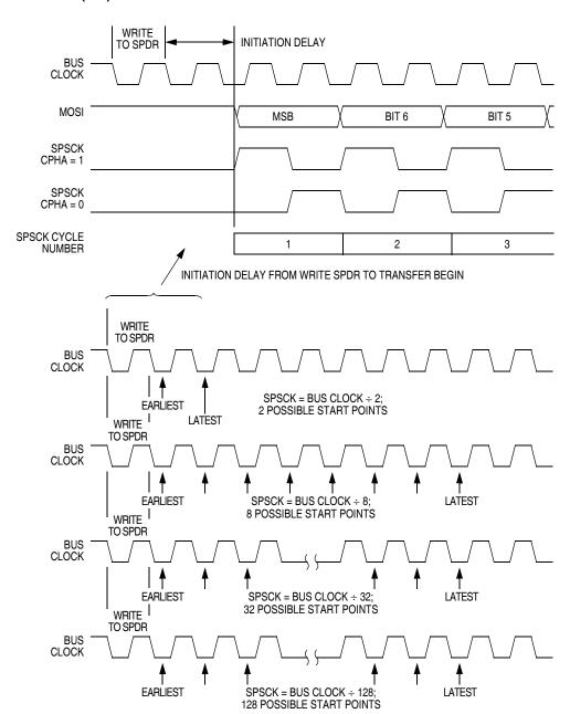
Figure 15-8. Transmission Start Delay (Master)
