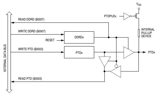
Figure 12-15. Port D I/O Circuit
