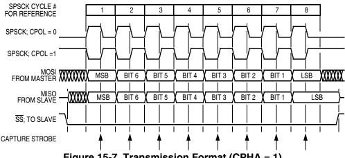
Figure 15-7. Transmission Format (CPHA = 1)
