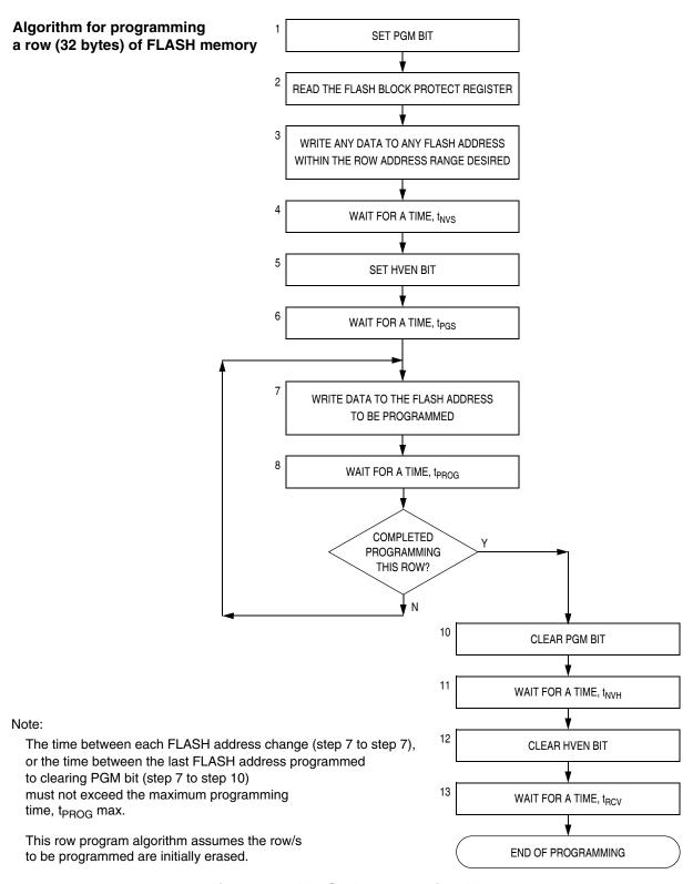
Figure 2-4. FLASH Programming Flowchart
