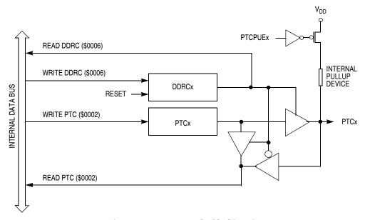
Figure 12-11. Port C I/O Circuit
