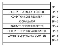
Figure 18-16. Stack Pointer at Monitor Mode Entry
