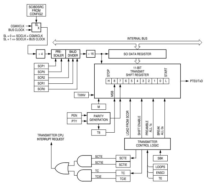
Figure 13-5. SCI Transmitter
