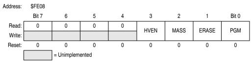
Figure 2-3. FLASH Control Register (FLCR)
