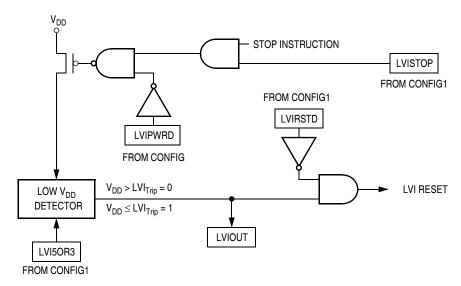
Figure 11-1. LVI Module Block Diagram
