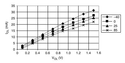
$V_{OL} < 0.4 \ V \ @ \ I_{OL} = 1.6 \ mA$  $V_{OL} < 1.5 \ V \ @ \ I_{OL} = 10.0 \ mA$
