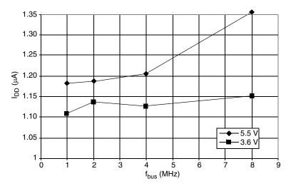
Figure 19-15. Typical Stop Mode I<sub>DD</sub>, with all Modules Disabled (–40  $^{\circ}$ C to 125  $^{\circ}$ C)
