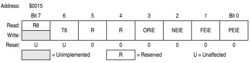
Figure 13-12. SCI Control Register 3 (SCC3)
