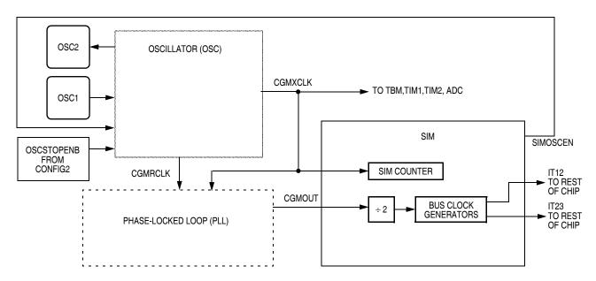
Figure 14-3. System Clock Signals
