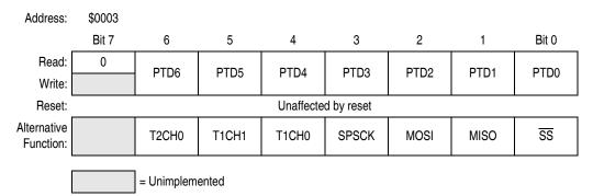
Figure 12-13. Port D Data Register (PTD)
