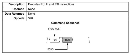
The MCU executes the SWI and PSHH instructions when it enters monitor mode. The RUN command tells the MCU to execute the PULH and RTI instructions. Before sending the RUN command, the host can modify the stacked CPU registers to prepare to run the host program. The READSP command returns the incremented stack pointer value, SP + 1. The high and low bytes of the program counter are at addresses SP + 5 and SP + 6.
