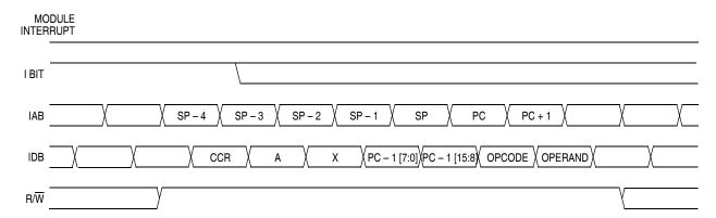
Figure 14-9. Interrupt Recovery Timing
