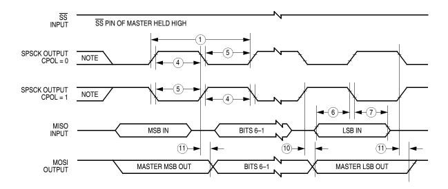
Note: This first clock edge is generated internally, but is not seen at the SPSCK pin.
