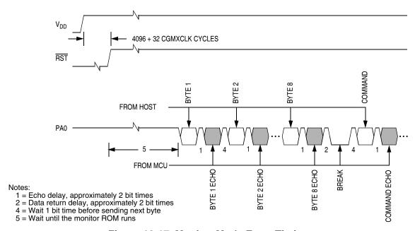
Figure 18-17. Monitor Mode Entry Timing
