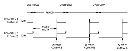
Figure 17-4. PWM Period and Pulse Width
