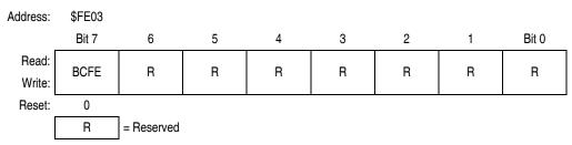
Figure 14-22. SIM Break Flag Control Register (BFCR)
