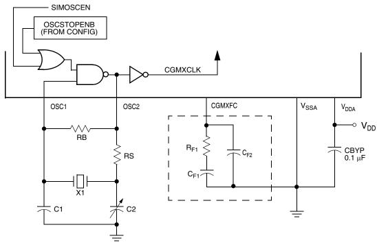
Note: Filter network in box can be replaced with C<sub>F</sub> but will degrade stability.
