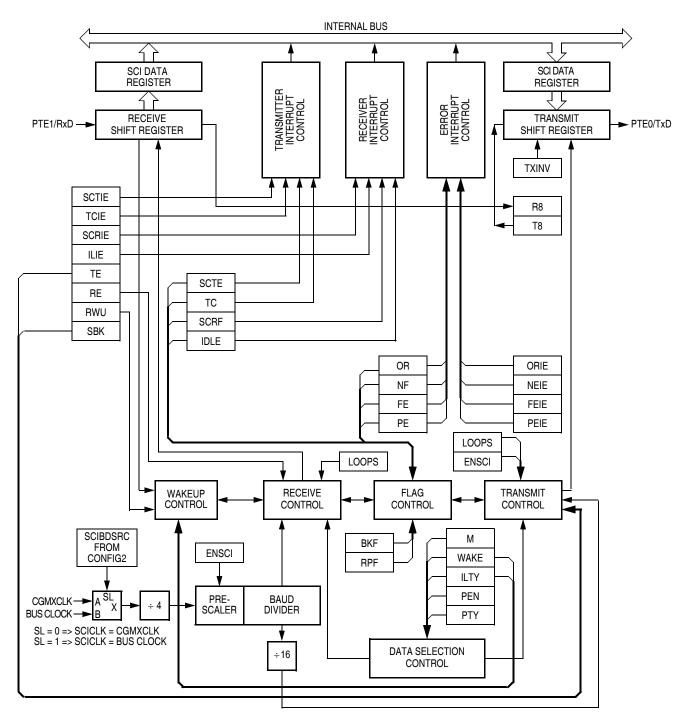
Figure 13-3. SCI Module Block Diagram
