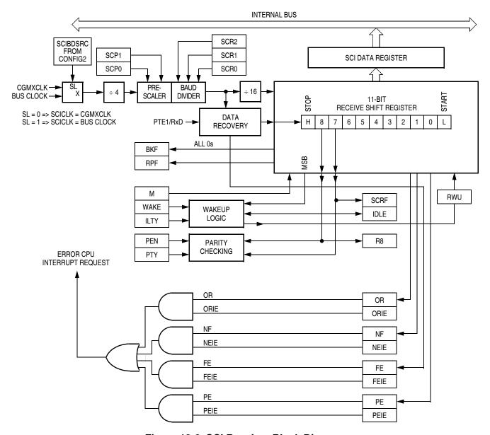
Figure 13-6. SCI Receiver Block Diagram
