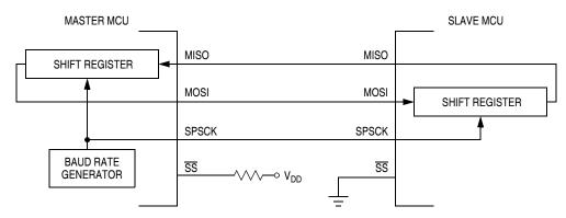
Figure 15-4. Full-Duplex Master-Slave Connections
