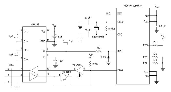
Figure 18-10. Normal Monitor Mode Circuit
