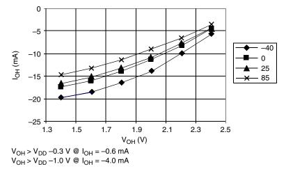
Figure 19-2. Typical High-Side Driver Characteristics — Port PTA3–PTA0 (V<sub>DD</sub> = 2.7 Vdc)
