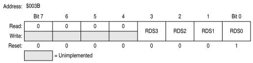
Figure 4-9. PLL Reference Divider Select Register (PMDS)
