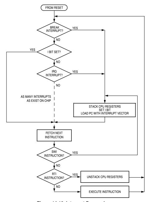
Figure 14-10. Interrupt Processing
