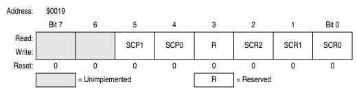
Figure 13-17. SCI Baud Rate Register (SCBR)
