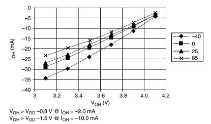
Figure 19-1. Typical High-Side Driver Characteristics — Port PTA3-PTA0 (V<sub>DD</sub> = 4.5 Vdc)
