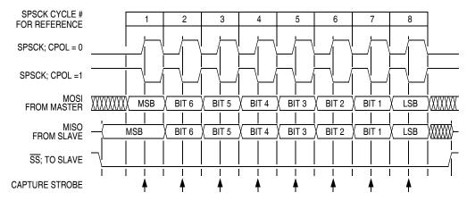
Figure 15-5. Transmission Format (CPHA = 0)
