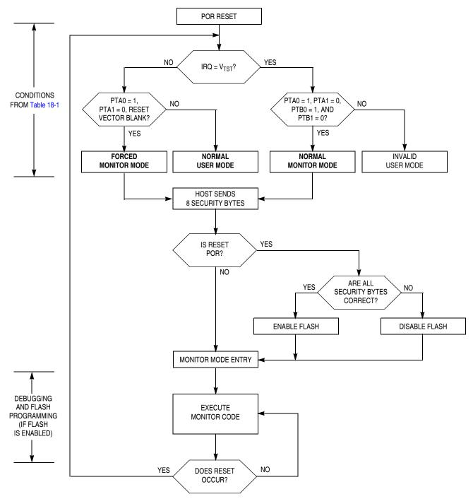
Figure 18-9. Simplified Monitor Mode Entry Flowchart
