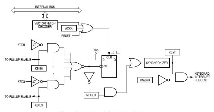
Figure 9-2. Keyboard Module Block Diagram
