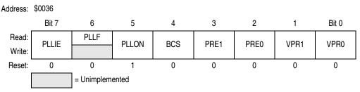
Figure 4-4. PLL Control Register (PCTL)
