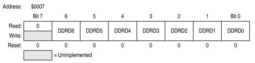
Figure 12-14. Data Direction Register D (DDRD)
