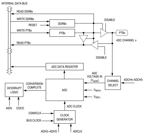
Figure 3-2. ADC Block Diagram
