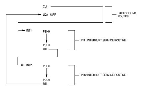
Figure 14-11. Interrupt Recognition Example
