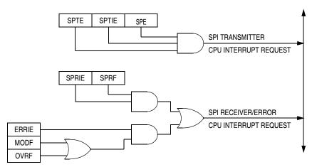
Figure 15-12. SPI Interrupt Request Generation
