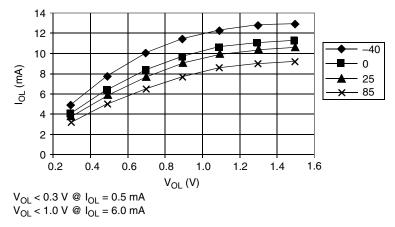
Figure 19-8. Typical Low-Side Driver Characteristics — Port PTA3–PTA0 (V<sub>DD</sub> = 2.7 Vdc)
