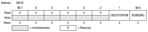
Figure 5-1. Configuration Register 2 (CONFIG2)
