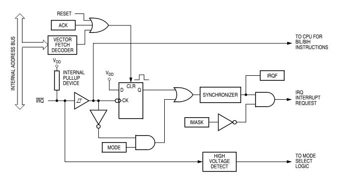
Figure 8-1. IRQ Module Block Diagram
