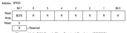
Figure 18-8. SIM Break Flag Control Register (SBFCR)
