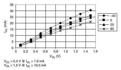
Figure 19-7. Typical Low-Side Driver Characteristics — Port PTA3–PTA0 (V<sub>DD</sub> = 5.5 Vdc)
