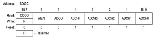
Figure 3-3. ADC Status and Control Register (ADSCR)
