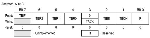
Figure 16-2. Timebase Control Register (TBCR)
