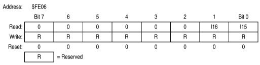
Figure 14-14. Interrupt Status Register 3 (INT3)
