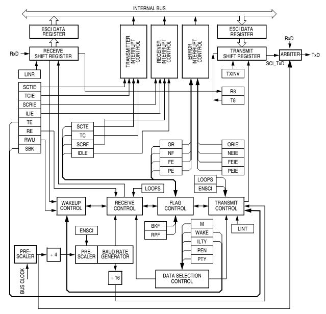
Figure 14-2. ESCI Module Block Diagram
