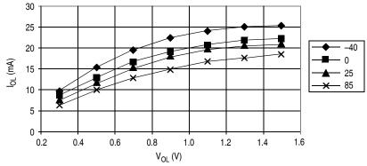
$V_{OL} < 0.8 V @ I_{OL} = 10 mA$
