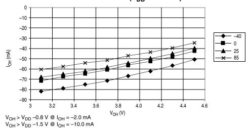
Figure 20-7. Typical High-Side Driver Characteristics – Ports PTB7–PTB0, PTC6–PTC5, PTD7–PTD0, and PTE1–PTE0 (V<sub>DD</sub> = 5.5 Vdc)
