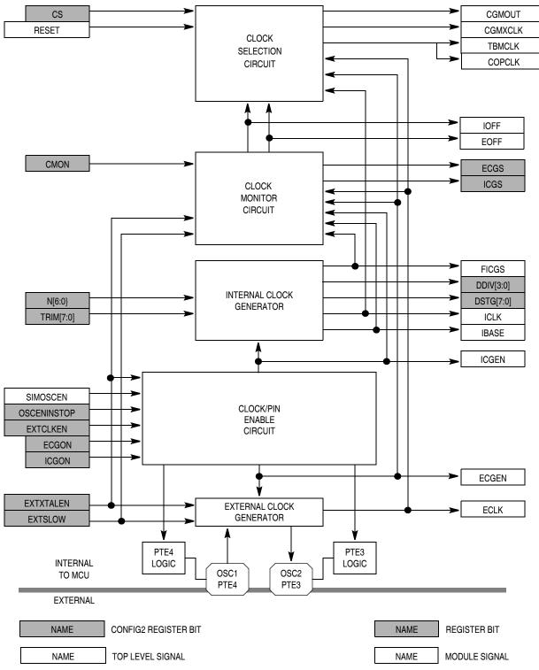
Figure 7-2. ICG Module Block Diagram
