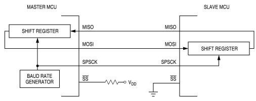
Figure 16-4. Full-Duplex Master-Slave Connections
