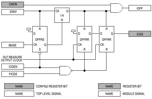
Figure 7-6. Internal Clock Activity Detector
