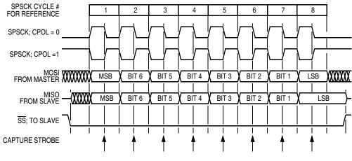
Figure 16-7. Transmission Format (CPHA = 1)
