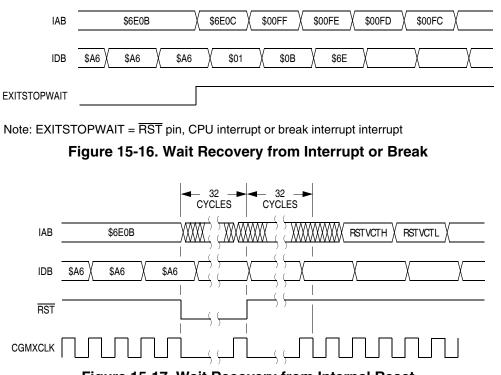
Figure 15-17. Wait Recovery from Internal Reset
