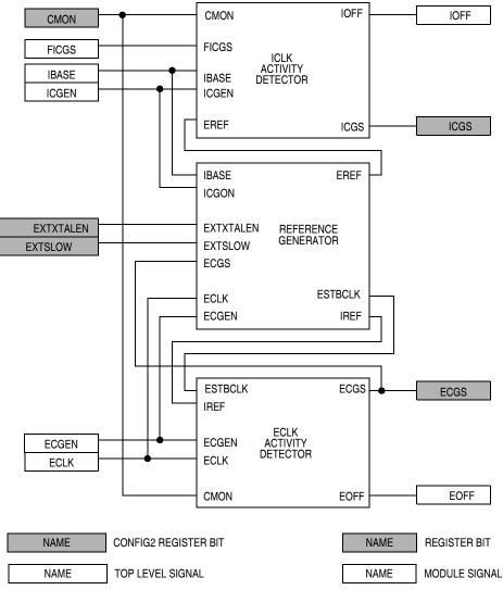
Figure 7-5. Clock Monitor Block Diagram
