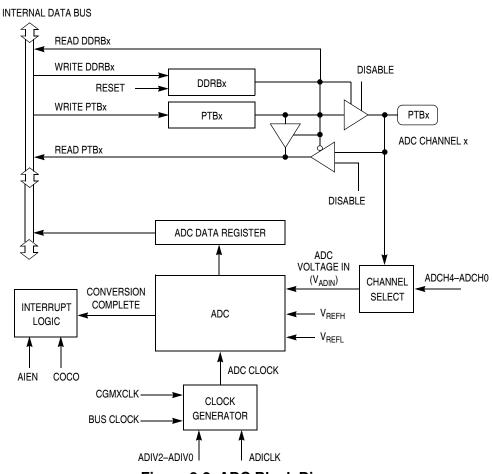
Figure 3-2. ADC Block Diagram
