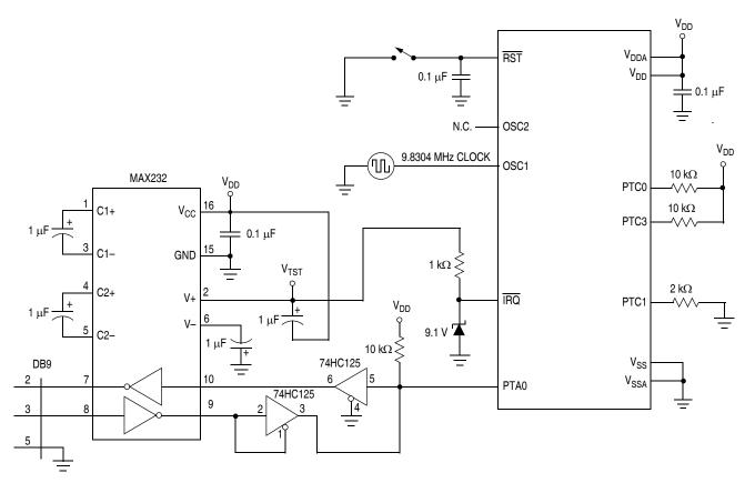
Figure 19-12. Standard Monitor Mode
