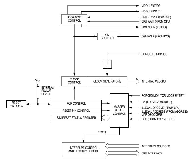
Figure 15-1. SIM Block Diagram
