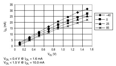
Figure 20-13. Typical Low-Side Driver Characteristics – Ports PTB7–PTB0, PTC6–PTC5, PTD7–PTD0, and PTE1–PTE0 (V<sub>DD</sub> = 5.5 Vdc)
