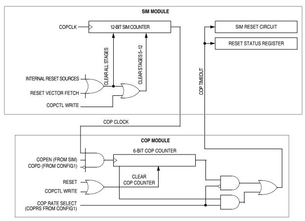
Figure 5-1. COP Block Diagram
