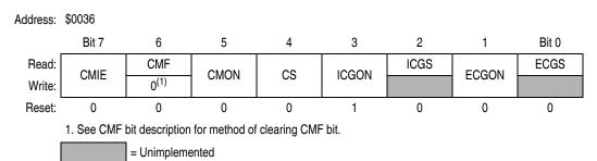
Figure 7-12. ICG Control Register (ICGCR)
