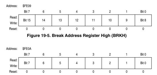
Figure 19-6. Break Address Register Low (BRKL)
