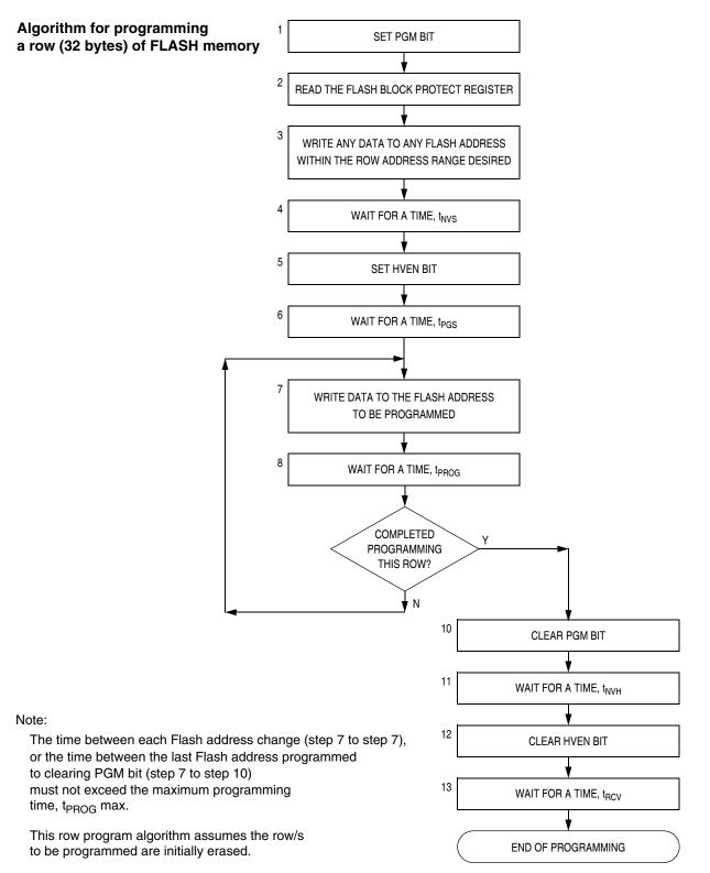
Figure 2-4. Flash Programming Flowchart
