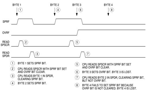
Figure 16-10. Missed Read of Overflow Condition
