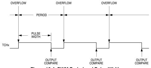
Figure 18-4. PWM Period and Pulse Width
