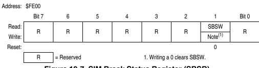
Figure 19-7. SIM Break Status Register (SBSR)
