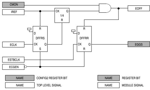
Figure 7-7. External Clock Activity Detector
