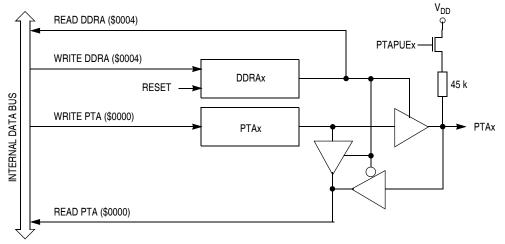
Figure 12-4. Port A I/O Circuit
