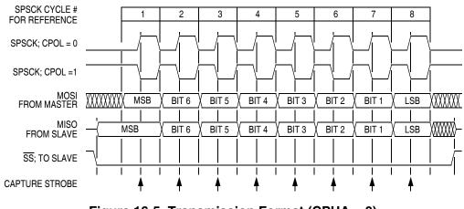
Figure 16-5. Transmission Format (CPHA = 0)
