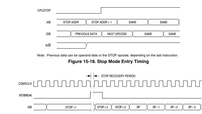
Figure 15-19. Stop Mode Recovery from Interrupt
