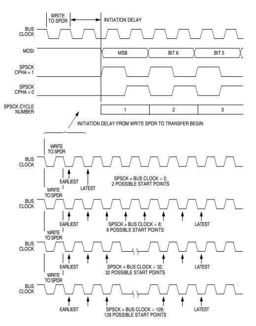
Figure 16-8. Transmission Start Delay (Master)
