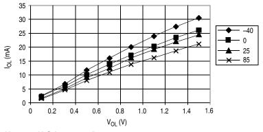
$\begin{array}{l} V_{OL} < 0.4 \ V \ @ \ I_{OL} = 1.6 \ mA \\ V_{OL} < 1.5 \ V \ @ \ I_{OL} = 10.0 \ mA \end{array}$
