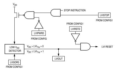
Figure 10-1. LVI Module Block Diagram
