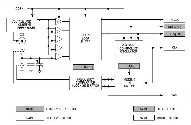
Figure 7-3. Internal Clock Generator Block Diagram
