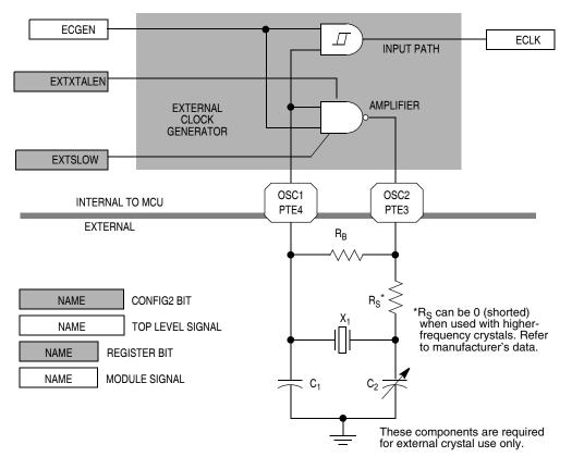
Figure 7-4. External Clock Generator Block Diagram
