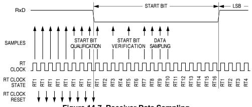
Figure 14-7. Receiver Data Sampling
