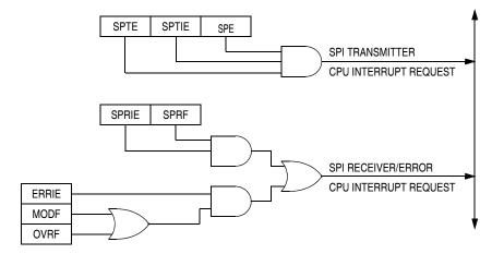
Figure 16-12. SPI Interrupt Request Generation
