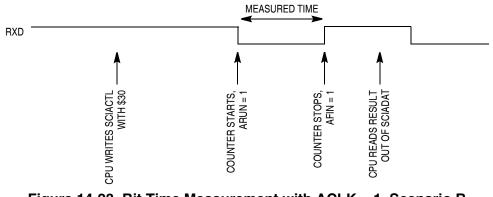
Figure 14-23. Bit Time Measurement with ACLK = 1, Scenario B
