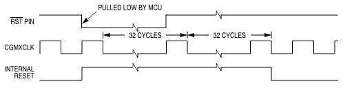
Figure 13-1. Internal Reset Timing
