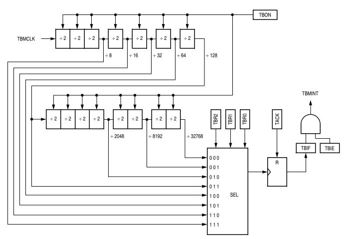
Figure 17-1. Timebase Block Diagram
