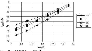
$V_{OH} > V_{DD} - 0.8 V @ I_{OH} = -2.0 mA$  $V_{OH} > V_{DD} - 1.5 V @ I_{OH} = -10.0 mA$
