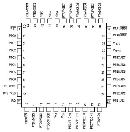
Figure 1-3. 44-Pin QFP Pin Assignments
