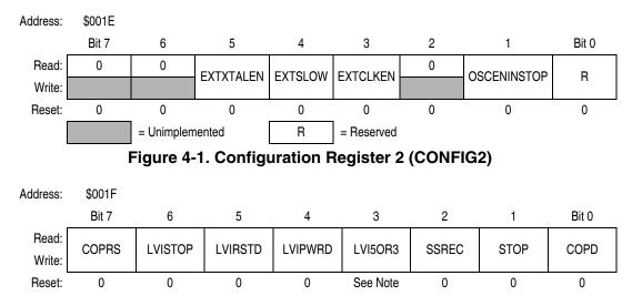
Note: LVI5OR3 bit is only reset via POR (power-on reset)
