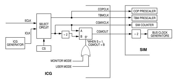
Figure 15-3. System Clock Signals
