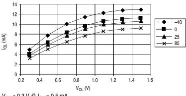
$V_{OL} < 0.3 V @ I_{OL} = 0.5 mA$  $V_{OL} < 1.0 V @ I_{OL} = 6.0 mA$
