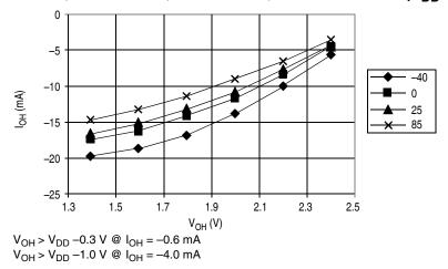
Figure 20-8. Typical High-Side Driver Characteristics – Ports PTB7–PTB0, PTC6–PTC5, PTD7–PTD0, and PTE1–PTE0 (V<sub>DD</sub> = 2.7 Vdc)
