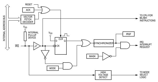
Figure 8-2. IRQ Module Block Diagram
