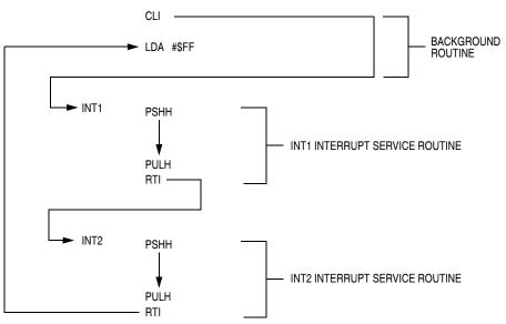
Figure 15-11. Interrupt Recognition Example
