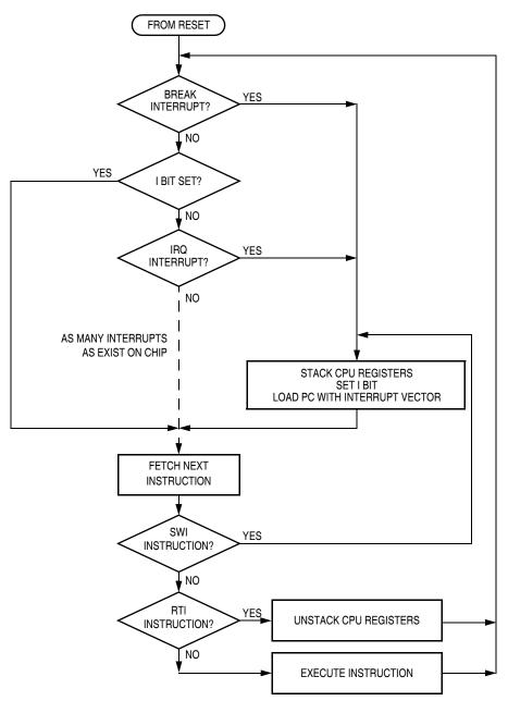
Figure 15-10. Interrupt Processing
