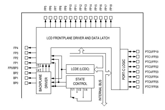
Figure 16-2. LCD Block Diagram
