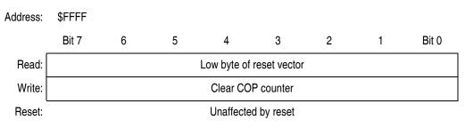
Figure 20-3. COP Control Register (COPCTL)
