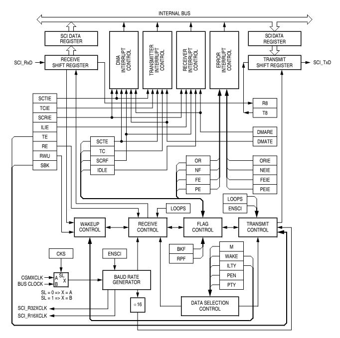
Figure 13-5. SCI Module Block Diagram
