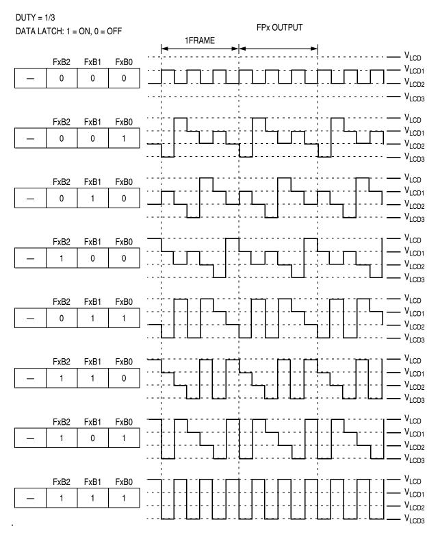
Figure 16-9. 1/3 Duty LCD Frontplane Driver Waveforms
