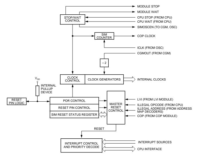
Figure 9-1. SIM Block Diagram
