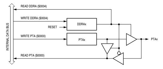
Figure 17-4. Port A I/O Circuit
