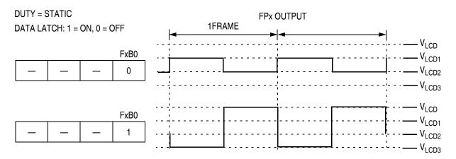
Figure 16-8. Static LCD Frontplane Driver Waveforms
