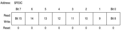
Figure 22-4. Break Address Register High (BRKH)
