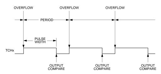
Figure 11-3. PWM Period and Pulse Width
