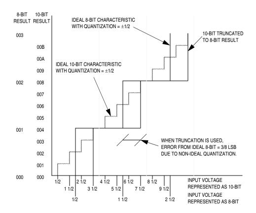
Figure 15-3. 8-Bit Truncation Mode Error
