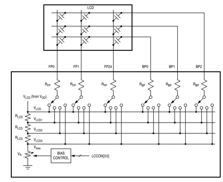
Figure 16-3. Simplified LCD Schematic (1/3 Duty, 1/3 Bias)
