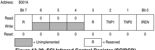
Figure 13-20. SCI Infrared Control Register (SCIRCR)
