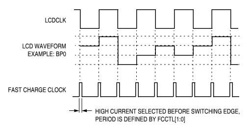
Figure 16-4. Fast Charge Timing
