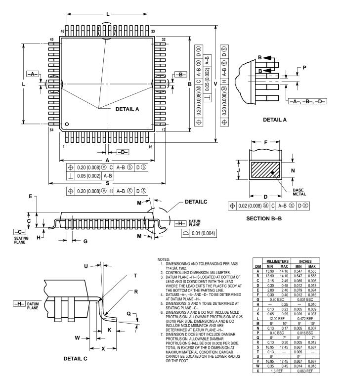
Figure 24-3. 64-Pin Quad Flat Pack (Case No. 840B)
