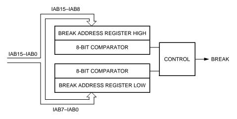
Figure 22-1. Break Module Block Diagram
