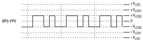
Figure 16-15. "e" Segment Voltage Waveform
