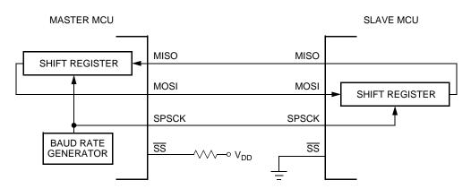
Figure 14-3. Full-Duplex Master-Slave Connections
