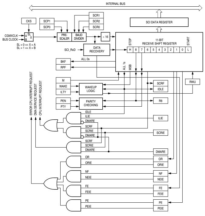
Figure 13-8. SCI Receiver Block Diagram
