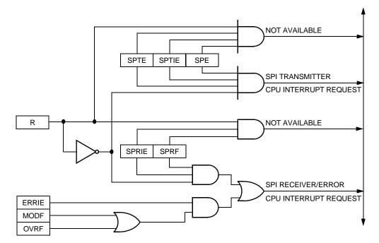
Figure 14-11. SPI Interrupt Request Generation
