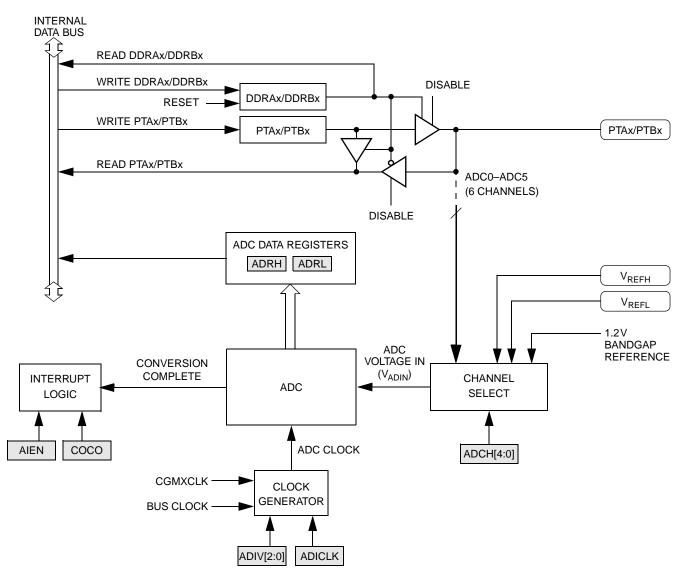
Figure 15-2. ADC Block Diagram
