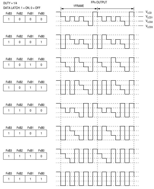
Figure 16-11. 1/4 Duty LCD Frontplane Driver Waveforms (continued)
