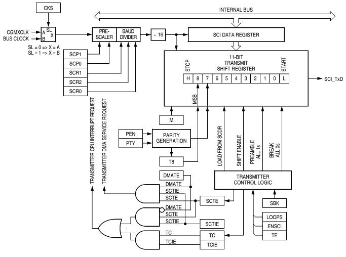
Figure 13-7. SCI Transmitter
