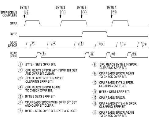
Figure 14-10. Clearing SPRF When OVRF Interrupt Is Not Enabled
