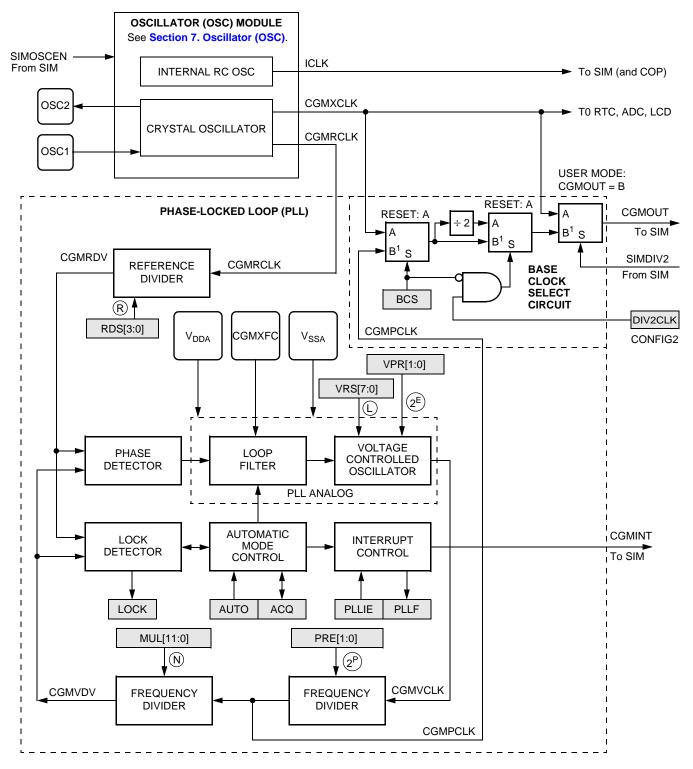
Figure 8-1. CGM Block Diagram
