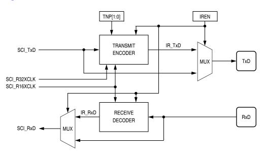
Figure 13-3 shows the structure of the infrared sub-module.
