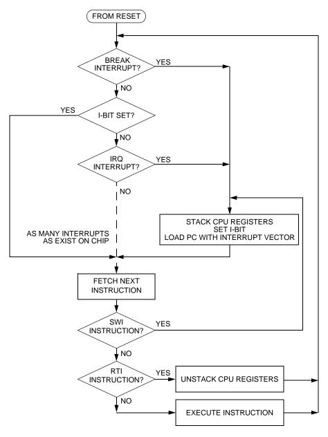
Figure 9-10. Interrupt Processing
