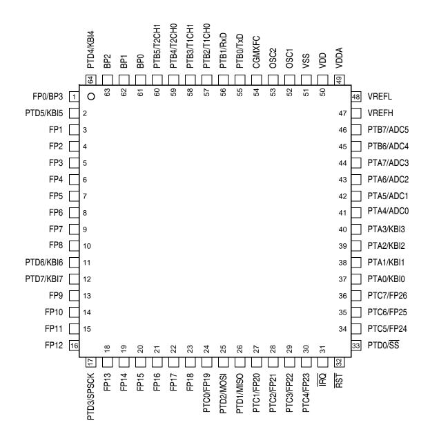
Figure 1-2. 64-Pin QFP and 64-Pin LQFP Pin Assignment
