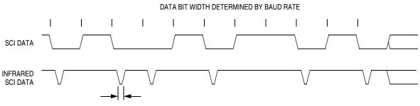
PULSE WIDTH = 1/32, 1/16, OR 3/16 DATA BIT WIDTH
