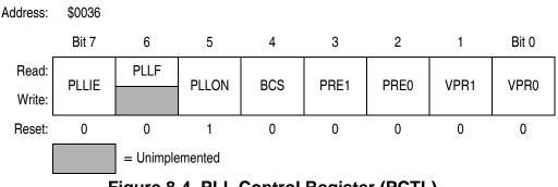
Figure 8-4. PLL Control Register (PCTL)
