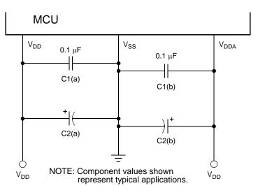
Figure 1-4. Power Supply Bypassing
