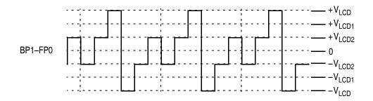
Figure 16-14. "f" Segment Voltage Waveform
