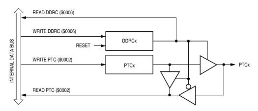
Figure 17-11. Port C I/O Circuit
