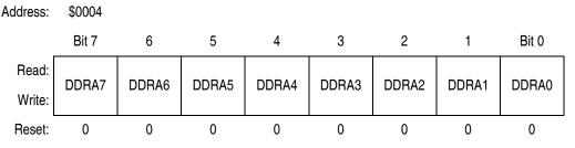
Figure 17-3. Data Direction Register A (DDRA)
