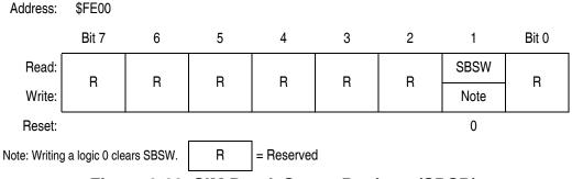
Figure 9-20. SIM Break Status Register (SBSR)
