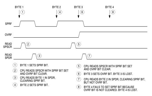
Figure 14-9. Missed Read of Overflow Condition
