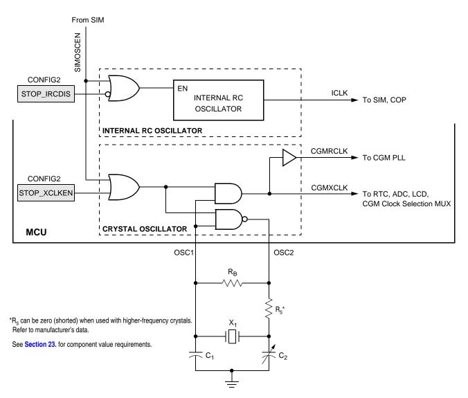
Figure 7-1. Oscillator Module Block Diagram
