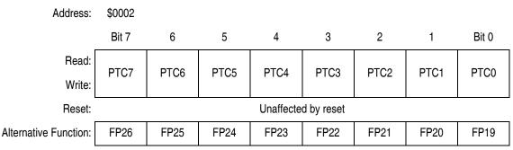
Figure 17-9. Port C Data Register (PTC)
