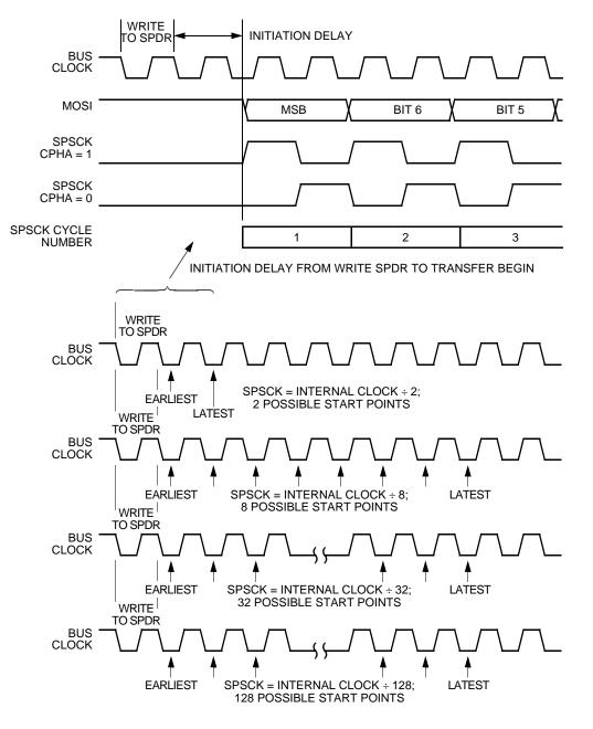
Figure 14-7. Transmission Start Delay (Master)
