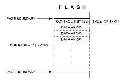
Figure 10-10. EE\_WRITE FLASH Memory Usage
