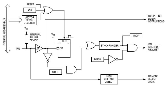
Figure 18-1. IRQ Module Block Diagram
