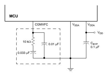
Note: Filter network in box can be replaced with a  $0.47\,\mu\text{F}$  capacitor, but will degrade stability.
