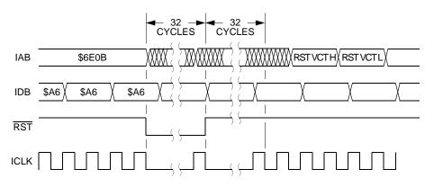
Figure 9-17. Wait Recovery from Internal Reset
