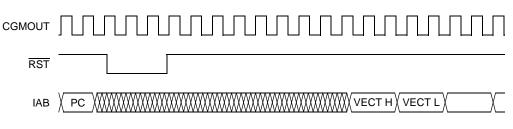
Figure 9-4. External Reset Timing
