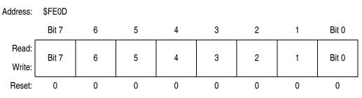
Figure 22-5. Break Address Register Low (BRKL)
