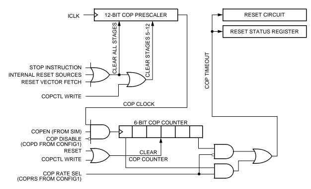
Figure 20-1. COP Block Diagram
