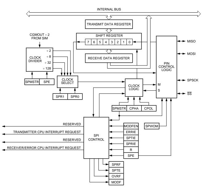
Figure 14-2. SPI Module Block Diagram
