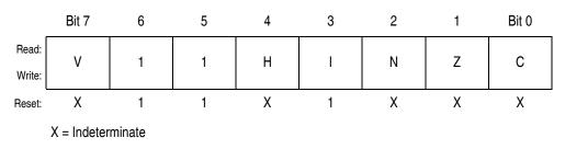
Figure 6-6. Condition Code Register (CCR)
