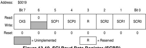
Figure 13-19. SCI Baud Rate Register (SCBR)
